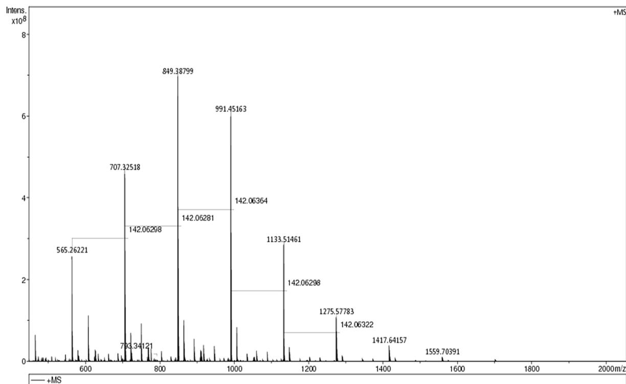
**Figure 2:** MALDI–TOF spectrum of poly(hexene carbonate) prepared using catalyst **2**. The peak at 565 Daltons corresponds to four ring-opened cyclohexene oxide units, three CO<sub>2</sub> units, 2 hydrogens (to cap the two terminal oxygens) and a sodium ion. The other peaks are then separated by 142 Daltons corresponding to an additional ring-opened cyclohexene oxide and carbon dioxide.
