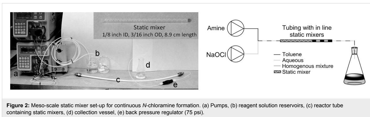
**Figure 2:** Meso-scale static mixer set-up for continuous *N*-chloramine formation. (a) Pumps, (b) reagent solution reservoirs, (c) reactor tube containing static mixers, (d) collection vessel, (e) back pressure regulator (75 psi).
