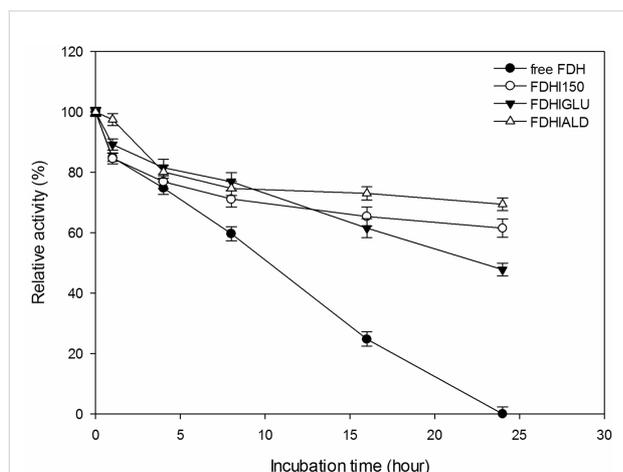
**Figure 4:** Thermal stability of free and immobilized FDH preparations at 35 °C.
