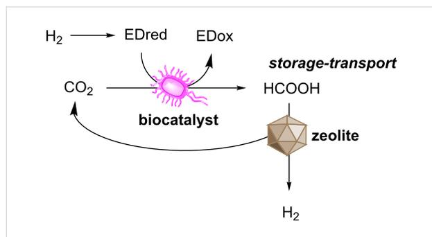
**Figure 6:** Hydrogen storage as formic acid through biocatalytic hydrogenation of CO<sub>2</sub> and subsequent on-demand release through zeolite catalysed dehydrogenation.
