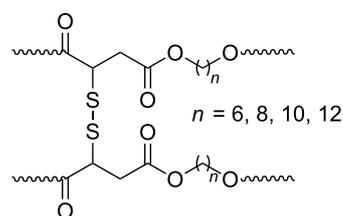
**Figure 12:** Oxidized poly(hexanediol-2-mercaptosuccinate) polymer.
