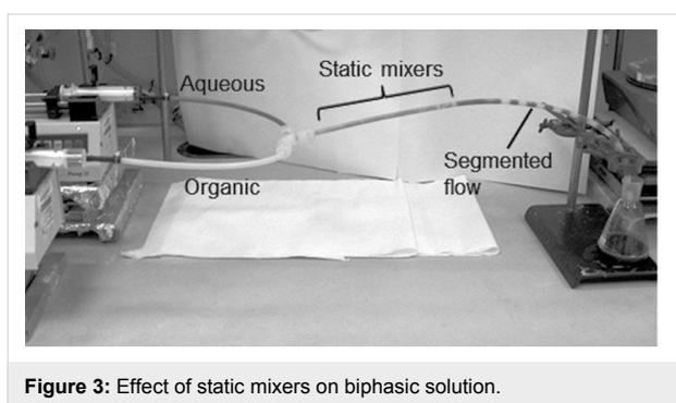
**Figure 3:** Effect of static mixers on biphasic solution.
