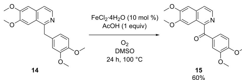
**Scheme 3:** Iron-catalyzed aerobic oxidation of papaverine (**14**).
