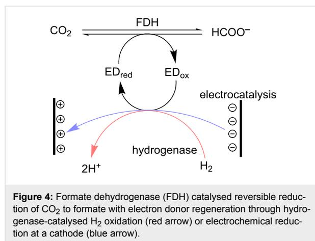
**Figure 4:** Formate dehydrogenase (FDH) catalysed reversible reduction of  $\text{CO}_2$  to formate with electron donor regeneration through hydrogenase-catalysed  $\text{H}_2$  oxidation (red arrow) or electrochemical reduction at a cathode (blue arrow).
