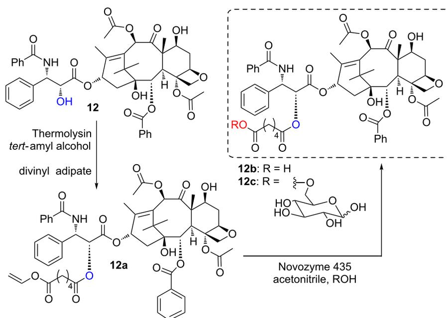
**Scheme 2:** Biocatalyzed synthesis of paclitaxel derivatives.
