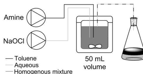
**Figure 5:** CSTR set-up for *N*-chloramine formation. (a) Syringe pump, (b) collection vessels, (c) reactor (50 mL), (d) stirrer plate: stirring rate 1200 rpm.
