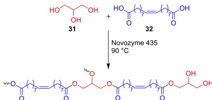
**Figure 10:** Biocatalyzed synthesis of polyesters containing glycerol.
