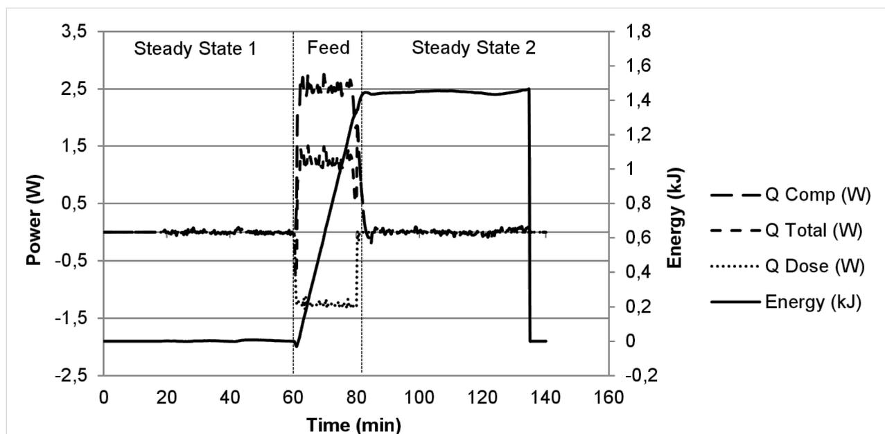
**Figure 1:** Calorimeter trace for the single phase reaction of morpholine (aq) and NaOCl (aq).  $Q$  Comp: compensatory power,  $Q$  Total: total power,  $Q$  Dose: power delivered by dosing of room temperature NaOCl (aq) to cooled reaction solution. Energy: heat energy.
