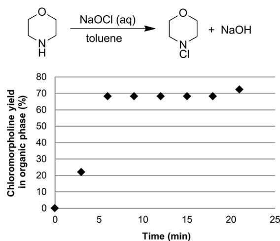
**Figure 4:** Progress of reaction for continuous formation of *N*-chloromorpholine. Morpholine (toluene) 0.9 M 1 mL/min, NaOCl (aq) 0.9 M, 1.1 mL/min, 6 mL total reactor volume, of which 0.8 mL is static mixers. Residence time = 2.9 min. Conversion refers to composition of organic phase of reaction solution.
