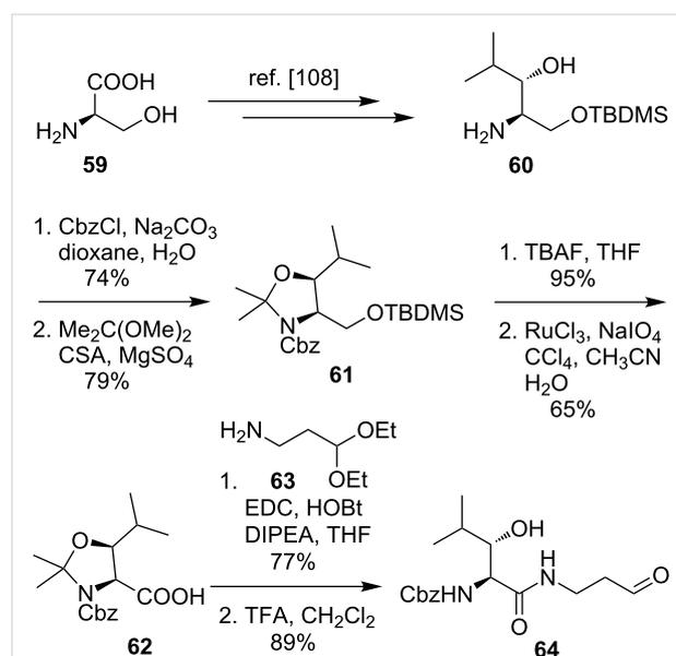
**Scheme 8:** Synthesis of a hydroxyleucine-derived aldehyde building block reported by Ducho et al. [107].
