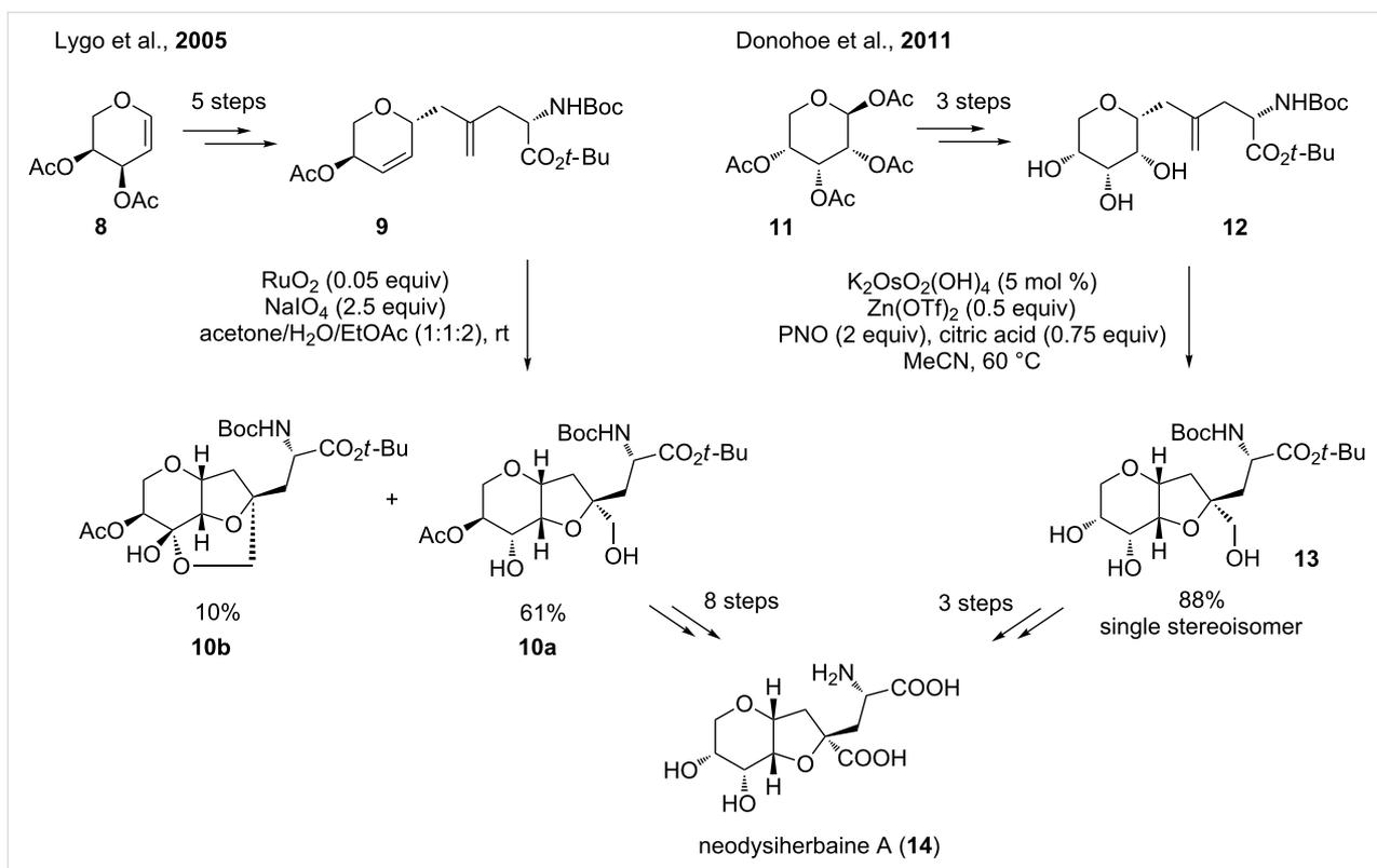
**Scheme 5:** Total synthesis of neodysiherbaine A via a Ru(VIII)- and an Os(VI)-catalyzed oxidative cyclization, respectively.
