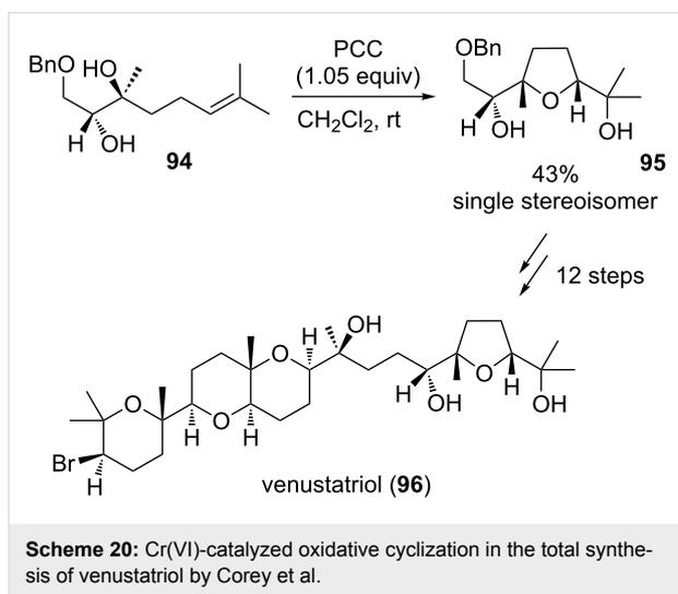
**Scheme 20:** Cr(VI)-catalyzed oxidative cyclization in the total synthesis of venustatriol by Corey et al.
