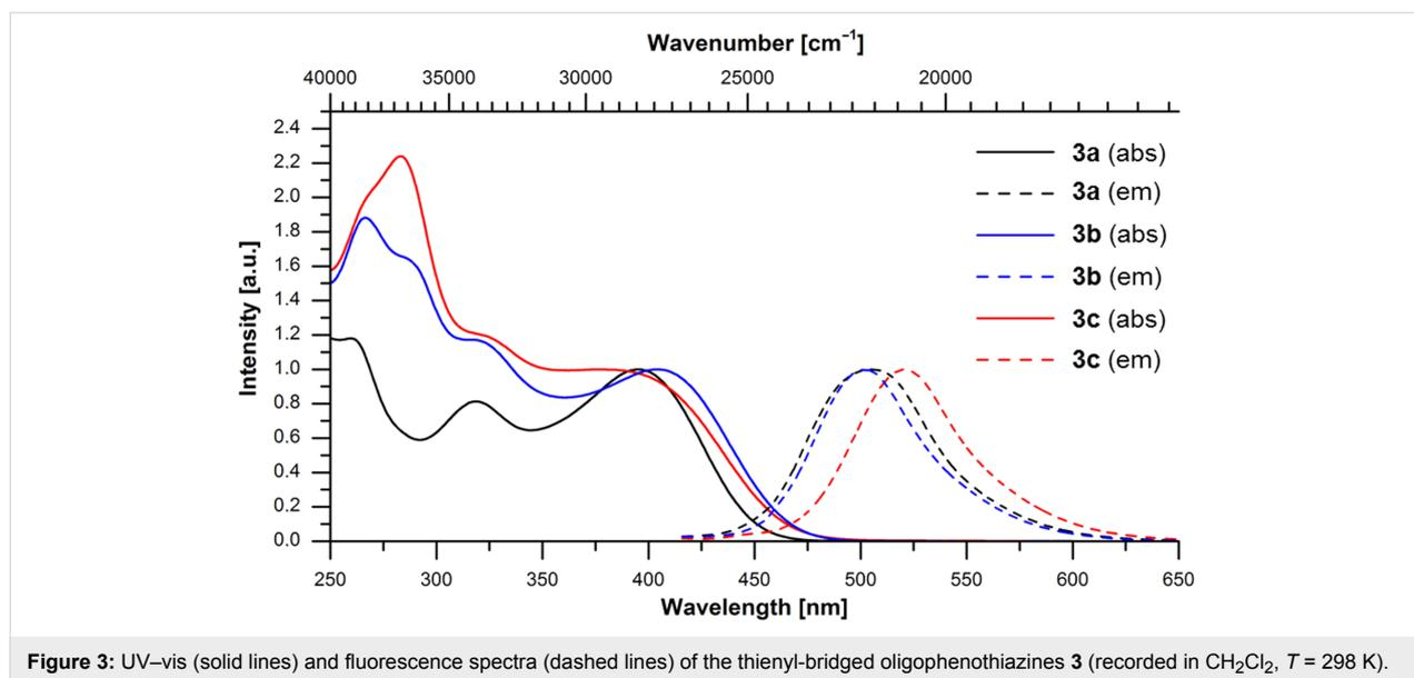
**Figure 3:** UV–vis (solid lines) and fluorescence spectra (dashed lines) of the thienyl-bridged oligophenothiazines **3** (recorded in CH<sub>2</sub>Cl<sub>2</sub>, *T* = 298 K).
