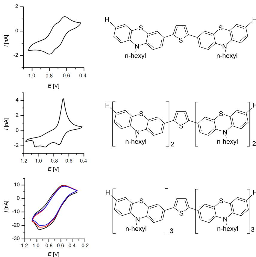
**Figure 2:** Cyclic voltammograms of compounds **3** (recorded in  $\text{CH}_2\text{Cl}_2$ ,  $T = 293 \text{ K}$ , electrolyte  $n\text{-Bu}_4\text{N}^+\text{PF}_6^-$ , Pt working electrode, Pt counter electrode, Ag/AgCl reference electrode,  $\nu = 50 \text{ mV/s}$  (**3a** and **3b**),  $\nu = 100 \text{ mV/s}$  (**3c**, multisweep experiment, 1. cycle (black), 2. cycle (red), 3. cycle (blue)).
