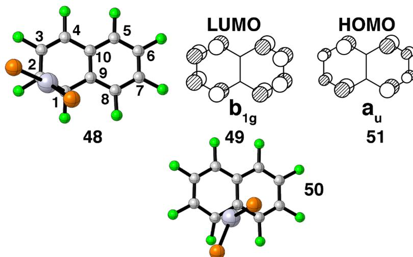
**Figure 14:** A top view of two stationary points found for  $F_8C_{10}$ -Pt(dpe); **48** is the ground state and **50**, represents one point on the plateau. The LUMO and HOMO in naphthalene are drawn in **49** and **51**, respectively.
