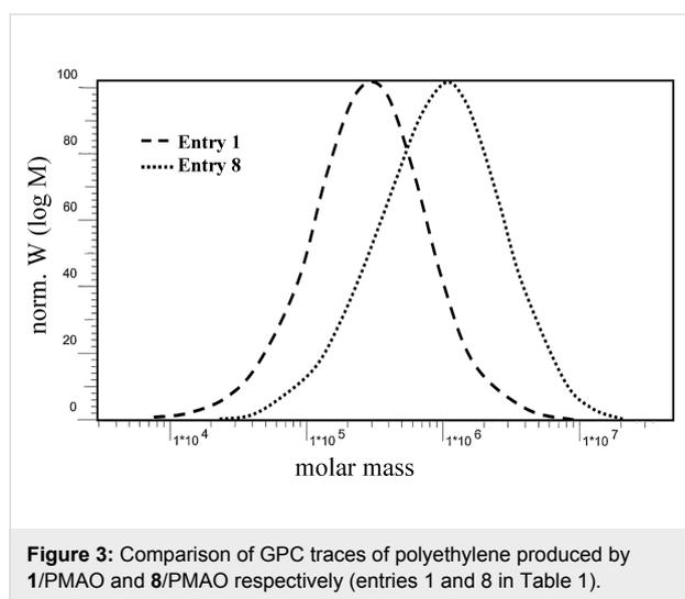
**Figure 3:** Comparison of GPC traces of polyethylene produced by 1/PMAO and 8/PMAO respectively (entries 1 and 8 in Table 1).
