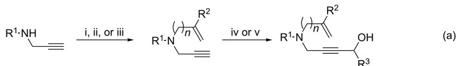
Conditions: i. NaH, DMSO, rt, then alkyl bromide, 14 h. ii) NaH, DMF, 0 °C, then alkyl bromide, 0 °C to rt, 17 h. iii) Alcohol, PPh<sub>3</sub>, DIAD, THF, rt, 17 h. iv) LiHMDS, THF, –78 °C, 30 min then R<sup>3</sup>CHO, –78 °C, 1 h. v) *n*-BuLi, THF, –78 °C, 30 min then R<sup>3</sup>CHO, –78 °C, 1 h.
