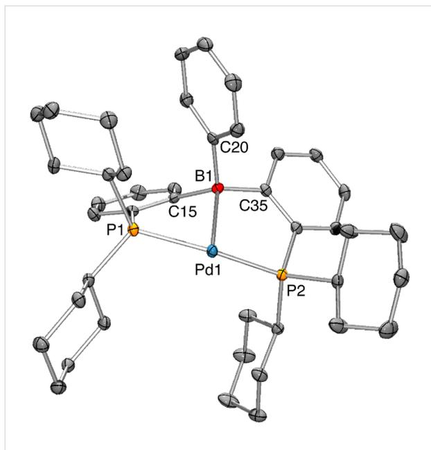
**Figure 2:** Thermal ellipsoid plots of complex **9** at the 50% probability level. H atoms and one molecule of hexane have been omitted for clarity. Selected interatomic distances (Å) and angles (°): Pd1–B1 2.243(2), Pd1–P1 2.2761(6), Pd1–P2 2.3084(6), B1–Pd1–P1 85.82(6), B1–Pd1–P2 82.49(6), P1–Pd1–P2 157.72(2), C15–B1–C20 110.94(18), C15–B1–C35 116.58(18), C20–B1–C35 112.56(18).
