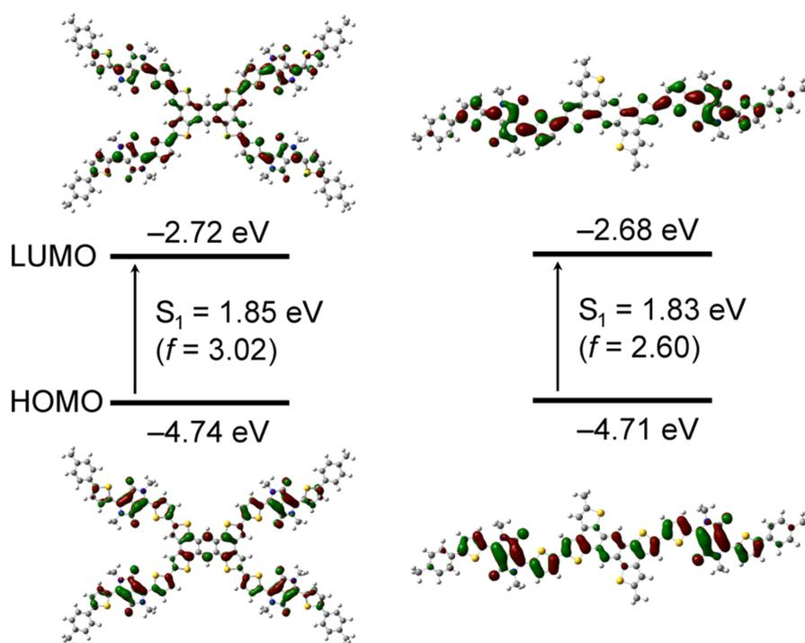
**Figure 2:** HOMO and LUMO distributions, calculated energy levels, and associated oscillator strengths ( $f$ ) for TTA-DPP4 and TTA-DPP2 calculated at the B3LYP/6-31G(d,p) level. The arrows indicate the first singlet–excited state ( $S_1$ ) transition. The alkyl chains are modified to methyl groups to simplify the calculations.
