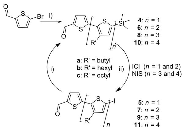
**Scheme 2:** Oligothiophenes **4–11** synthesised through reaction of the commercially available 5-bromo-2-thiophenecarboxaldehyde with **3a–c**, i) **3**, cat. Pd<sub>2</sub>dba<sub>3</sub>.4[f-Bu<sub>3</sub>PH]BF<sub>4</sub>, THF, K<sub>3</sub>PO<sub>4</sub> (2 M), 80 °C, 16 h, ii) ICl, DCM, 0 °C or NIS, 50:50 CHCl<sub>3</sub>/CH<sub>3</sub>CO<sub>2</sub>H, rt, 2 h.
