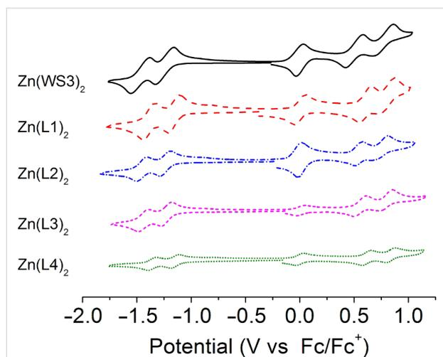
**Figure 6:** Cyclic voltammograms of zinc(II) chelates in 0.1 M TBAPF<sub>6</sub> dichloromethane solution with Fc/Fc<sup>+</sup> as an internal standard ( $E_{1/2}$  at 0.0 V).
