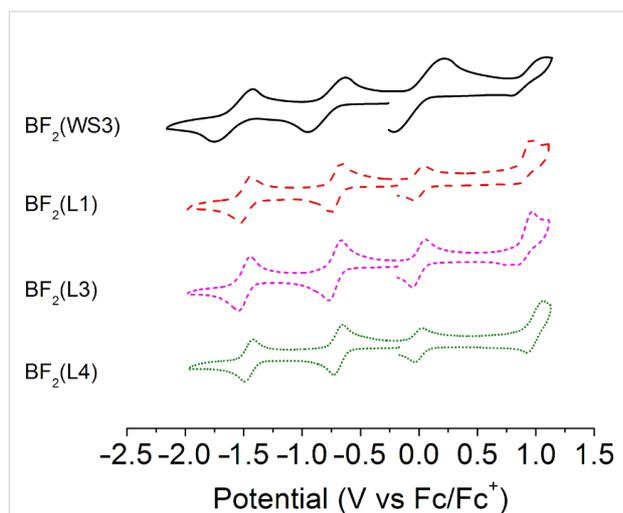
**Figure 7:** Cyclic voltammograms of BF<sub>2</sub><sup>+</sup> chelates in 0.1 M TBAPF<sub>6</sub> dichloromethane solution with Fc/Fc<sup>+</sup> as an internal standard ( $E_{1/2}$  at 0.0 V).
