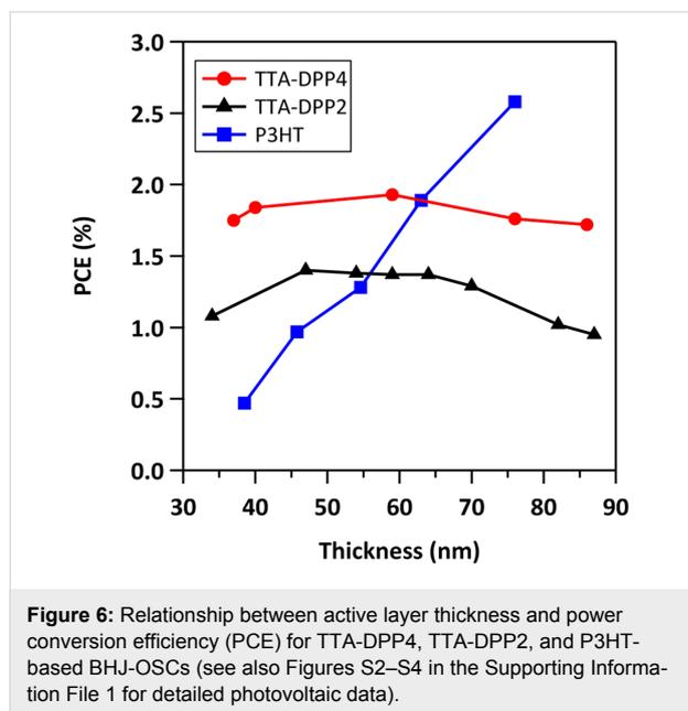
**Figure 6:** Relationship between active layer thickness and power conversion efficiency (PCE) for TTA-DPP4, TTA-DPP2, and P3HT-based BHJ-OSCs (see also Figures S2–S4 in the Supporting Information File 1 for detailed photovoltaic data).
