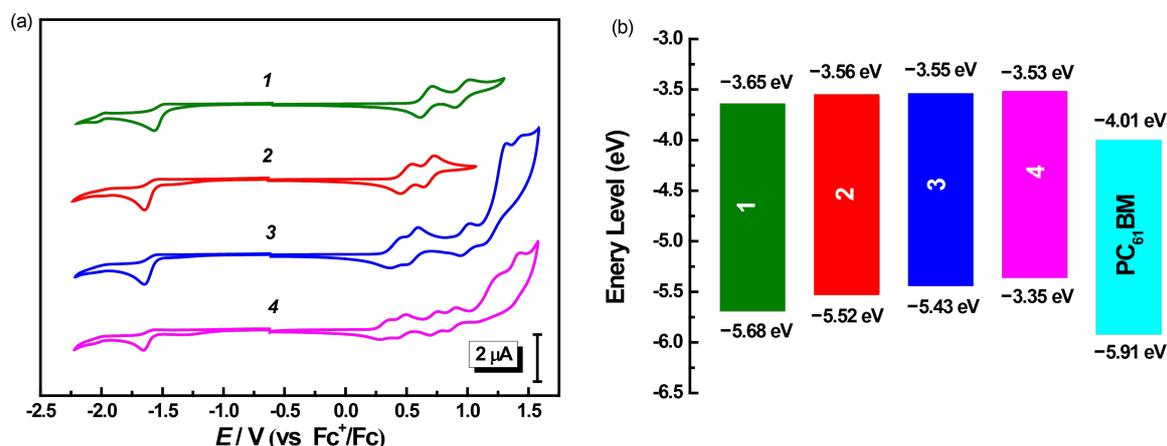
**Figure 2:** (a) Cyclic voltammograms of **1–4** measured in  $\text{CH}_2\text{Cl}_2$  solution ( $1.0 \times 10^{-3} \text{ mol} \cdot \text{L}^{-1}$ ) with  $0.1 \text{ mol} \cdot \text{L}^{-1} \text{ Bu}_4\text{NPF}_6$  at a scan rate of  $100 \text{ mV} \cdot \text{s}^{-1}$ ; (b) HOMO and LUMO energy levels of these compounds.
