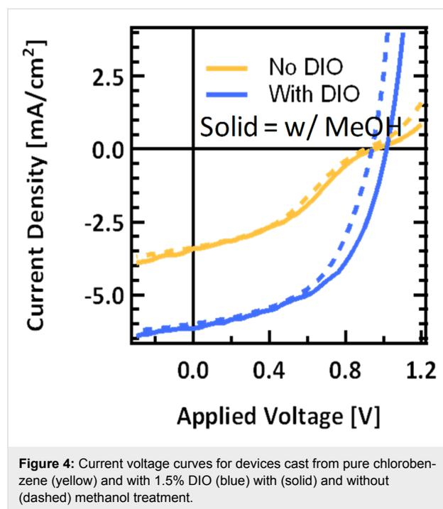
**Figure 4:** Current voltage curves for devices cast from pure chlorobenzene (yellow) and with 1.5% DIO (blue) with (solid) and without (dashed) methanol treatment.
