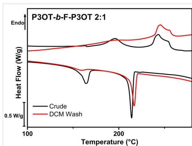
**Figure 1:** Differential scanning calorimetry thermogram (second cycle, 10 K/min) of P3OT-*b*-F-P3OT 2:1 before (black) and after (red) washing with dichloromethane. The reduction in the thermal transitions occurring below 200 °C, attributed to P3OT, indicate that a substantial amount of P3OT homopolymer was present in the crude polymer, but was removed by extraction.
