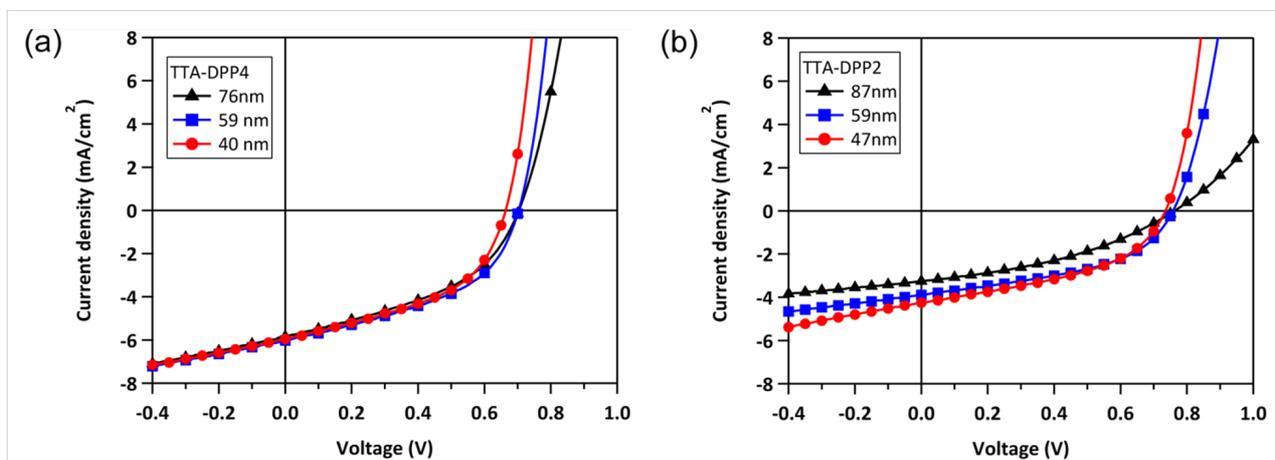
**Figure 5:**  $J$ – $V$  characteristics of BHJ-OSCs based on (a) TTA-DPP4:PC<sub>71</sub>BM (1:1.5, w/w) and (b) TTA-DPP2:PC<sub>71</sub>BM (1:1.5, w/w) with different active layer thicknesses, measured under simulated AM 1.5G,  $100 \text{ mW cm}^{-2}$  illumination.
