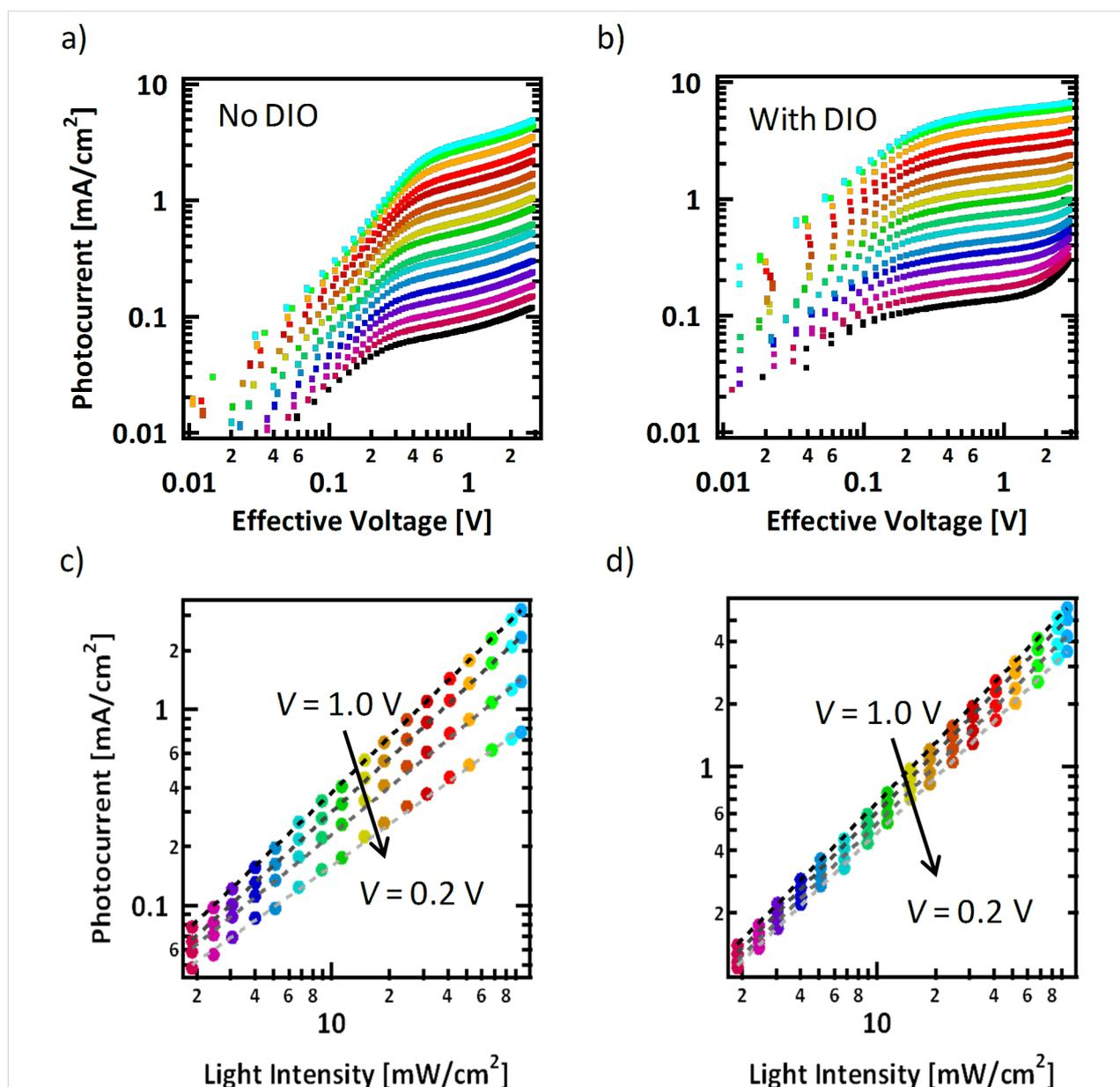
**Figure 3:** Light intensity dependence of photocurrent as a function of the effective voltage,  $V_0 - V$ , for devices cast a) without DIO and b) with DIO and the extracted photocurrent at effective voltages of 1.0, 0.5, 0.3, and 0.2 V (from black to grey, respectively) as detailed in Table 2 for devices cast c) without DIO and d) with DIO.
