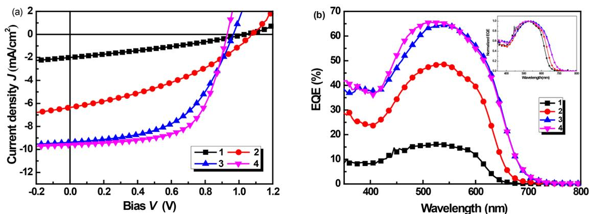
**Figure 3:** (a)  $J$ - $V$  curves of the best COOP-*n*HT-TBTD:PC<sub>61</sub>BM solar cells; (b) EQE spectra of the corresponding cells, Inset: normalized EQE spectra of four best devices, showing the difference in spectrum response wavelength range.
