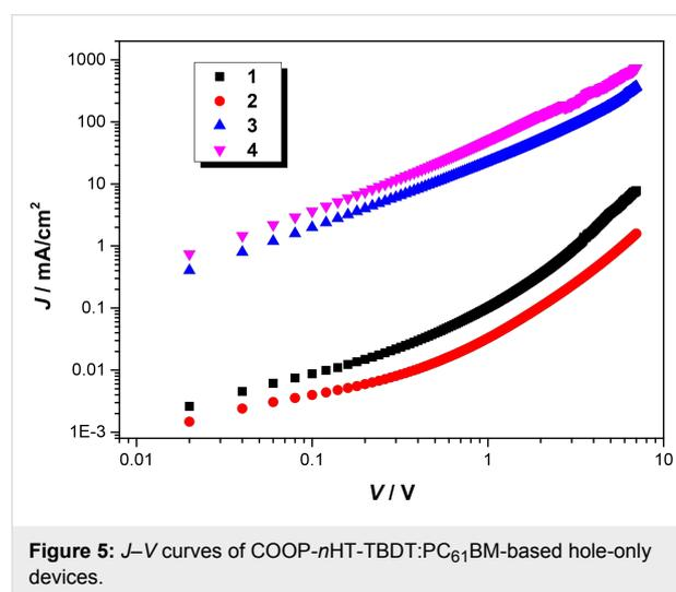
**Figure 5:** *J*-*V* curves of COOP-*n*HT-TBDT:PC<sub>61</sub>BM-based hole-only devices.
