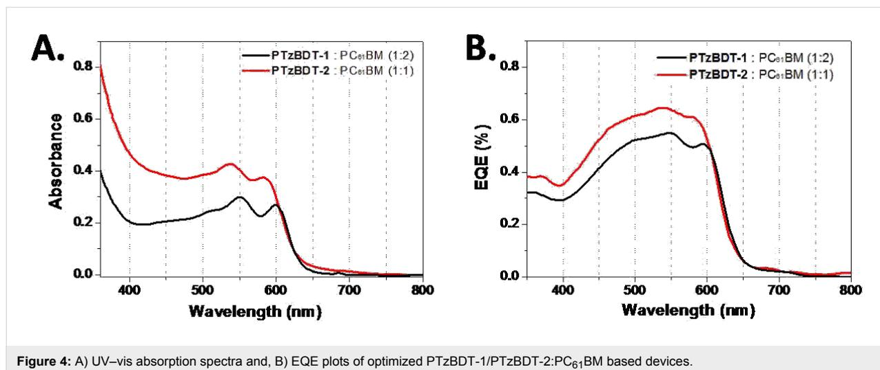
Figure 4: A) UV-vis absorption spectra and, B) EQE plots of optimized PTzBDT-1/PTzBDT-2:PC<sub>61</sub>BM based devices.
