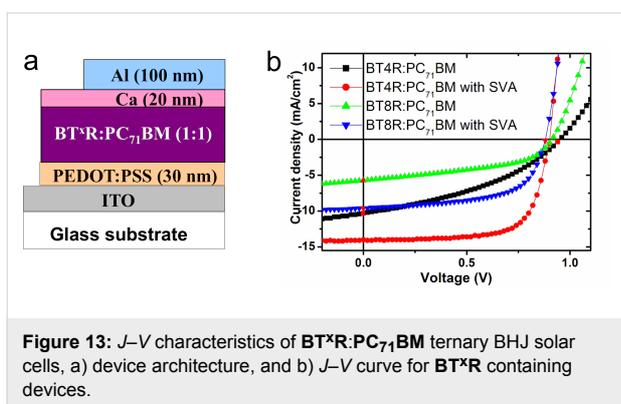
**Figure 13:**  $J$ - $V$  characteristics of **BT<sup>x</sup>R:PC<sub>71</sub>BM** ternary BHJ solar cells, a) device architecture, and b)  $J$ - $V$  curve for **BT<sup>x</sup>R** containing devices.
