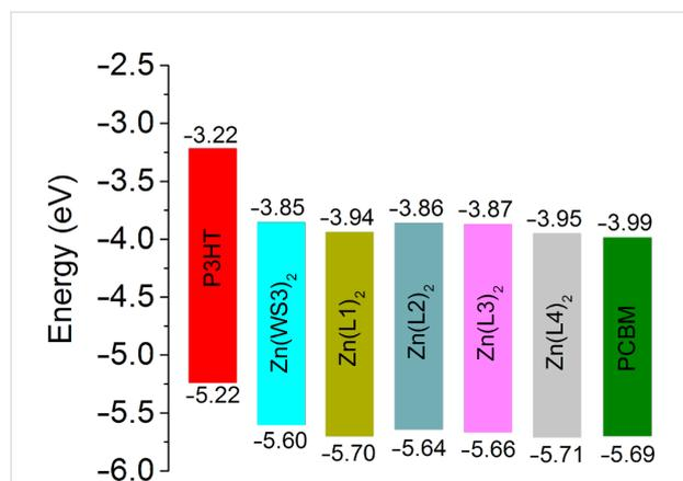
**Figure 8:** Estimated HOMO and LUMO energy levels obtained by cyclic voltammetry from the  $E_{1/2}$  values in dichloromethane solution, using the value of -5.1 eV for Fc/Fc<sup>+</sup>. The included HOMO and LUMO levels of P3HT films were estimated in our laboratory from the oxidation onset and the optical gap.
