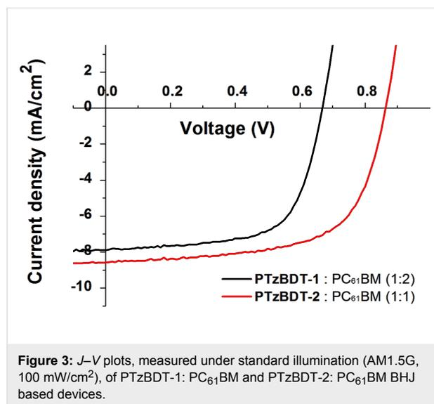
**Figure 3:**  $J$ – $V$  plots, measured under standard illumination (AM1.5G, 100 mW/cm<sup>2</sup>), of PTzBDT-1:PC<sub>61</sub>BM and PTzBDT-2:PC<sub>61</sub>BM BHJ based devices.
