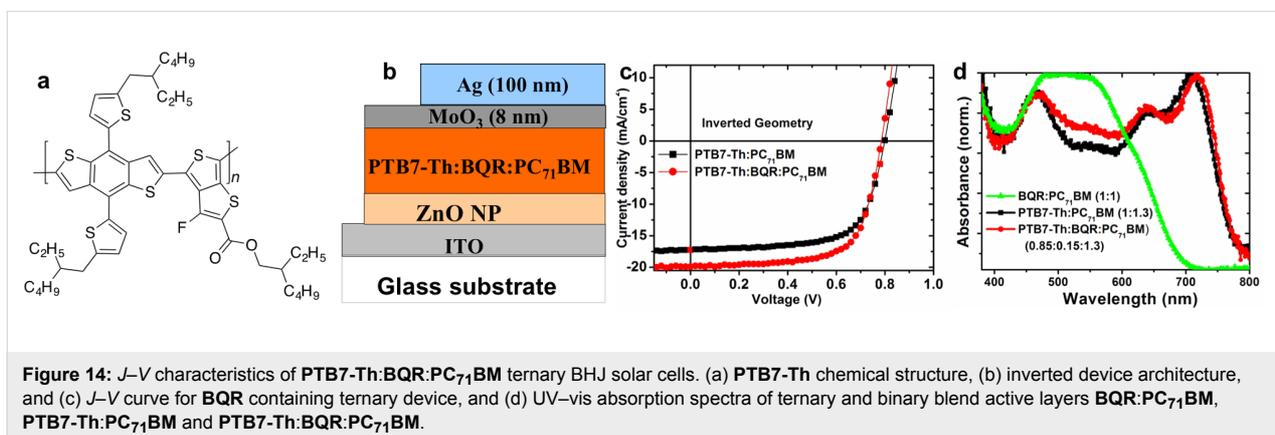
**Figure 14:**  $J$ - $V$  characteristics of **PTB7-Th:BQR:PC<sub>71</sub>BM** ternary BHJ solar cells. (a) **PTB7-Th** chemical structure, (b) inverted device architecture, and (c)  $J$ - $V$  curve for **BQR** containing ternary device, and (d) UV-vis absorption spectra of ternary and binary blend active layers **BQR:PC<sub>71</sub>BM**, **PTB7-Th:PC<sub>71</sub>BM** and **PTB7-Th:BQR:PC<sub>71</sub>BM**.
