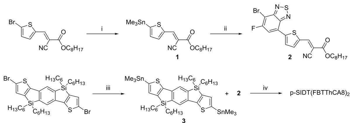
**Scheme 1:** Synthetic route towards p-SIDT(FBTThCA8)<sub>2</sub>. (i) Sn<sub>2</sub>Me<sub>6</sub>, Pd(PPh<sub>3</sub>)<sub>4</sub>, toluene, 85 °C; (ii) 4,7-dibromo-5-fluorobenzo[c][1,2,5]thiadiazole, Pd(PPh<sub>3</sub>)<sub>4</sub>, toluene, 90 °C, 42.8%; (iii) *n*-BuLi, THF, –78 °C, 10 min; then Me<sub>3</sub>SnCl, 98.9%; (iv) Pd(PPh<sub>3</sub>)<sub>4</sub>, toluene, MW, 80.6%.
