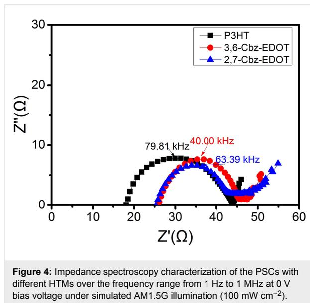
**Figure 4:** Impedance spectroscopy characterization of the PSCs with different HTMs over the frequency range from 1 Hz to 1 MHz at 0 V bias voltage under simulated AM1.5G illumination ( $100 \text{ mW cm}^{-2}$ ).
