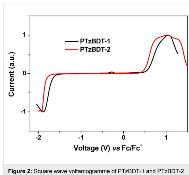
**Figure 2:** Square wave voltammogramme of PTzBDT-1 and PTzBDT-2.
