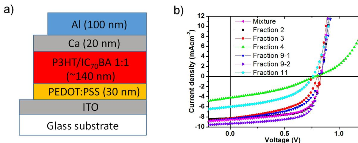
**Figure 7:** Schematic diagram of the architecture of BHJ solar cell devices (a) and  $J$ - $V$  curves of the devices containing P3HT and each IC<sub>70</sub>BA fractions (b).**Table 2:** Performance of BHJ solar cell devices based on a blend of P3HT and each IC<sub>70</sub>BA fractions as the active layer.<sup>a</sup>
