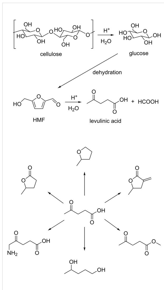
**Scheme 1:** Synthesis of levulinic acid from ligno-cellulosic feedstocks and its principal uses to access fine chemicals.
