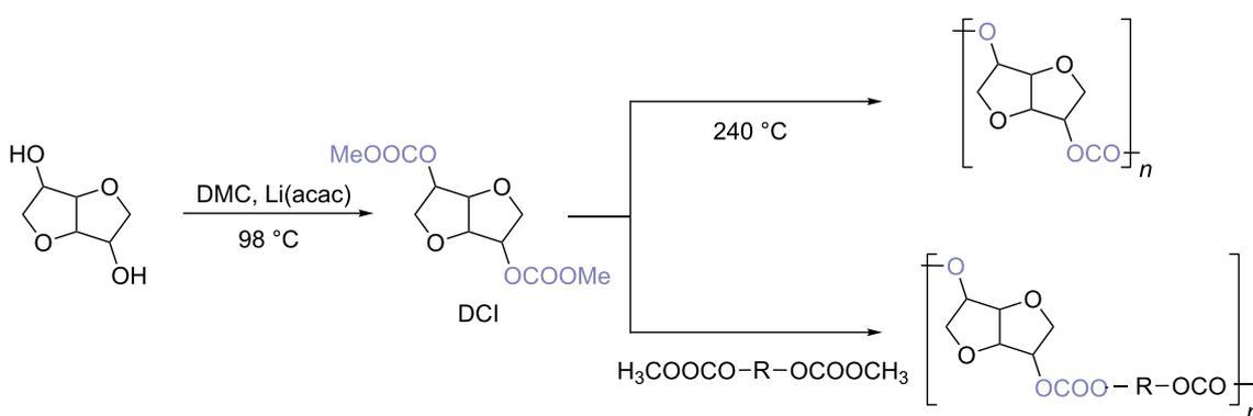
**Scheme 4:** Isosorbide homo- and co-polycarbonate via melt polycondensation.
