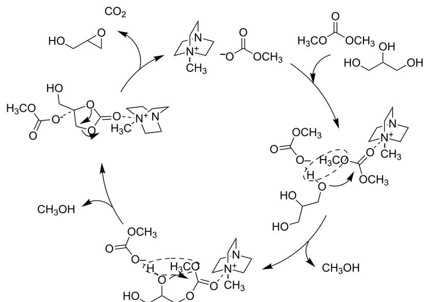
**Scheme 14:** Cooperative mechanism of ionic liquid-catalyzed glycidol production.
