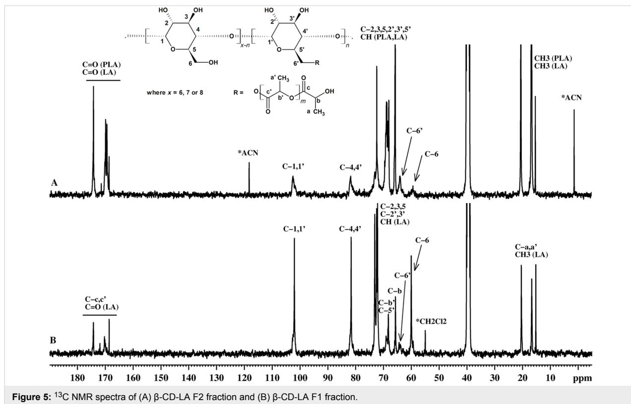
Figure 5:  $^{13}\text{C}$  NMR spectra of (A)  $\beta$ -CD-LA F2 fraction and (B)  $\beta$ -CD-LA F1 fraction.
