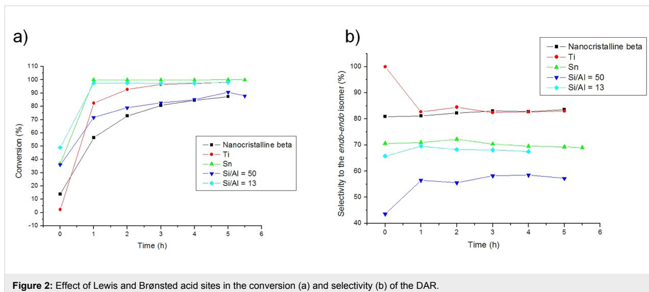
**Figure 2:** Effect of Lewis and Brønsted acid sites in the conversion (a) and selectivity (b) of the DAR.
