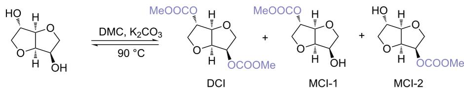
**Scheme 3:** Methoxycarbonylation of isosorbide via DMC chemistry.
