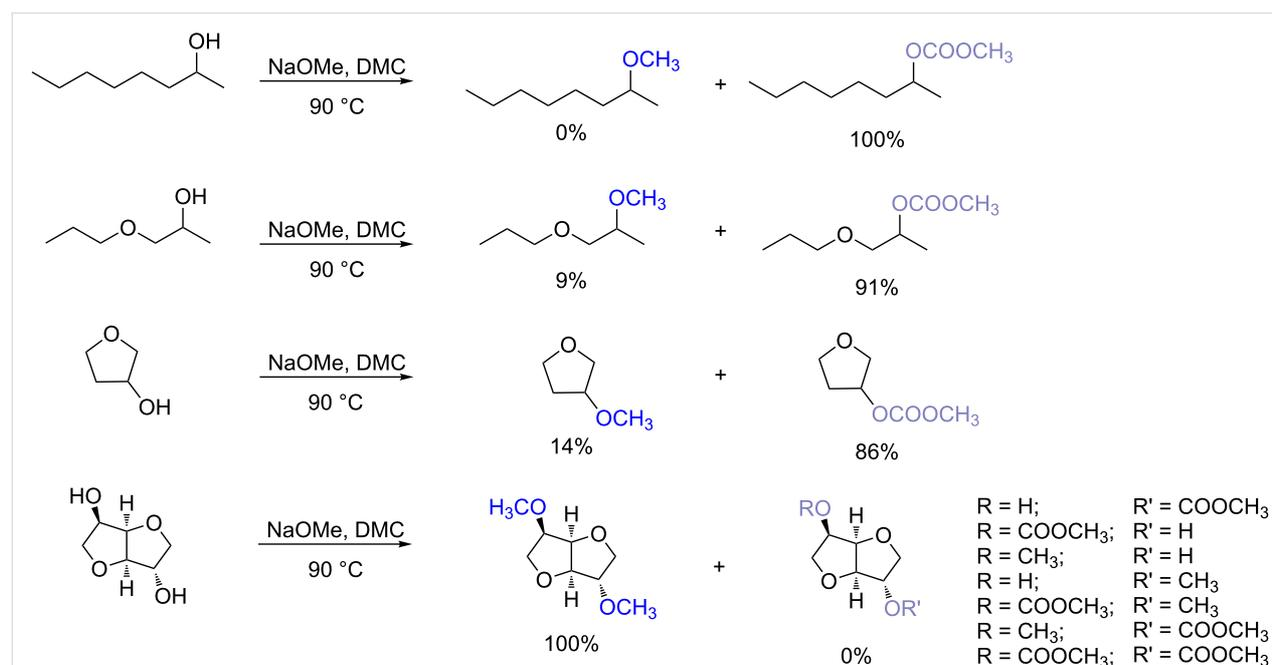
**Scheme 6:** Comparison of the reactivity of isororbide with other secondary alcohols in methylation reaction. Reaction conditions: Isororbide DMC 1:50 equiv; reaction time 20 h; 90 °C.
