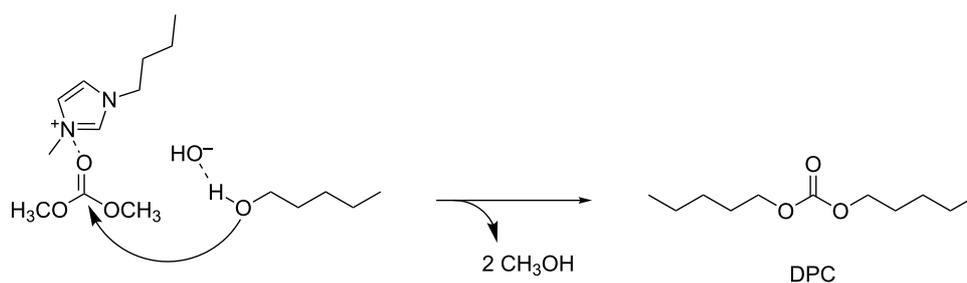
**Scheme 16:** [BMIM]OH-catalyzed synthesis of DPC from DMC and 1-pentanol.
