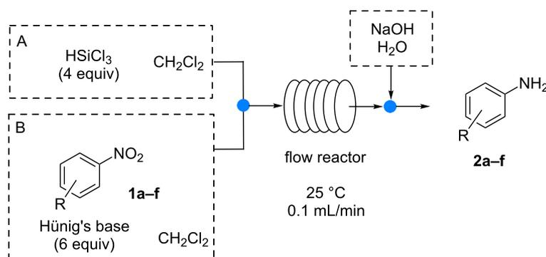
**Scheme 2:** Continuous flow reduction of aromatic nitro compounds.**Table 2:** Scope of the reaction (see Scheme 2).
