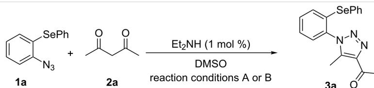
Scheme 2: Comparative study of the conventional conditions and ultrasound irradiation. Conditions A: Reaction at 25 °C for 2 h (**3a**, 98%); Conditions B: Reaction under ultrasound irradiation (20% of the amplitude) at 25 °C for 20 min (**3a**, 92%).
