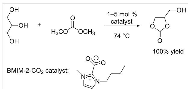
**Scheme 9:** Transesterification of glycerol with DMC in the presence of 1-*n*-butyl-3-methylimidazolium-2-carboxylate (BMIM-2-CO<sub>2</sub>).
