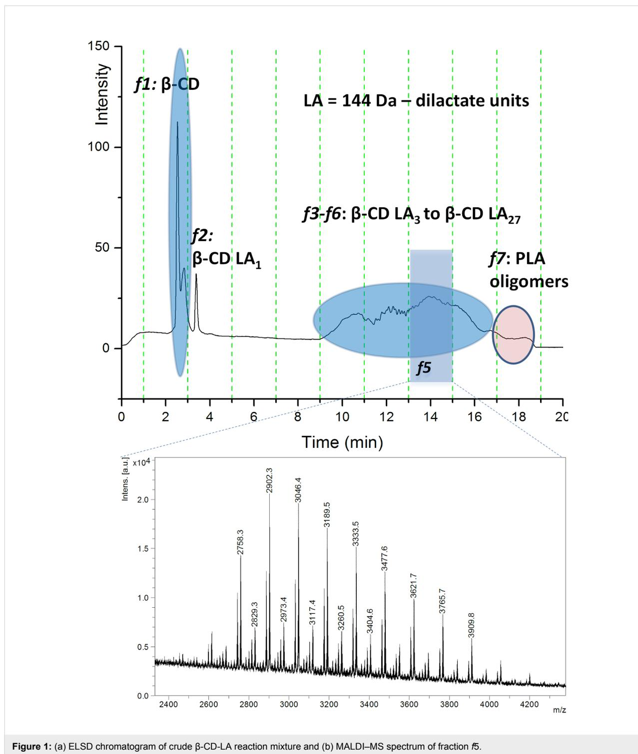
**Figure 1:** (a) ELSD chromatogram of crude  $\beta$ -CD-LA reaction mixture and (b) MALDI-MS spectrum of fraction *f5*.
