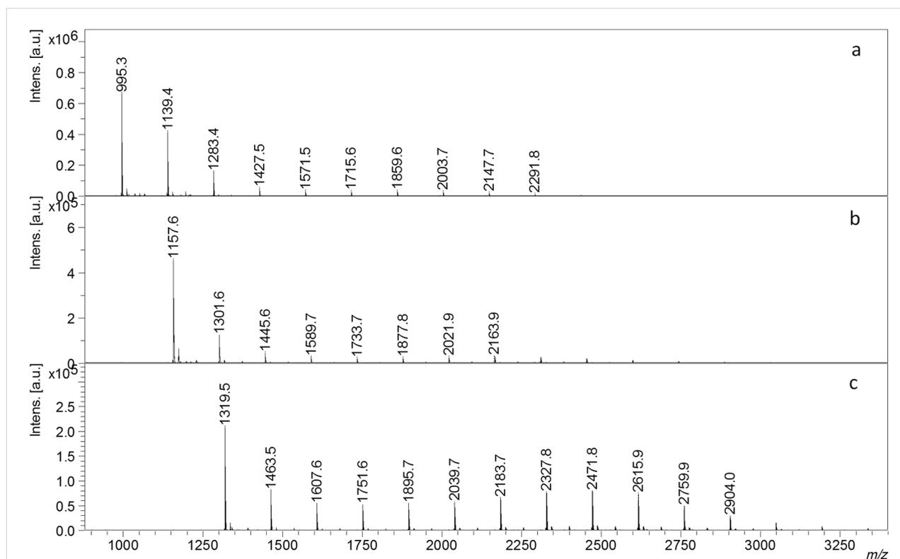
**Figure 2:** MALDI-MS spectra of the fractionated  $\alpha$ -,  $\beta$ - and  $\gamma$ -CD-LA products – fractions precipitated in THF: (a)  $\alpha$ -CD-LA fraction F1A, (b)  $\beta$ -CD-LA fraction F1B and (c)  $\gamma$ -CD-LA fraction F1C.
