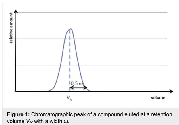
**Figure 1:** Chromatographic peak of a compound eluted at a retention volume  $V_R$  with a width  $\omega$ .
