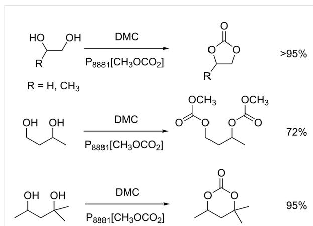
**Scheme 19:** Examples of carbonates obtained from different bio-based diols using  $[P_{8881}][CH_3OCO_2]$  as catalyst.
