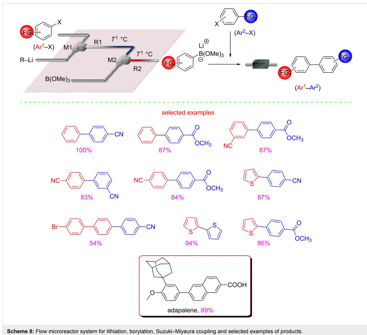
**Scheme 8:** Flow microreactor system for lithiation, borylation, Suzuki–Miyaura coupling and selected examples of products.
