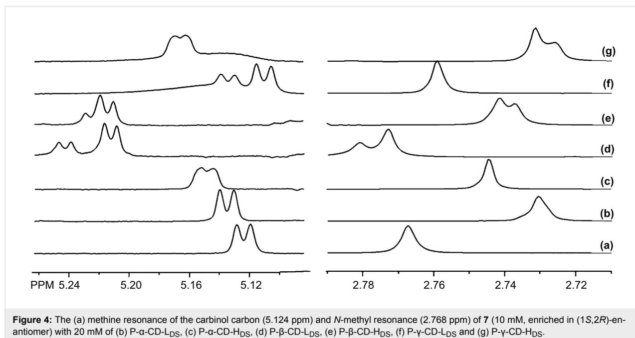
**Figure 4:** The (a) methine resonance of the carbinol carbon (5.124 ppm) and *N*-methyl resonance (2.768 ppm) of **7** (10 mM, enriched in (1*S*,2*R*)-enantiomer) with 20 mM of (b) P- $\alpha$ -CD-L<sub>DS</sub>, (c) P- $\alpha$ -CD-H<sub>DS</sub>, (d) P- $\beta$ -CD-L<sub>DS</sub>, (e) P- $\beta$ -CD-H<sub>DS</sub>, (f) P- $\gamma$ -CD-L<sub>DS</sub> and (g) P- $\gamma$ -CD-H<sub>DS</sub>.
