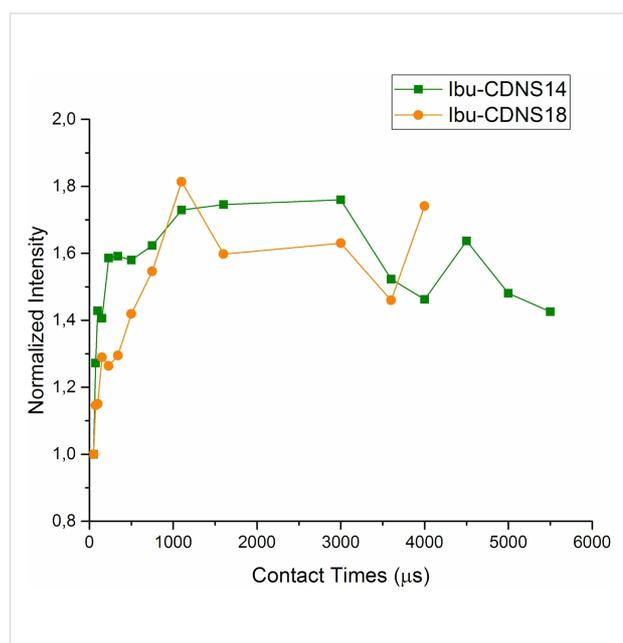
**Figure 9:**  $^1\text{H}$ - $^{13}\text{C}$  CP oscillatory kinetics for the ibuprofen aromatic carbon atoms C(6,8) in samples CDNS(1:4)-IbuNa and CDNS(1:8)-IbuNa. The notation CDNS-IbuNa indicates the original preparation, irrespective of the conversion of the sodium salt into the undissociated acid.
