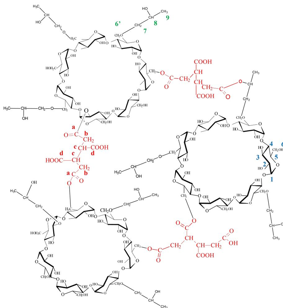
**Figure 1:** Chemical structure of the non-activated polyBTCA-CD.
