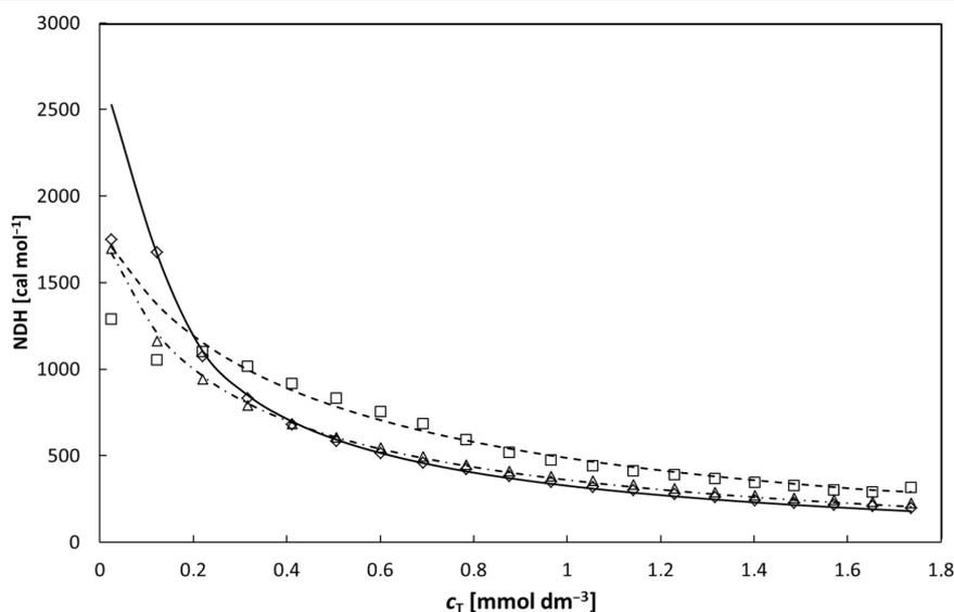
**Figure 7:** Heat change for injection per mole of NA- $\gamma$ -CD added as a function of the total concentration of NA- $\gamma$ -CD at 10 °C. Symbols are used for experimental values; lines for fits: 6-*O*-NA- $\gamma$ -CD **2c** squares and a dashed line; 2-*O*-NA- $\gamma$ -CD **2a** diamonds and a full line; 3-*O*-NA- $\gamma$ -CD **2b** triangles and a dashed-dotted line.
