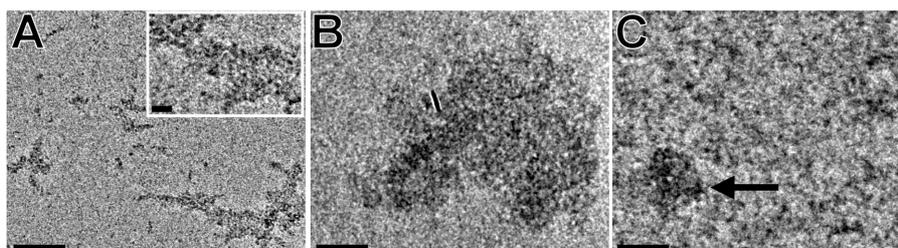
**Figure 5:** Effect of increasing concentration and sonication on the morphology of the 2-*O*-derivative **2a**. A: 2 mM unsonicated specimen; B: 20 mM unsonicated specimen; C: 100 mM sonicated specimen. The arrow indicates an aggregated particle. Scale bars: 50 nm, inset: 10 nm.
