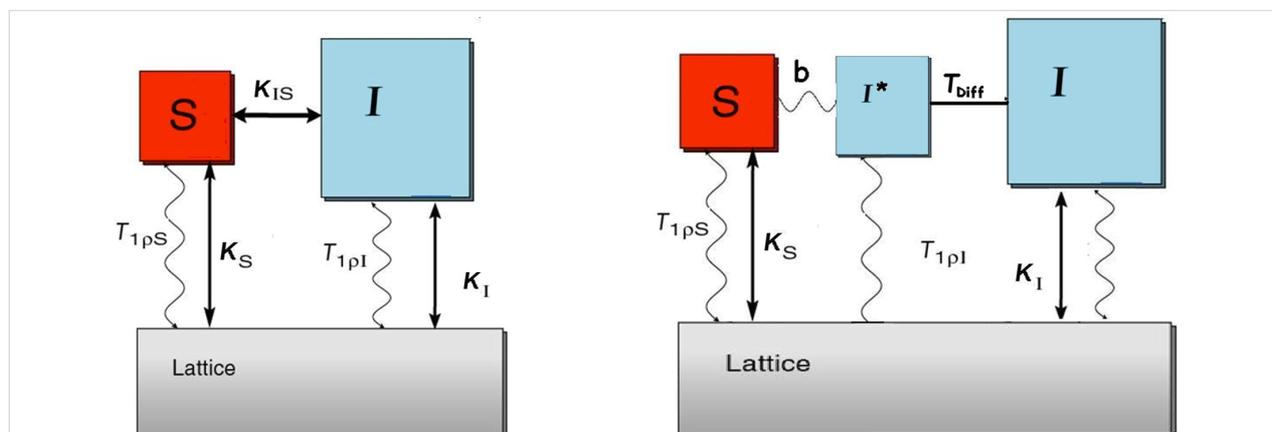
**Figure 1:** Schematic thermodynamic description of the CP process and time constants. The  $I$ - $S$  model (left), the  $I$ - $I^*$ - $S$  model (right). Adapted with permission from [14]. Copyright 2002 American Chemical Society.
