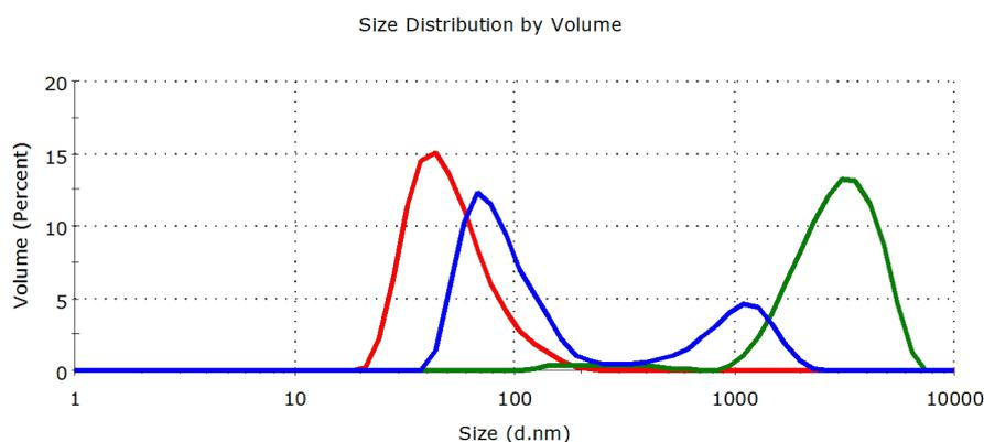
**Figure 3:** Aggregation effect of 0.1% NaCl on 0.02% nanoTiO<sub>2</sub> dispersion in the absence (green curve) and presence of CMBCD-P polymer (blue curve). The red curve shows the particle size distribution in the absence of destabilizing ions.
