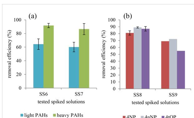
**Figure 7:** Removal efficiency (%) after treatment with activated polyBTCA-CD (concentration = 2 g·L<sup>-1</sup>) for (a) two concentrations of PAHs: low for SS6 and high for SS7 (*n* = 3) and (b) two concentrations of APs: low for SS8 (*n* = 3) and high for SS9 (*n* = 1) (4NP: 4-nonylphenol, 4nNP: 4-*n*-nonylphenol, 4tOP: 4-*tert*-octylphenol).
