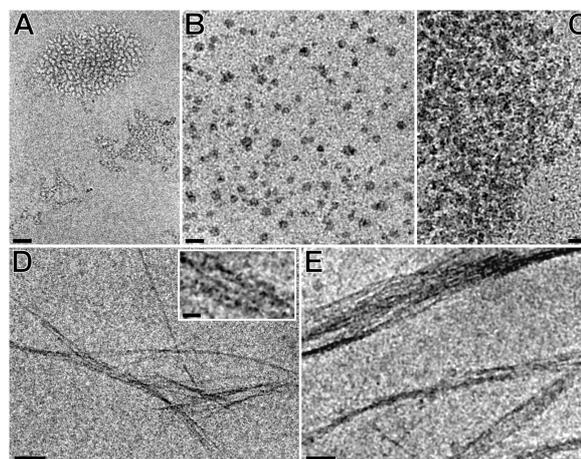
**Figure 4:** Effect of increasing concentration and sonication on the morphology of the 3-*O*-derivative **2b**. A to C: 2 mM, 20 mM, and 100 mM unsonicated specimens; D: fibers of the 2 mM specimen after sonication. Inset: high-magnification detail of the fibers; E: fibers and aggregates of the 100 mM specimen. Scale bars: A–C: 50 nm, D–E: 100 nm, inset: 20 nm.
