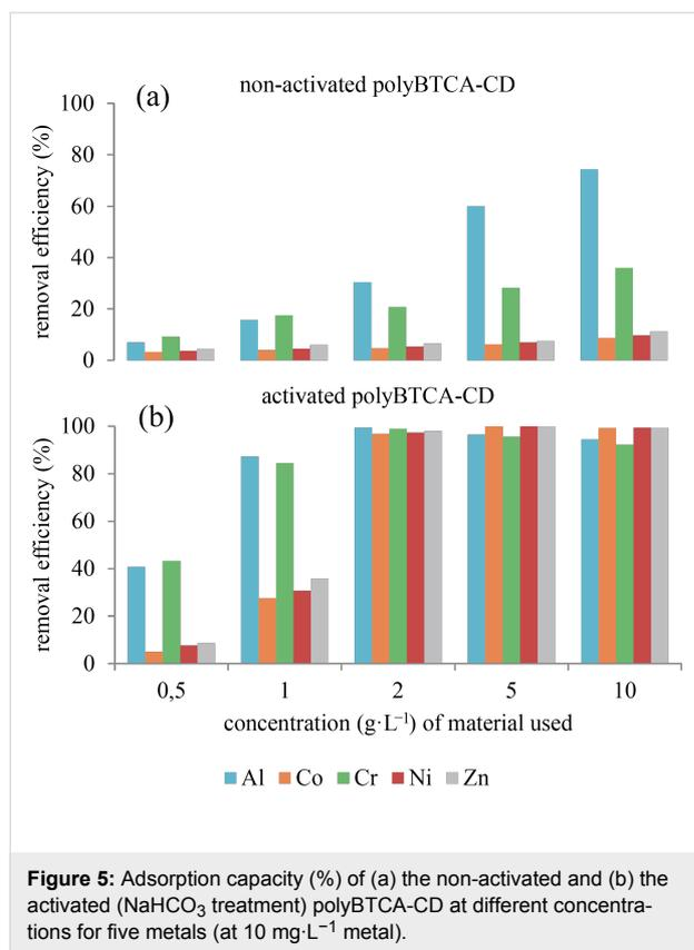
**Figure 5:** Adsorption capacity (%) of (a) the non-activated and (b) the activated (NaHCO<sub>3</sub> treatment) polyBTCA-CD at different concentrations for five metals (at 10 mg·L<sup>-1</sup> metal).
