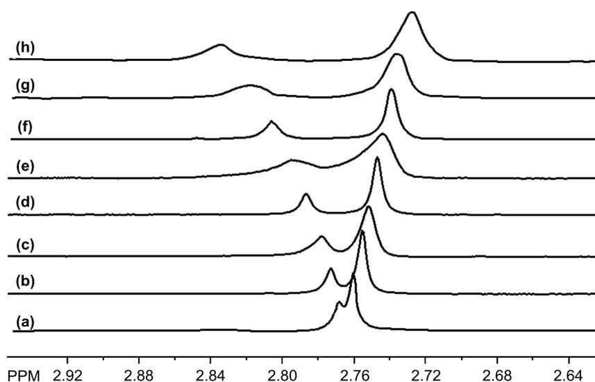
**Figure 5:** The *N*-methyl resonance of **7** (10 mM, enriched in (1*S*,2*R*)-enantiomer) with P- $\beta$ -CD-L<sub>DS</sub> (20 mM) and concentrations of ytterbium(III) nitrate of (a) 0 mM, (b) 2 mM, (c) 4 mM, (d) 6 mM, (e) 8 mM, (f) 10 mM, (g) 12 mM and (h) 16 mM.
