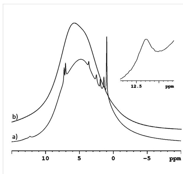
**Figure 2:**  $^1\text{H}$  MAS NMR spectra of a) CDNS(1:8)-IbuNa and b) CDNS(1:8). The inset (top right) shows the expansion of the spectral region where the hydrogen bonded protons of the carboxylic functional groups resonate. The notation CDNS-IbuNa indicates the original preparation, irrespective of the conversion of the sodium salt into the undissociated acid.
