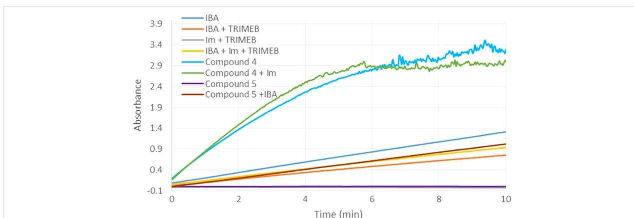
**Figure 8:** Hydrolysis of methyl paraoxon (0.5 mM) in the presence of mixtures of compounds **4**, **5** with IBA or imidazole and in the presence of a mixture of TRIMEB, 2-iodosobenzoic acid (IBA) and imidazole. The final concentrations of compounds **4**, **5**, 2-iodosobenzoic acid (IBA), imidazole and TRIMEB were 0.5 mM.
