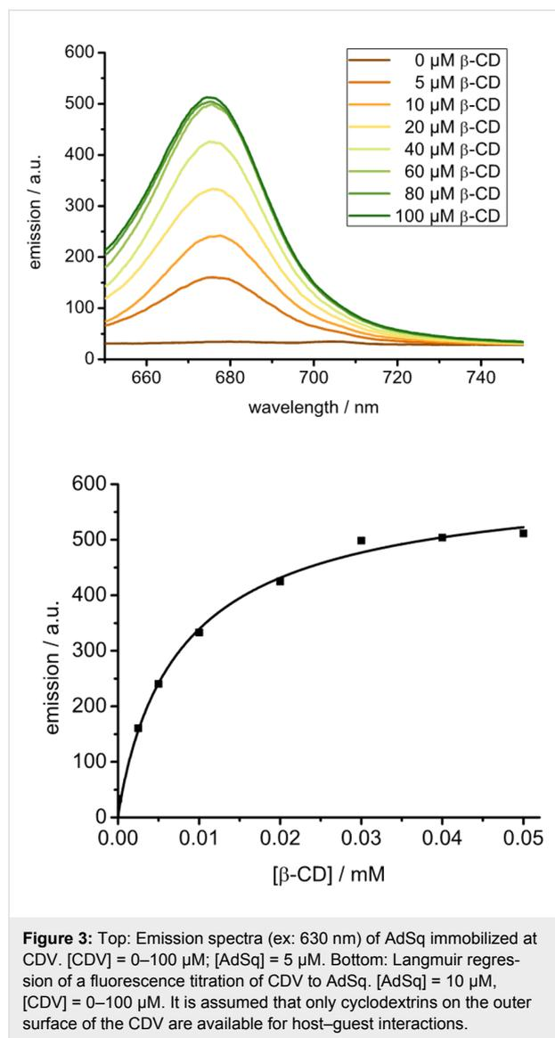
**Figure 3:** Top: Emission spectra (ex: 630 nm) of AdSq immobilized at CDV. [CDV] = 0–100  $\mu$ M; [AdSq] = 5  $\mu$ M. Bottom: Langmuir regression of a fluorescence titration of CDV to AdSq. [AdSq] = 10  $\mu$ M, [CDV] = 0–100  $\mu$ M. It is assumed that only cyclodextrins on the outer surface of the CDV are available for host–guest interactions.
