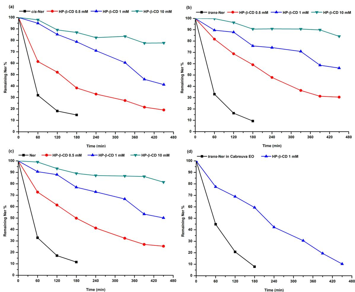
**Figure 5:** Photodegradation kinetics of *cis*-Ner (a), *trans*-Ner (b), the isomer mixture Ner (c) in the absence and presence of increasing concentrations of HP- $\beta$ -CD (0.5, 1 and 10 mM) and of *trans*-Ner in cabreuva EO (d) in the absence and presence of 1 mM HP- $\beta$ -CD under UV light irradiation.
