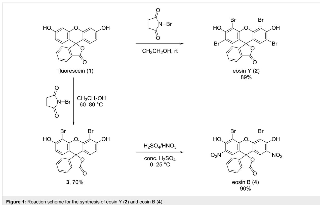
**Figure 1:** Reaction scheme for the synthesis of eosin Y (**2**) and eosin B (**4**).
