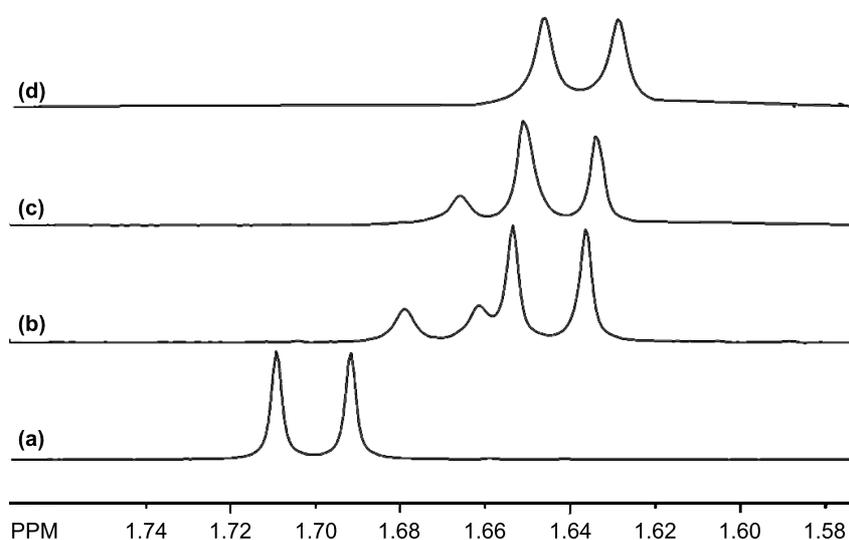
**Figure 3:** The (a) C-methyl resonance of **3** (10 mM, enriched in the (R)-enantiomer) in the presence of (b) P- $\alpha$ -CD-H<sub>DS</sub> (10 mM), (c) P- $\beta$ -CD-H<sub>DS</sub> (10 mM) and (d) P- $\gamma$ -CD-H<sub>DS</sub> (10 mM).
