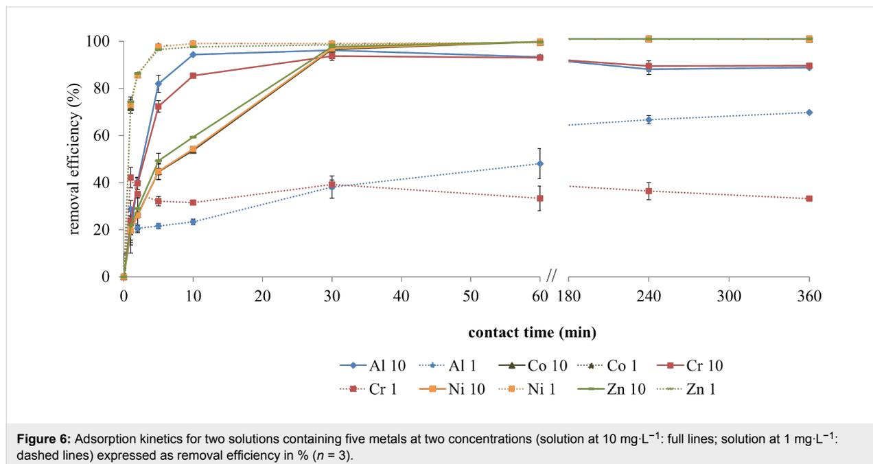
**Figure 6:** Adsorption kinetics for two solutions containing five metals at two concentrations (solution at 10 mg·L<sup>-1</sup>: full lines; solution at 1 mg·L<sup>-1</sup>: dashed lines) expressed as removal efficiency in % (n = 3).
