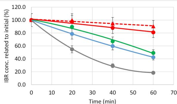
**Figure 6:** Photodegradation of IBR in distilled water examining the drug itself (blue circle), and in the presence of 1% CMBCD-P (green circle), of 0.02% nanoTiO<sub>2</sub> (grey circle), 0.02% nanoTiO<sub>2</sub> stabilized by 1% CMBCD-P (red circle), and 0.02% nanoTiO<sub>2</sub> stabilized by 1% CMBCD-P in tap water (red triangle).
