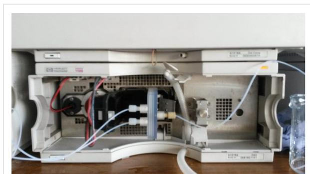
**Figure 4:** RD1 held in place within the DAD compartment of an Agilent 1100 HPLC.
