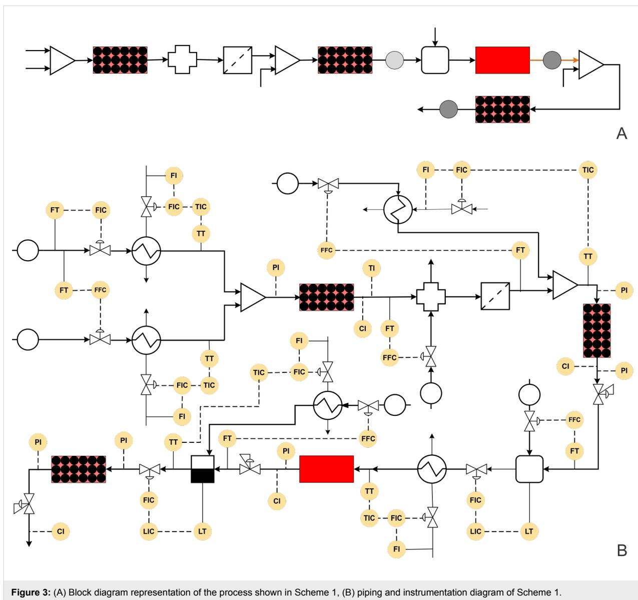
**Figure 3:** (A) Block diagram representation of the process shown in Scheme 1, (B) piping and instrumentation diagram of Scheme 1.
