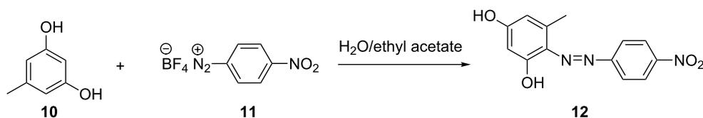
Scheme 4: Phase transfer catalyzed azo coupling of 5-methylresorcinol in microreactors.
