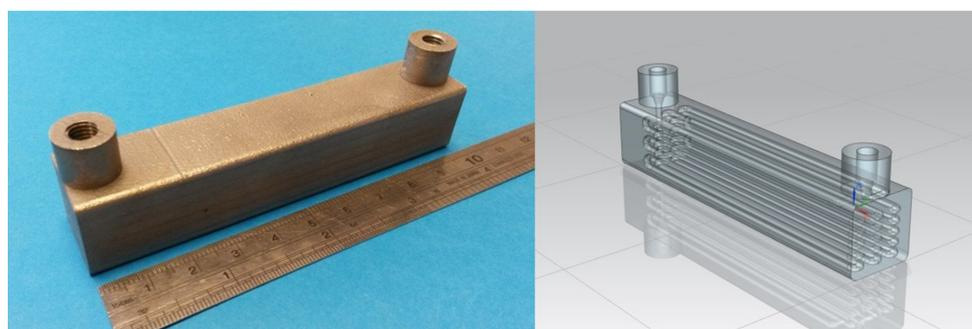
**Figure 6:** SLM reactor RD2 (left), CAD model of RD2 (right). External dimensions of RD2 are 100 (length) × 20 (width) × 20 mm (depth).
