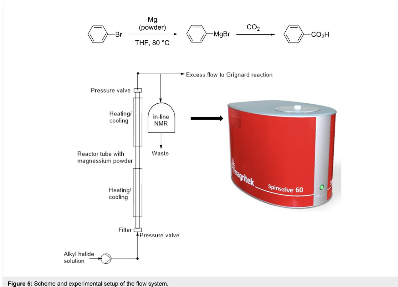
both acquisition and maintenance, and they require special laboratory installation. Benchtop NMR instruments have low cost and low maintenance; they can be easily placed in a conventional laboratory fume hood and transported to the required place.
