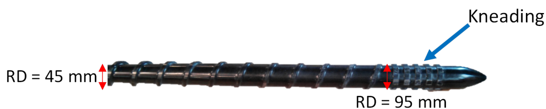
Figure 2: PTFE screw employed in single screw extrusion, with increasing root diameter (RD) from 45 mm to 95 mm and a final kneading section.
