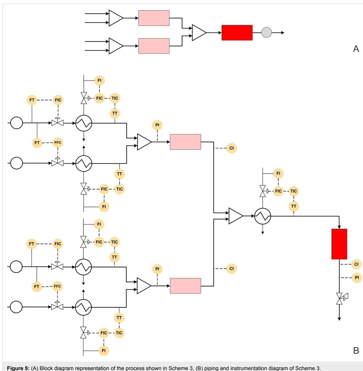
**Figure 5:** (A) Block diagram representation of the process shown in Scheme 3, (B) piping and instrumentation diagram of Scheme 3.
