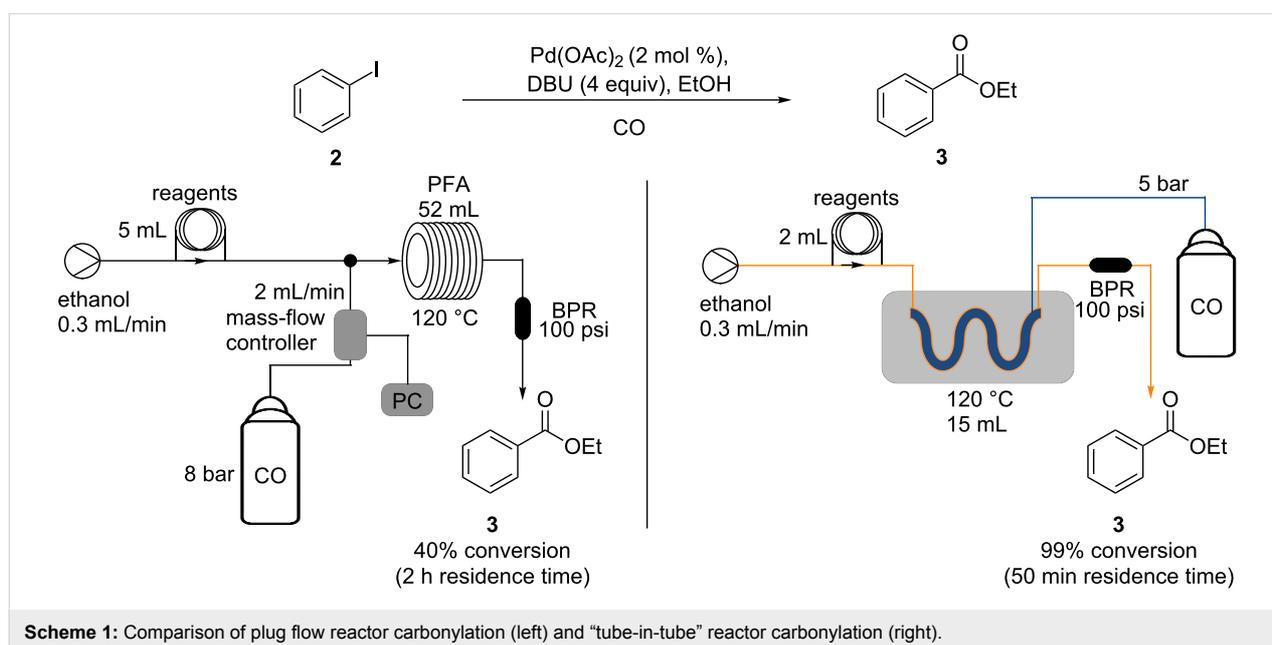
Scheme 1: Comparison of plug flow reactor carbonylation (left) and “tube-in-tube” reactor carbonylation (right).
