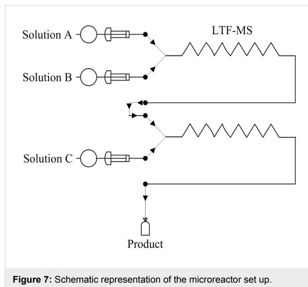
**Figure 7:** Schematic representation of the microreactor set up.
