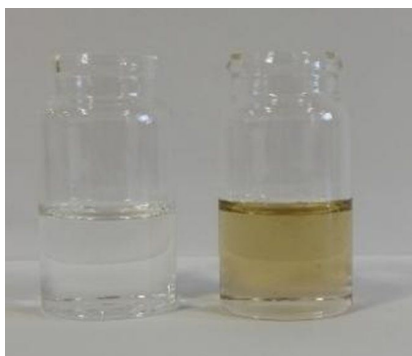
Figure 5: Comparison of choline chloride/D-fructose DES prepared via twin screw extrusion (left) and conventional heating (right). Taken from [44].
