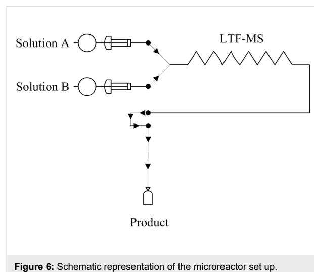
**Figure 6:** Schematic representation of the microreactor set up.
