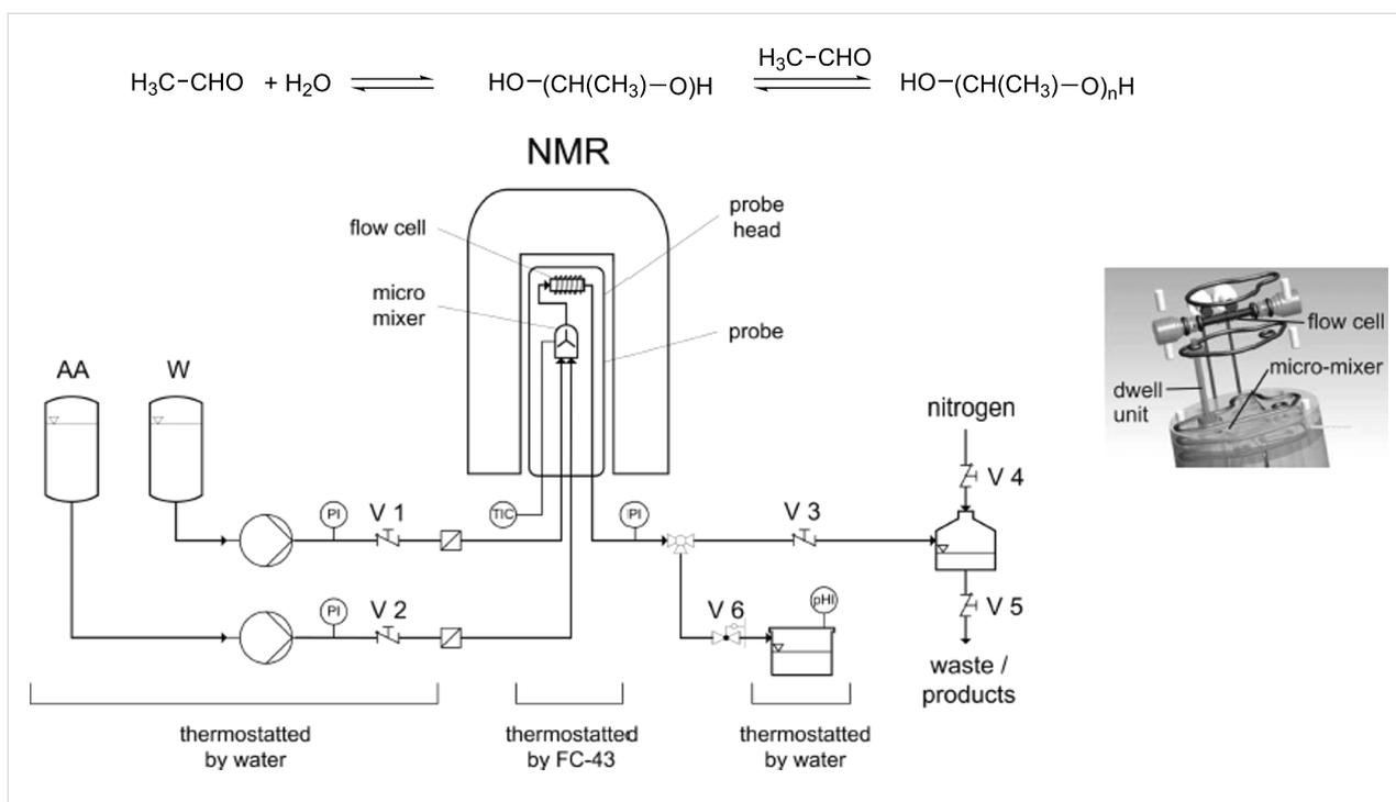
**Figure 9:** Flowsheet of the experimental setup used to study the reaction kinetics of the oligomer formation in mixtures of acetaldehyde (AA) and water (A) (Flow rates  $V_{AA}$  254  $\mu\text{L min}^{-1}$  and  $V_W$  748  $\mu\text{L min}^{-1}$ ). Reproduced with permission from reference [46]. Copyright 2014 The American Chemical Society.
