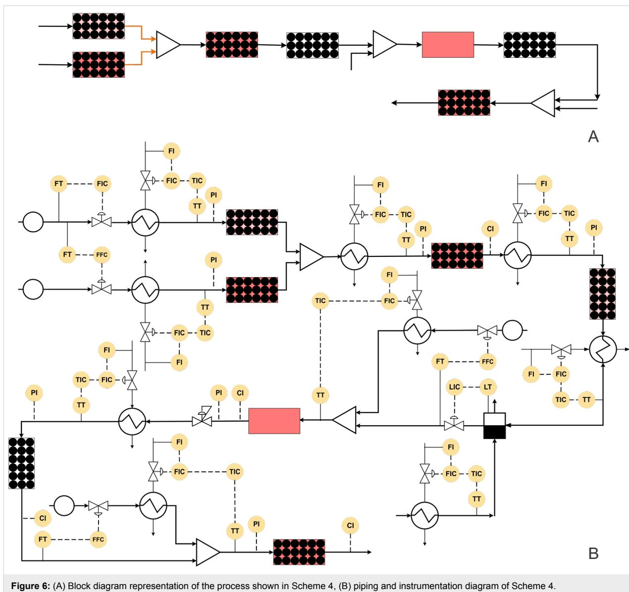
**Figure 6:** (A) Block diagram representation of the process shown in Scheme 4, (B) piping and instrumentation diagram of Scheme 4.
