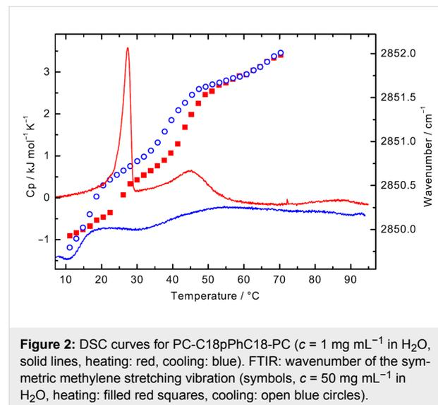
**Figure 2:** DSC curves for PC-C18pPhC18-PC ( $c = 1 \text{ mg mL}^{-1}$  in  $\text{H}_2\text{O}$ , solid lines, heating: red, cooling: blue). FTIR: wavenumber of the symmetric methylene stretching vibration (symbols,  $c = 50 \text{ mg mL}^{-1}$  in  $\text{H}_2\text{O}$ , heating: filled red squares, cooling: open blue circles).
