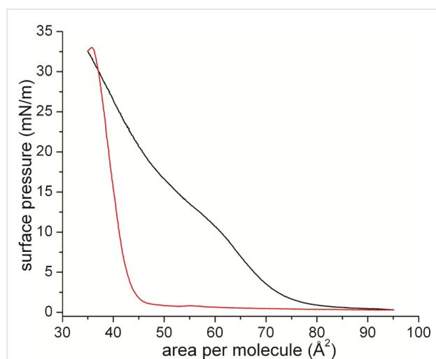
**Figure 2:** Langmuir–Pockels isotherm of a monolayer of flipper mechanophores during the first compression (black) and subsequent expansion (red) at the air/water interface at 20 °C subphase temperature and 22 °C air temperature.
