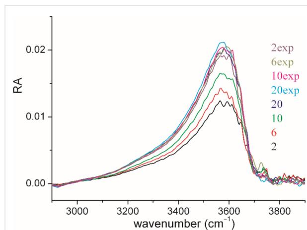
**Figure 3:** OH-stretching vibration ( $\nu(\text{OH})$ ;  $3600 \text{ cm}^{-1}$ ) for IRRAS spectra of a flipper mechanophore monolayer during compression (2, 6, 10, and  $20 \text{ mN/m}$ ) and expansion (20, 10, 6,  $2 \text{ mN/m}$ ). The increase of intensity up to  $20 \text{ mN/m}$  indicates an increase of the effective layer thickness. It is important to note that the OH-band intensity does not change during expansion.
