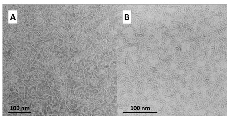
**Figure 3:** TEM image of an aqueous suspension ( $c = 0.05 \text{ mg mL}^{-1}$ ) of PC-C18pPhC18-PC. The samples were prepared at about  $7 \text{ }^\circ\text{C}$  (A) or at  $36 \text{ }^\circ\text{C}$  (B) and stained with uranyl acetate before drying.
