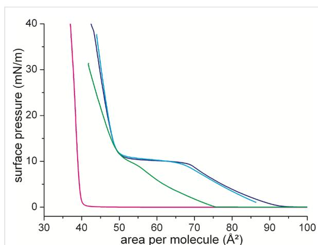
**Figure 4:** Isotherms of DPPC (dark blue), cholesterol (magenta), DPPC/cholesterol (8:2 mol/mol, green), and DPPC/flipper (8:2 mol/mol, blue) measured on water at 25 °C. The area in the mixture is given as area per DPPC molecule.
