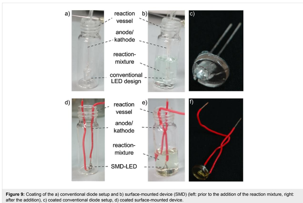
ferent LED designs were investigated, a conventional diode setup as well as a much smaller surface mounted device (SMD).
