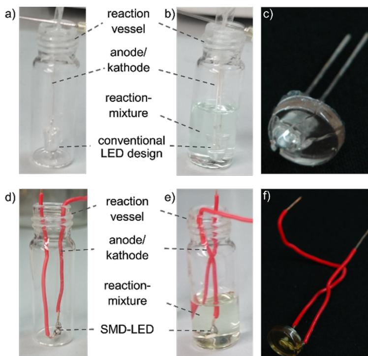
**Figure 9:** Coating of the a) conventional diode setup and b) surface-mounted device (SMD) (left: prior to the addition of the reaction mixture, right: after the addition), c) coated conventional diode setup, d) coated surface-mounted device.
