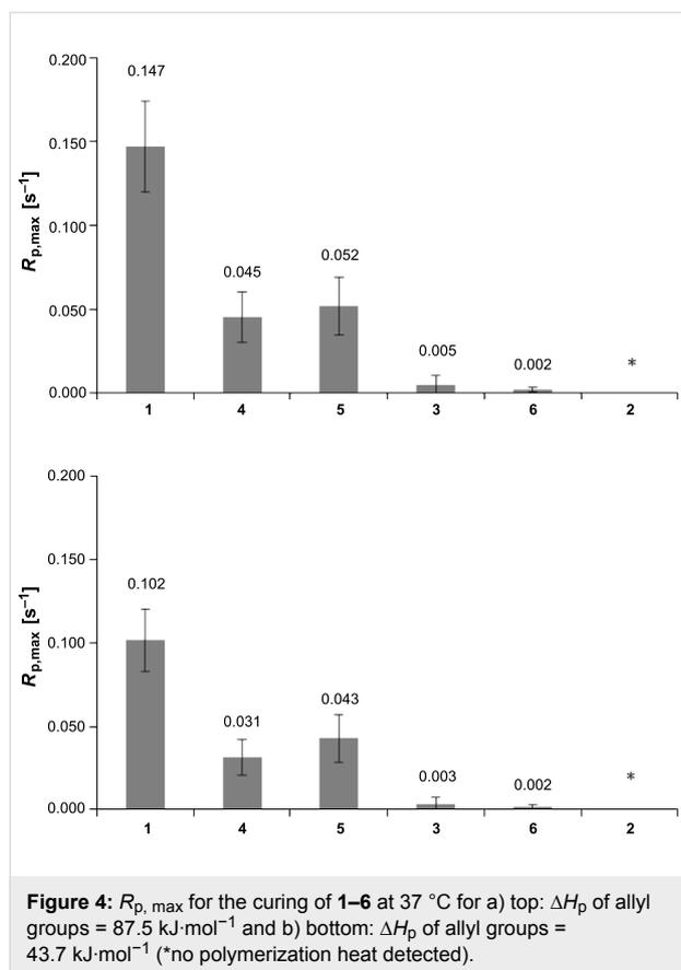
by a different work group (0.032) [34]. Interestingly, equipping the amide  $\alpha$ -carbon with a methyl group (1→4) led to a ~70% decrease of  $R_{p,max}$  from 0.147/0.102 to 0.045/0.031, indicating the special role of the internal double bond. Also, when
