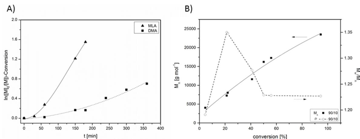
**Figure 10:** A) Kinetic plot for the RAFT copolymerization of MLA and DMA for the ratio 90/10 employing EMP. B) The evolution of  $M_n$  (full symbols) and  $\bar{D}$  (empty symbols) with conversion of the copolymerization.
