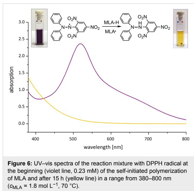
lation, Supporting Information File 1) [19]. The constant  $Q$  reflects the resonance stabilization of the growing radical. Large  $Q$  values ( $>0.5$ ) indicate stabilized monomers. The constant  $e$  reflects the polarity of the double bond and of the growing radical. For instance positive  $e$  values point to an electrophilic character while negative  $e$  values point to a nucleophilic character.
