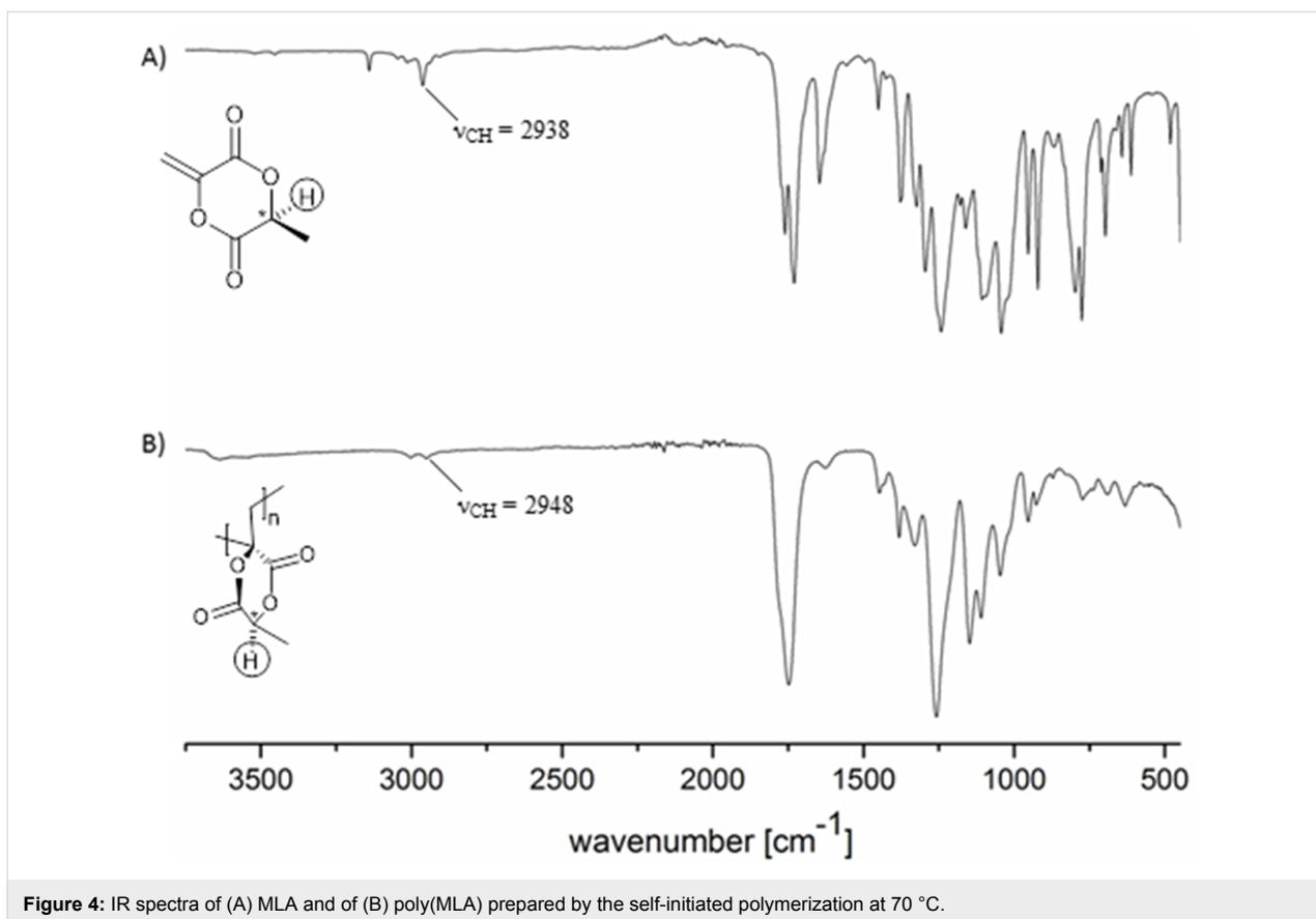
**Figure 4:** IR spectra of (A) MLA and of (B) poly(MLA) prepared by the self-initiated polymerization at 70 °C.
