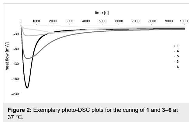
**Figure 2:** Exemplary photo-DSC plots for the curing of **1** and **3–6** at  $37^\circ\text{C}$ .
