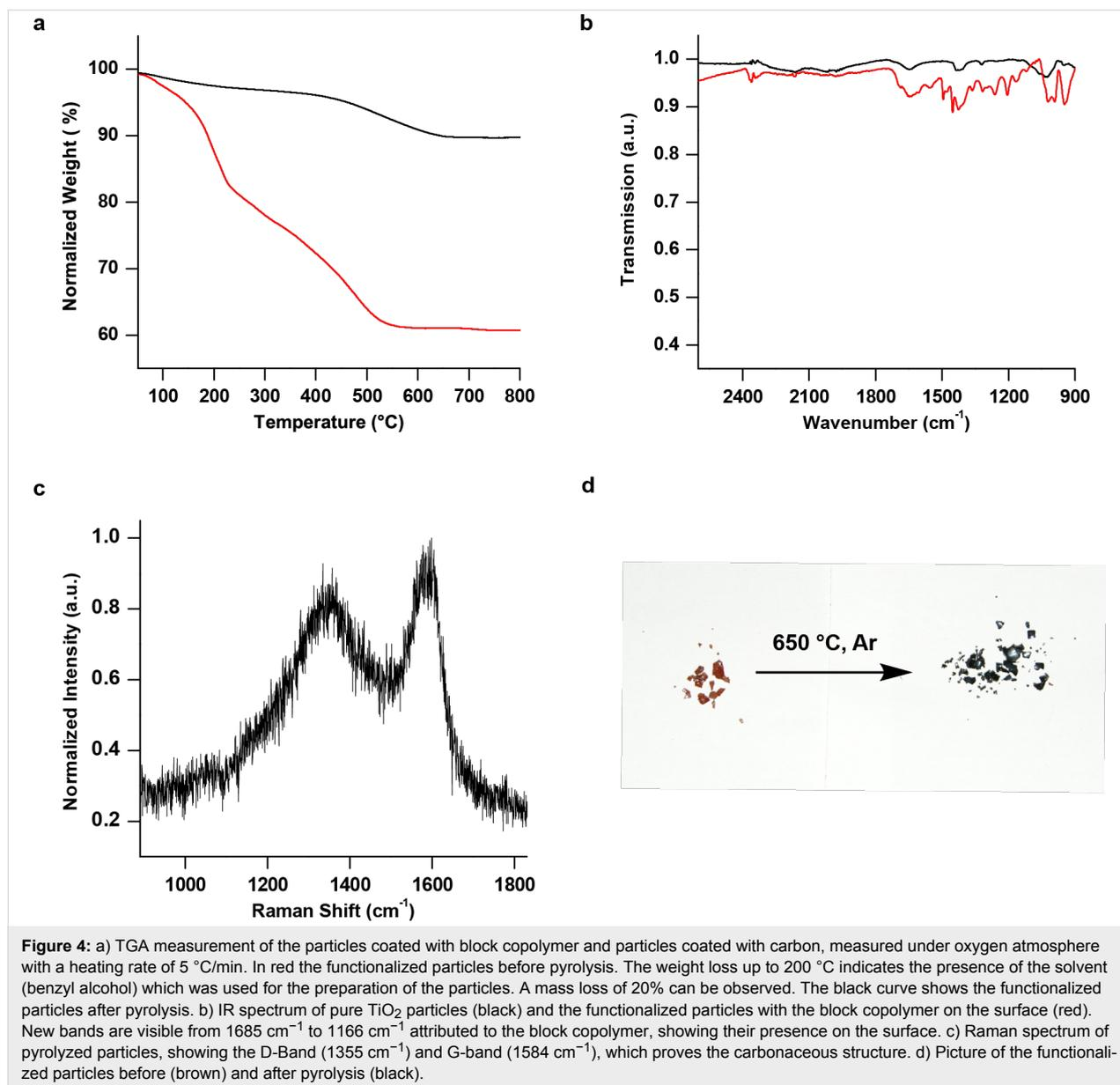
connected through lattices which might also help to provide longer paths for electrons to travel within the electrode. Summarizing, the Raman spectrum, the TGA measurements and the TEM images proves the success of the formation of a thin coating around the TiO<sub>2</sub> particles. Currently, we are investigating the application of the hybrid material in batteries.
