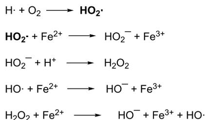
**Scheme 1:** Ionizing radiation reactions in the Fricke dosimeter.
