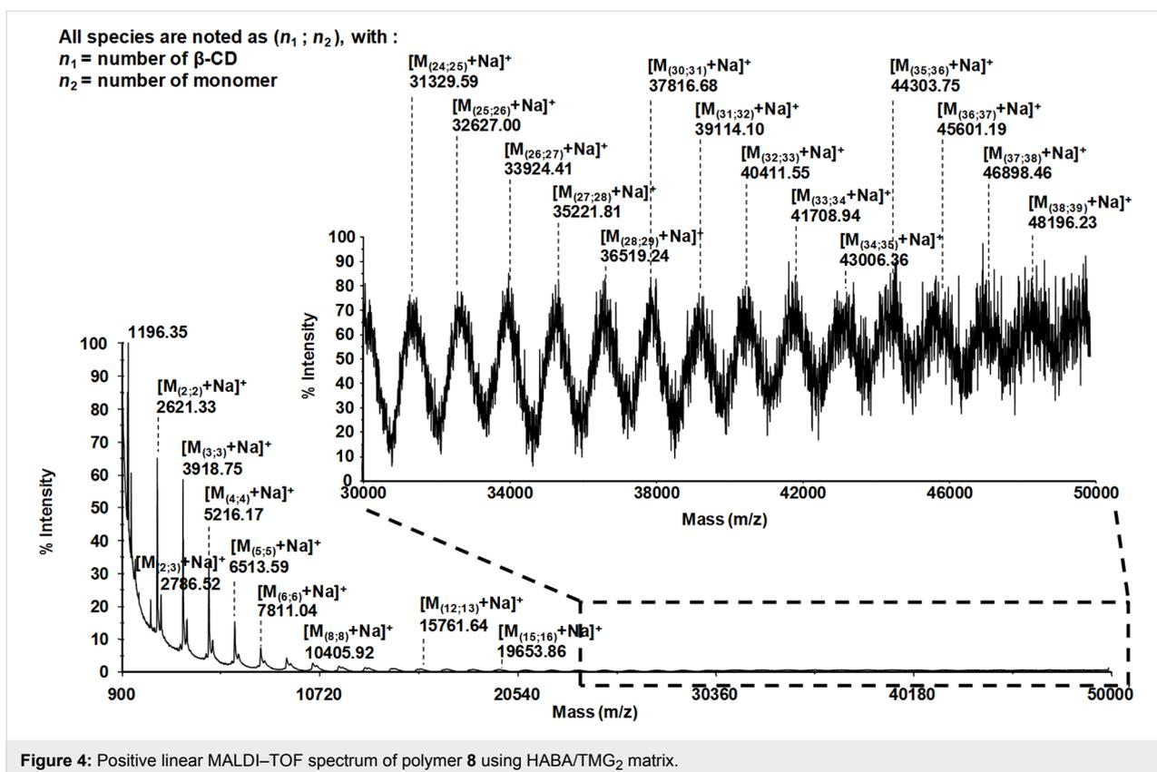
**Figure 4:** Positive linear MALDI-TOF spectrum of polymer **8** using HABA/TMG<sub>2</sub> matrix.
