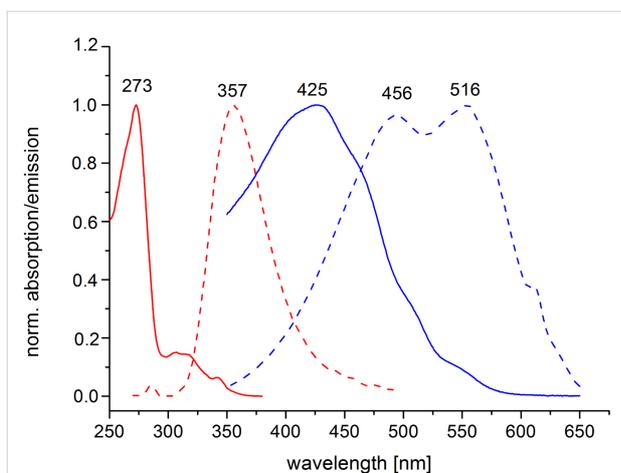
**Figure 3:** Absorption spectra of monomer **7** (solid red line) and polymer **8** (solid blue line) in water. Emission spectra of monomer **7** (dotted red line) and polymer **8** (dotted blue line) in water excited at 290 nm and 335 nm, respectively.
