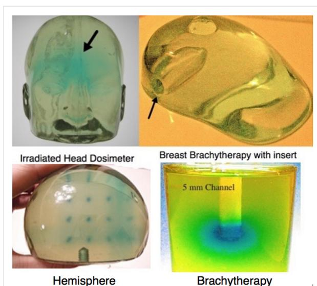
**Figure 4:** 3D dosimeters fabricated in our lab for a variety of radiation therapies. Top left a head dosimeter (12 kg); on the right a breast dosimeter with an inset for brachytherapy; bottom left an irradiated hemisphere; bottom right a cylindrical brachytherapy dosimeter with 5 mm channel for insert the radiation seed.
