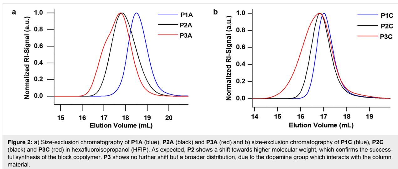
**Figure 2:** a) Size-exclusion chromatography of **P1A** (blue), **P2A** (black) and **P3A** (red) and b) size-exclusion chromatography of **P1C** (blue), **P2C** (black) and **P3C** (red) in hexafluoroisopropanol (HFIP). As expected, **P2** shows a shift towards higher molecular weight, which confirms the successful synthesis of the block copolymer. **P3** shows no further shift but a broader distribution, due to the dopamine group which interacts with the column material.
