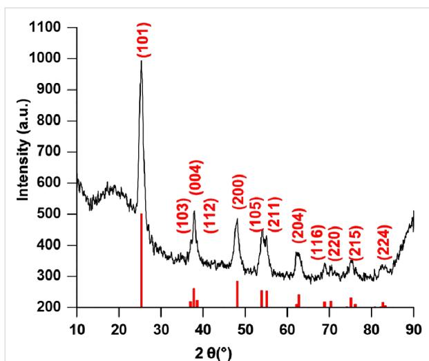
Figure 5: PXRD pattern of carbon-coated TiO<sub>2</sub> particles.
