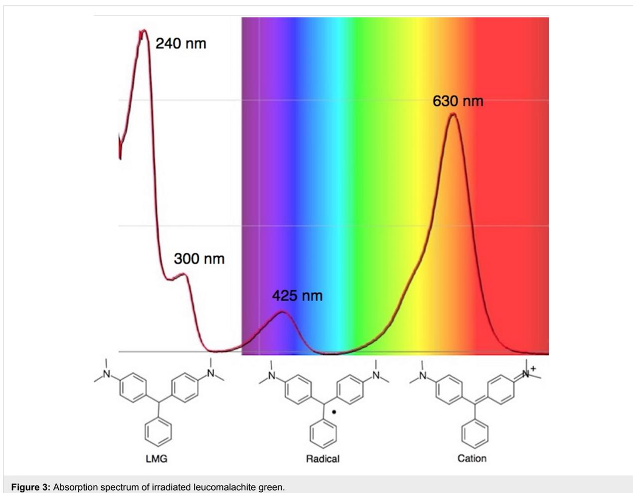
**Figure 3:** Absorption spectrum of irradiated leucomalachite green.
