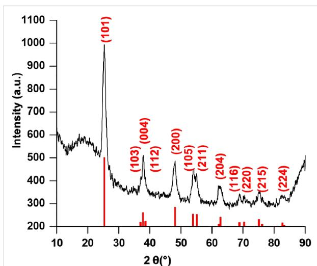
Figure 5: PXRD pattern of carbon-coated TiO<sub>2</sub> particles.
