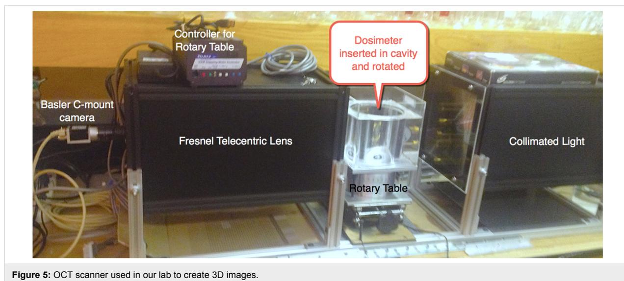
Figure 5: OCT scanner used in our lab to create 3D images.
