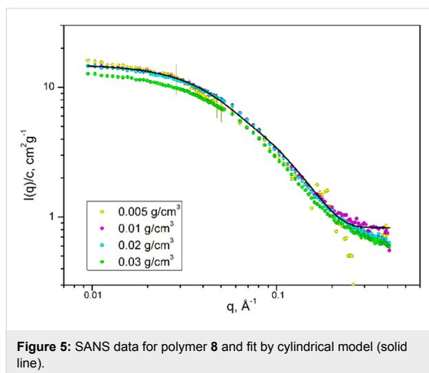
**Figure 5:** SANS data for polymer **8** and fit by cylindrical model (solid line).
