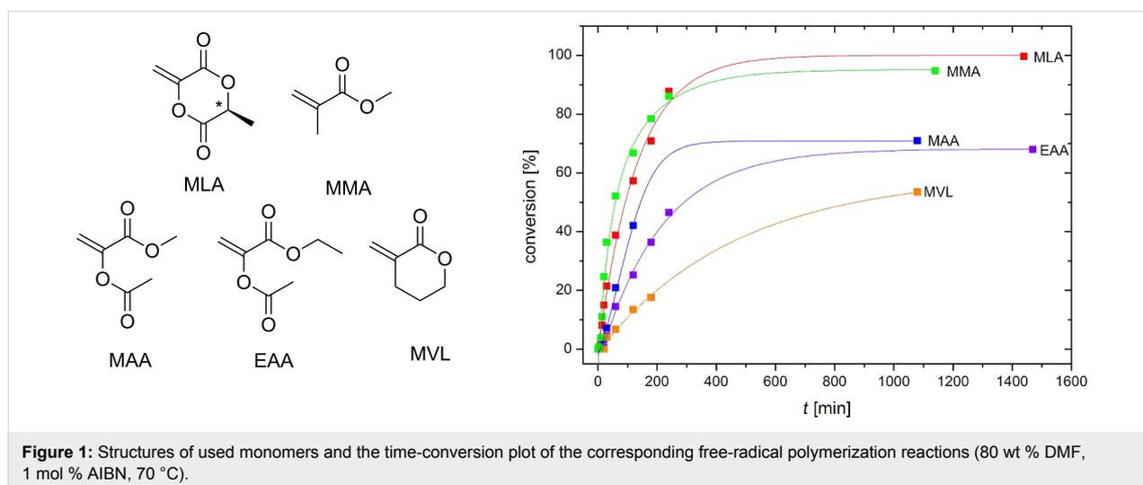
**Figure 1:** Structures of used monomers and the time-conversion plot of the corresponding free-radical polymerization reactions (80 wt % DMF, 1 mol % AIBN, 70 °C).
