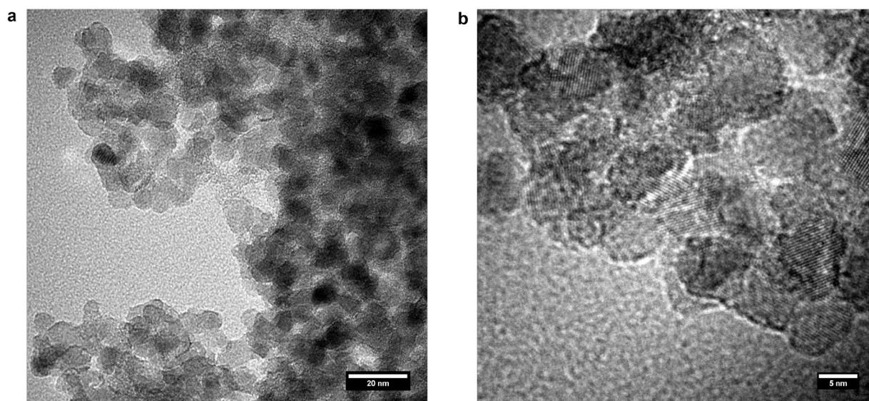
Figure 6: TEM images of the carbon coated TiO<sub>2</sub> nanoparticles.
