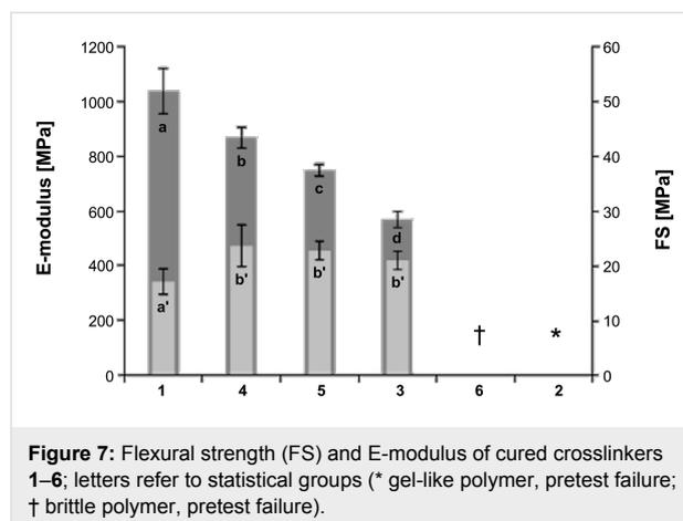
**Figure 7:** Flexural strength (FS) and E-modulus of cured crosslinkers **1–6**; letters refer to statistical groups (\* gel-like polymer, pretest failure; † brittle polymer, pretest failure).
