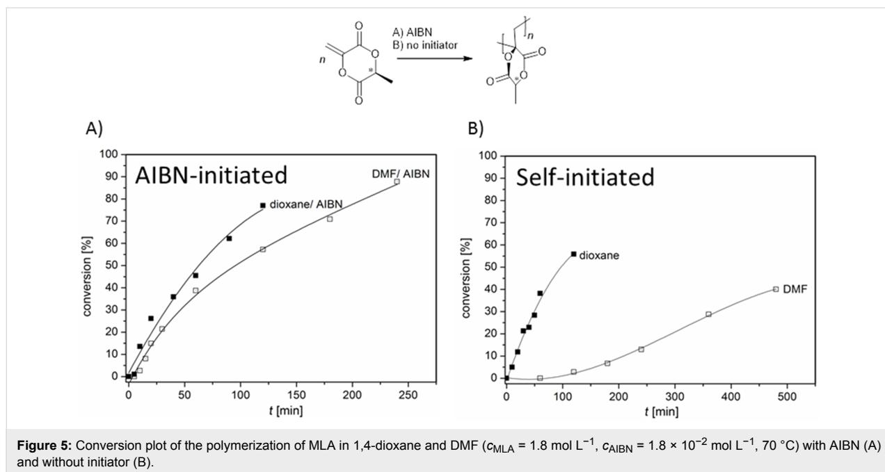
**Figure 5:** Conversion plot of the polymerization of MLA in 1,4-dioxane and DMF ( $c_{\text{MLA}} = 1.8 \text{ mol L}^{-1}$ ,  $c_{\text{AIBN}} = 1.8 \times 10^{-2} \text{ mol L}^{-1}$ , 70 °C) with AIBN (A) and without initiator (B).
