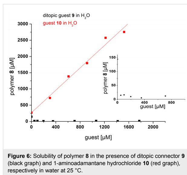
**Figure 6:** Solubility of polymer **8** in the presence of ditopic connector **9** (black graph) and 1-aminoadamantane hydrochloride **10** (red graph), respectively in water at 25 °C.
