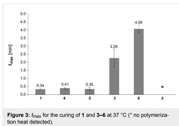
**Figure 3:**  $t_{\max}$  for the curing of **1** and **3–6** at  $37^\circ\text{C}$  (\* no polymerization heat detected).
