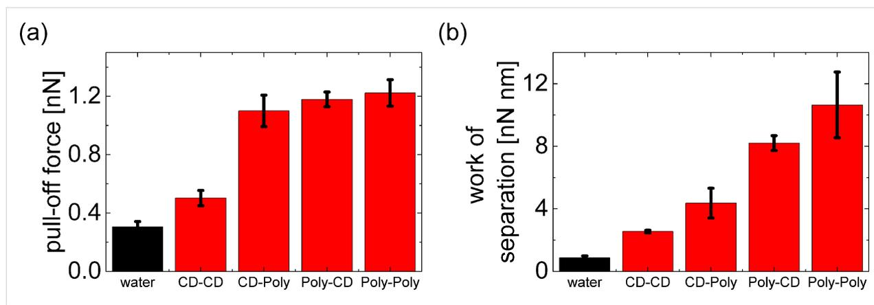
**Figure 8:** Graphical summary of experimental results for the four configurations of CD attachment introduced in Figure 2: (a) pull-off forces, (b) work of separation. The error bars indicate standard deviations for averages over different lateral positions on the functionalized surface.
