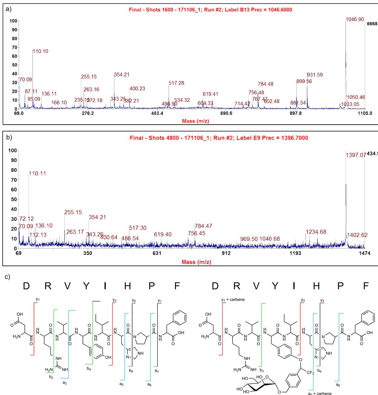
**Figure 4:** MS/MS spectra of angiotensin II (a) and of angiotensin II, photo-crosslinked with diazirine **2** (b), recorded on 4700 Proteomics Analyzer mass spectrometer (Applied Biosystems); (c) fragments of angiotensin II and photo-crosslinked angiotensin II according to Biemann's nomenclature (Table 3).
