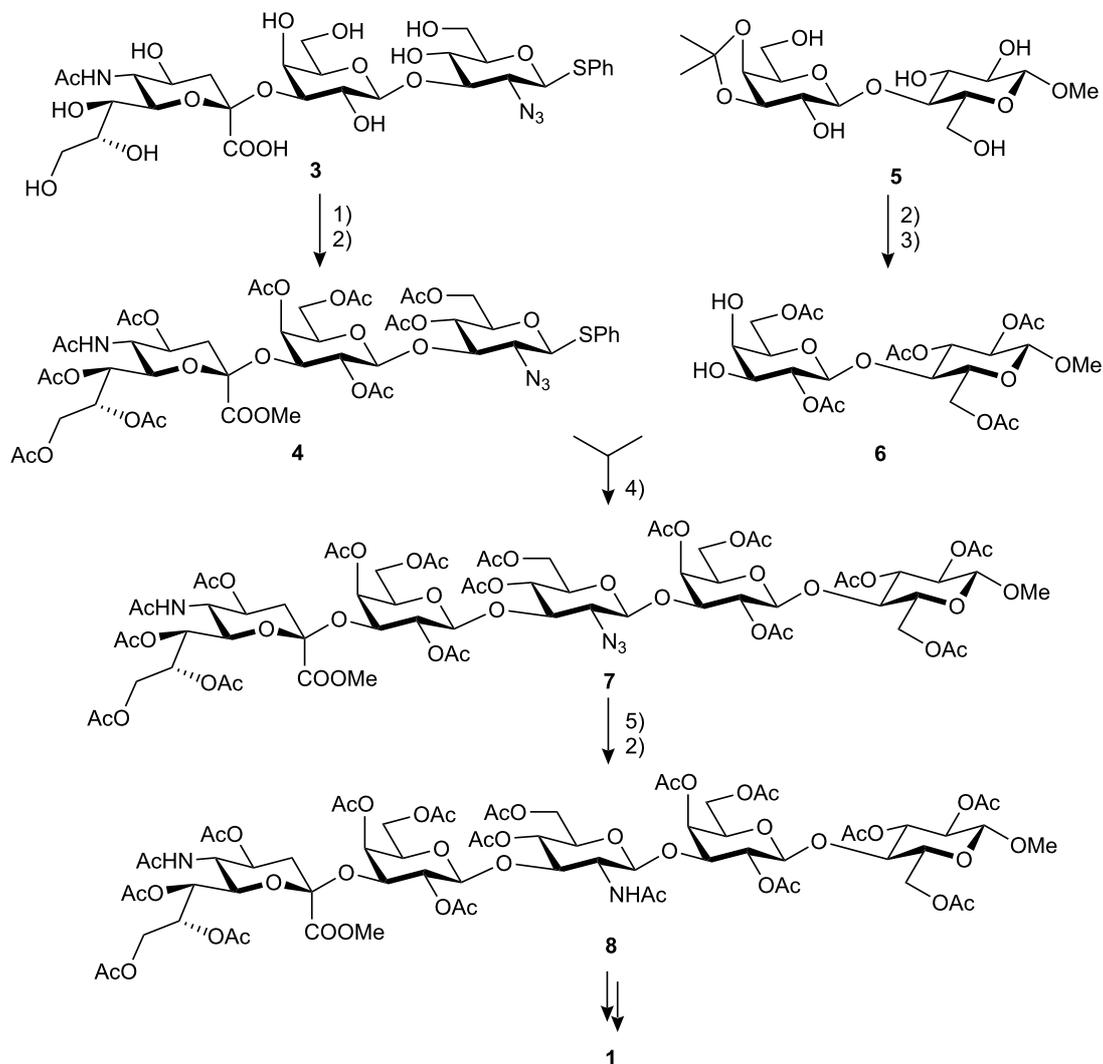
**Scheme 1:** Preparation of pentasaccharide **8**. 1) MeOH, acidic ion exchange resin; 2) Ac<sub>2</sub>O, pyridine; 3) 80% HOAc, 90 °C; 4) NIS, CF<sub>3</sub>SO<sub>3</sub>H, 61%; 5) NiCl<sub>2</sub>·6H<sub>2</sub>O, H<sub>3</sub>BO<sub>3</sub>, EtOH, then NaBH<sub>4</sub>, EtOH and acidic workup.
