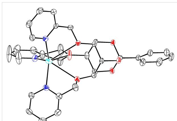
**Figure 3:** ORTEP drawing for the 1:Ag(I) cation complex (ellipsoids are drawn at the 50% probability level and H atoms are omitted for clarity).
