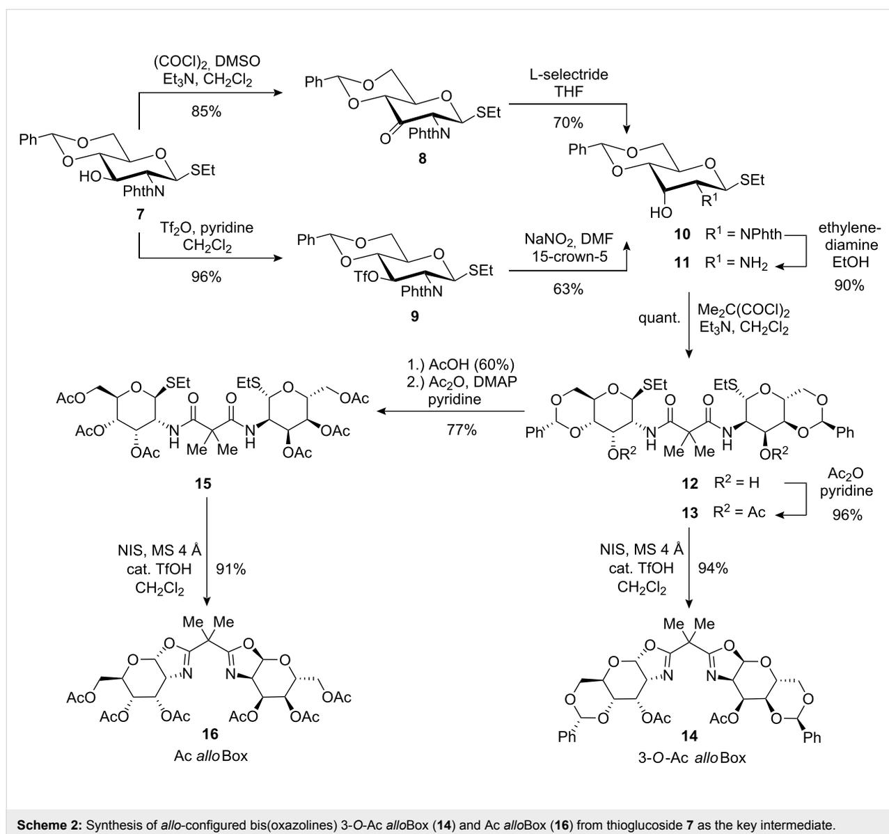
**Scheme 2:** Synthesis of *allo*-configured bis(oxazolines) 3-*O*-Ac *allo*Box (**14**) and Ac *allo*Box (**16**) from thioglucoside **7** as the key intermediate.
