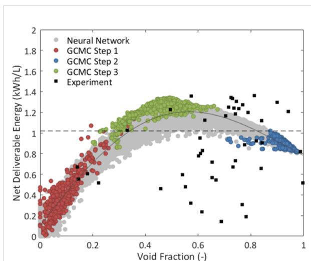
**Figure 14:** Net deliverable energy as a function of porous material void fraction at 77 K cycling between 100 and 1 bar. Predictions include the GCMC-simulated sample sets for three rounds of evolution (colours), and the final neural network model for the complete genome (grey). Experimental data from the literature is shown as black squares. Adapted with permission from [48]; copyright 2017 American Chemical Society.
