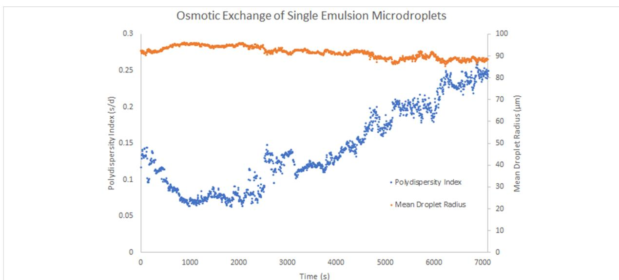
**Figure 5:** Real-time, LabVIEW™ tracking of osmosis-driven coarsening of 50 mM glycylglycine and pure water droplets. Increase in droplet polydispersity is monitored using LabVIEW™ image analysis.  $s$  = standard deviation of droplet radius,  $d$  = mean radius.
