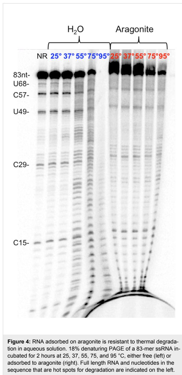
**Figure 4:** RNA adsorbed on aragonite is resistant to thermal degradation in aqueous solution. 18% denaturing PAGE of a 83-mer ssRNA incubated for 2 hours at 25, 37, 55, 75, and 95 °C, either free (left) or adsorbed to aragonite (right). Full length RNA and nucleotides in the sequence that are hot spots for degradation are indicated on the left.
