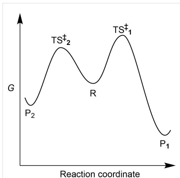
**Figure 2:** Kinetic control. In many chemical reactions leading to different products, the final composition is determined by the height of the kinetic barriers corresponding to transition states ( $TS^{\ddagger}_1$  and  $TS^{\ddagger}_2$ ) rather than by the relative free energies of reactant (**R**) and products (**P**<sub>1</sub> and **P**<sub>2</sub>). Under kinetic control, **P**<sub>2</sub> would be favoured over **P**<sub>1</sub>.
