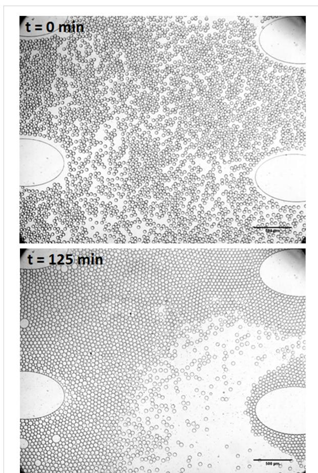
**Figure 4:** Osmotic exchange and coarsening of co-incubating aqueous microdroplets. 50 mM glycylglycine and pure H<sub>2</sub>O droplets were co-incubated in the same chamber. Upper panel: mixed but monodisperse droplet population at  $t = 0$  min; lower panel:  $t = 125$  min.
