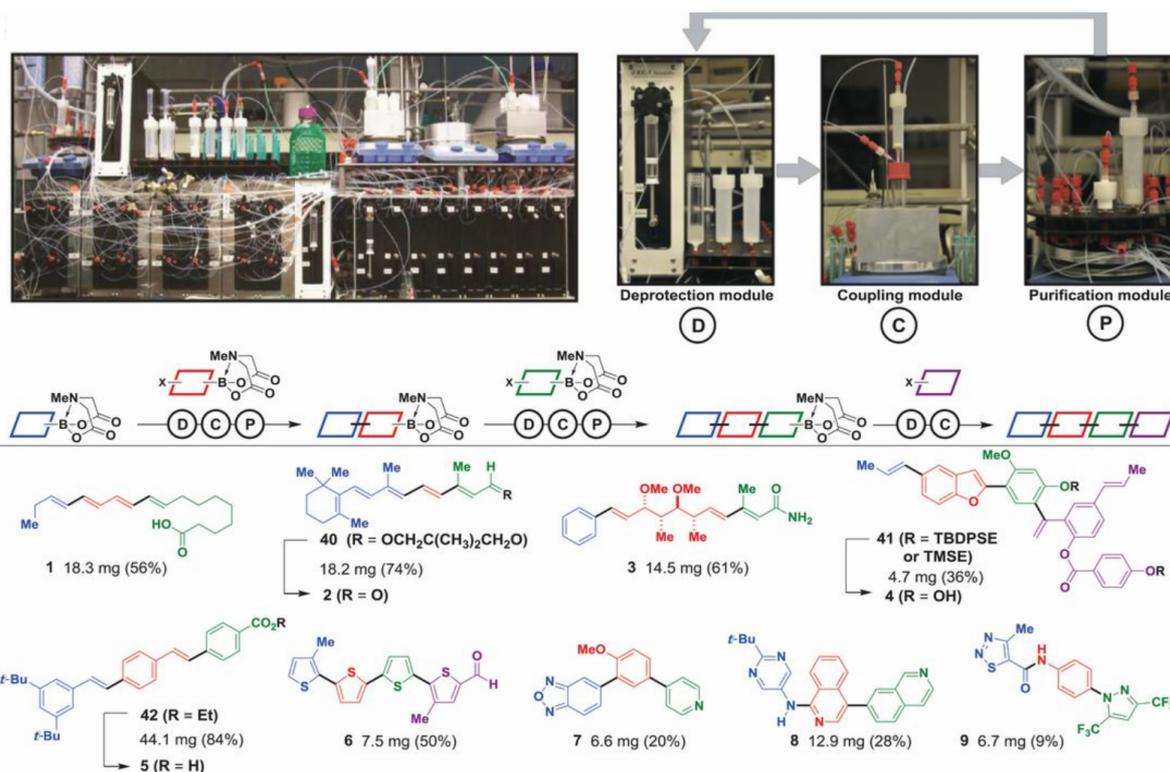
**Figure 9:** (Top) Photograph of a small-molecule synthesizer comprised of three modules for deprotection, coupling, and purification steps. (Bottom) Natural products, materials, pharmaceuticals, and biological probes synthesized by automated synthesis by iterative coupling of different building blocks (colors). TBDPSE, *tert*-butyldiphenylsilylethyl; TMSE, trimethylsilylethyl. Adapted with permission from [37]; copyright 2015 American Association for the Advancement of Science.
