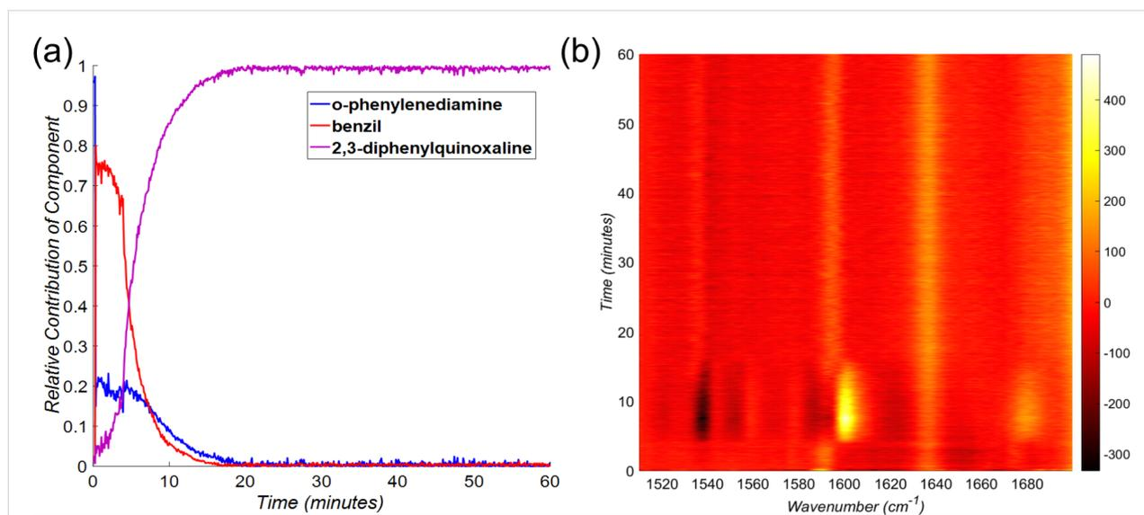
**Figure 3:** (Left) Estimated contribution of each component for each Raman spectrum over time of the synthesis of 2,3-diphenylquinoxaline at 30 Hz. (Right) Residual plot of the difference between experimental and estimated Raman spectra. In this case, this plot suggests an overestimation of 2,3-diphenylquinoxaline and an underestimation of o-phenylenediamine between  $\approx 5$  and  $\approx 15$  minutes. More information on the fitting can be found in Supporting Information File 1.
