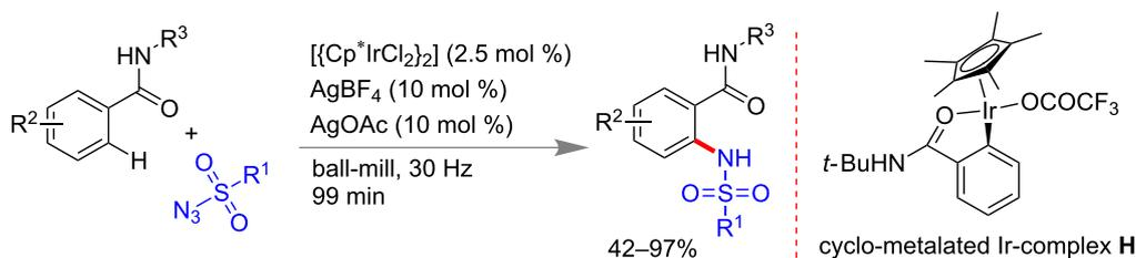
**Scheme 51:** Mechanochemical  $\text{C}_{\text{sp}^2}$ -H bond amidation using Ir(III) catalyst [183].
