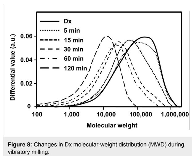
**Figure 8:** Changes in Dx molecular-weight distribution (MWD) during vibratory milling.
