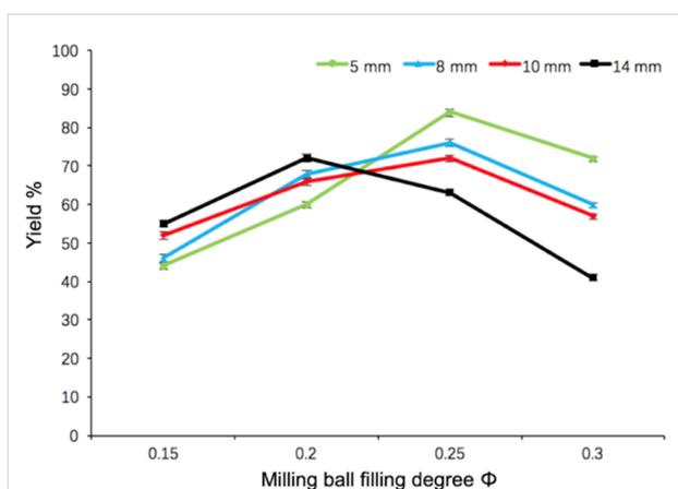
**Figure 2:** Examination of the milling-ball filling degree ( $\Phi_{MB}$ ) and milling-ball sizes on the yield of **3aa**. Reaction conditions: **1a** (1.5 mmol), **2a** (2.1 mmol), Pd/MgAl-LDHs (2.5 mol %), TBAB (1.5 mmol), K<sub>2</sub>CO<sub>3</sub> (3.6 mmol), 5 g silica gel were placed in a 80 mL stainless-steel vessel. HSBM conditions: 60 min at 800 rpm.
