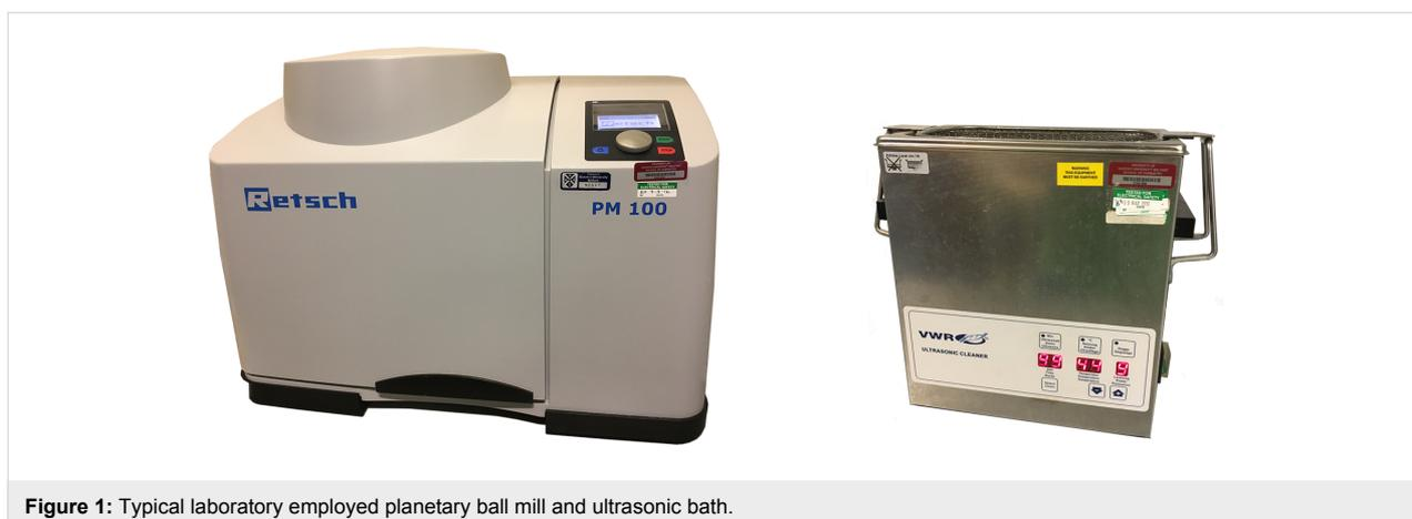
**Figure 1:** Typical laboratory employed planetary ball mill and ultrasonic bath.
