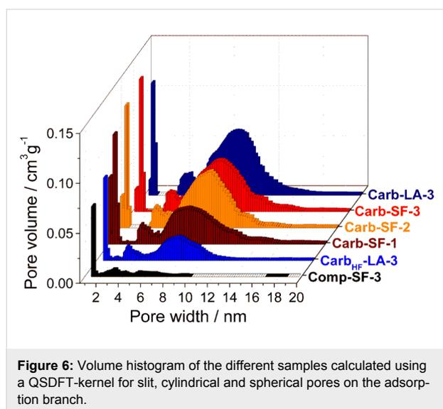
**Figure 6:** Volume histogram of the different samples calculated using a QSDFT-kernel for slit, cylindrical and spherical pores on the adsorption branch.
