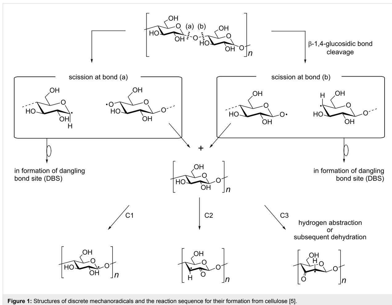
**Figure 1:** Structures of discrete mechanoradicals and the reaction sequence for their formation from cellulose [5].
