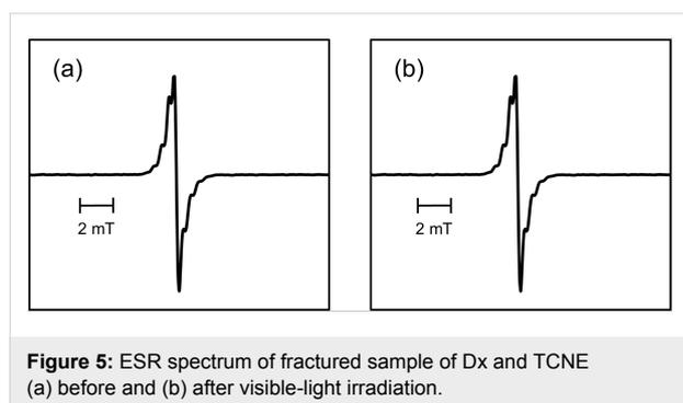
**Figure 5:** ESR spectrum of fractured sample of Dx and TCNE (a) before and (b) after visible-light irradiation.
