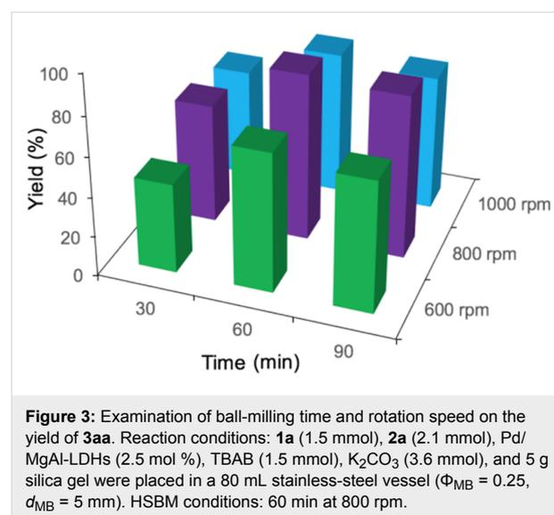
**Figure 3:** Examination of ball-milling time and rotation speed on the yield of **3aa**. Reaction conditions: **1a** (1.5 mmol), **2a** (2.1 mmol), Pd/MgAl-LDHs (2.5 mol %), TBAB (1.5 mmol), K<sub>2</sub>CO<sub>3</sub> (3.6 mmol), and 5 g silica gel were placed in a 80 mL stainless-steel vessel ( $\Phi_{MB} = 0.25$ ,  $d_{MB} = 5$  mm). HSBM conditions: 60 min at 800 rpm.
