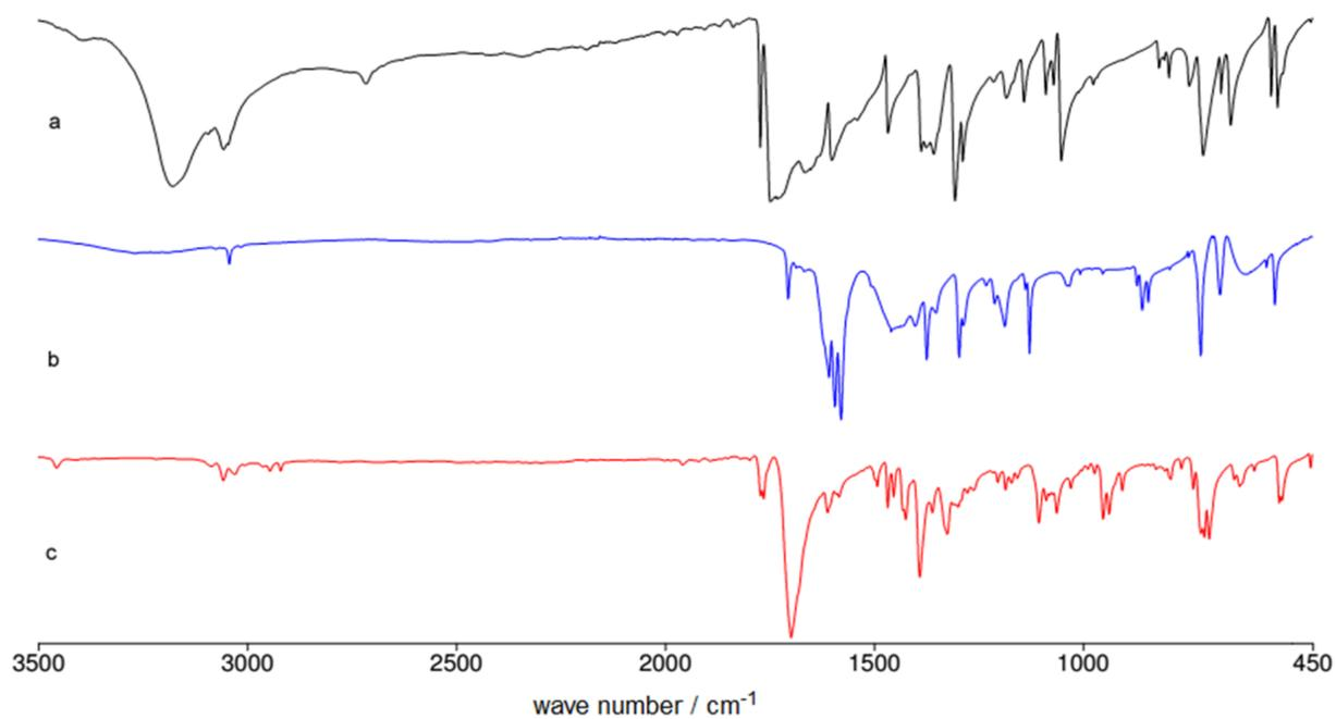
**Figure 2:** Ex situ IR spectroscopy of the reaction of **12** and benzyl bromide in the ball mill: a) phthalimide **12**; b) first step: phthalimide +  $K_2CO_3$ , 1 h milling; c) second step: addition of benzyl bromide, LAG DMF and further 1 h milling.
