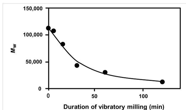
**Figure 9:** Changes in Dx weight-average molecular weight ( $M_w$ ) during vibratory milling.
