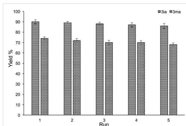
**Figure 5:** Recycling studies of the Pd/MgAl-LDH catalyst for Heck reactions. Reaction conditions: **1i** or **1m** (1.5 mmol), **2a** (2.1 mmol), Pd/MgAl-LDHs (2.5 mol %), TBAB (1.5 mmol), K<sub>2</sub>CO<sub>3</sub> (3.6 mmol), and silica gel 5 g were placed in a 80 mL stainless-steel vessel ( $\Phi_{MB} = 0.25$ ,  $d_{MB} = 5$  mm). HSBM conditions: 60 min at 800 rpm.
