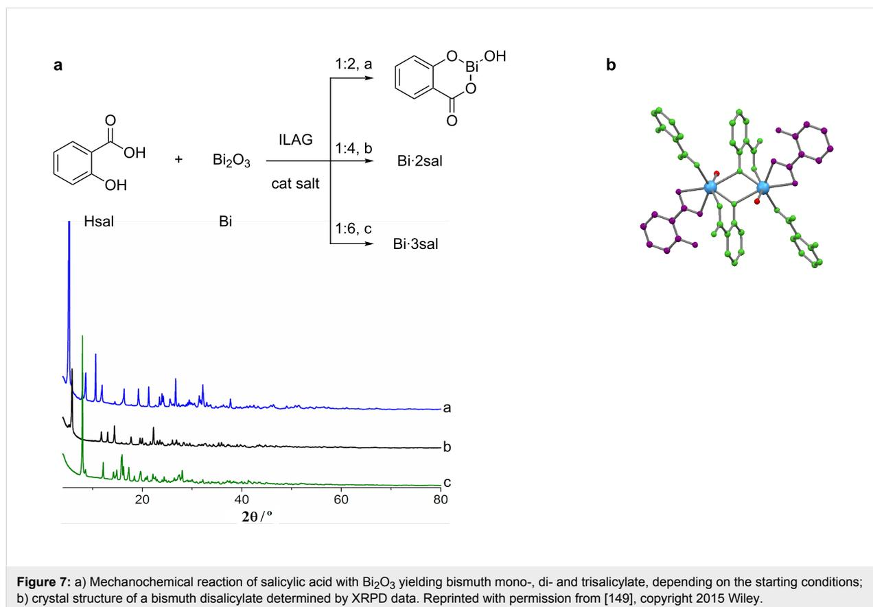
**Figure 7:** a) Mechanochemical reaction of salicylic acid with  $\text{Bi}_2\text{O}_3$  yielding bismuth mono-, di- and trisalicylate, depending on the starting conditions; b) crystal structure of a bismuth disalicylate determined by XRPD data. Reprinted with permission from [149], copyright 2015 Wiley.
