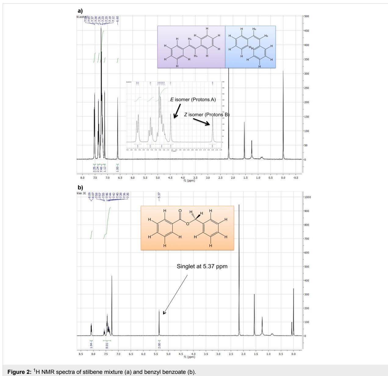
**Figure 2:** <sup>1</sup>H NMR spectra of stilbene mixture (a) and benzyl benzoate (b).
