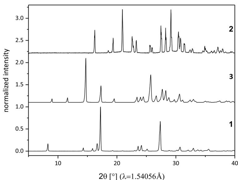
**Figure 1:** X-ray diffraction patterns of the reactants *p*-nitrobenzaldehyde (**1**) and malononitrile (**2**) and the product *p*-nitrobenzylidenemalononitrile (**3**).
