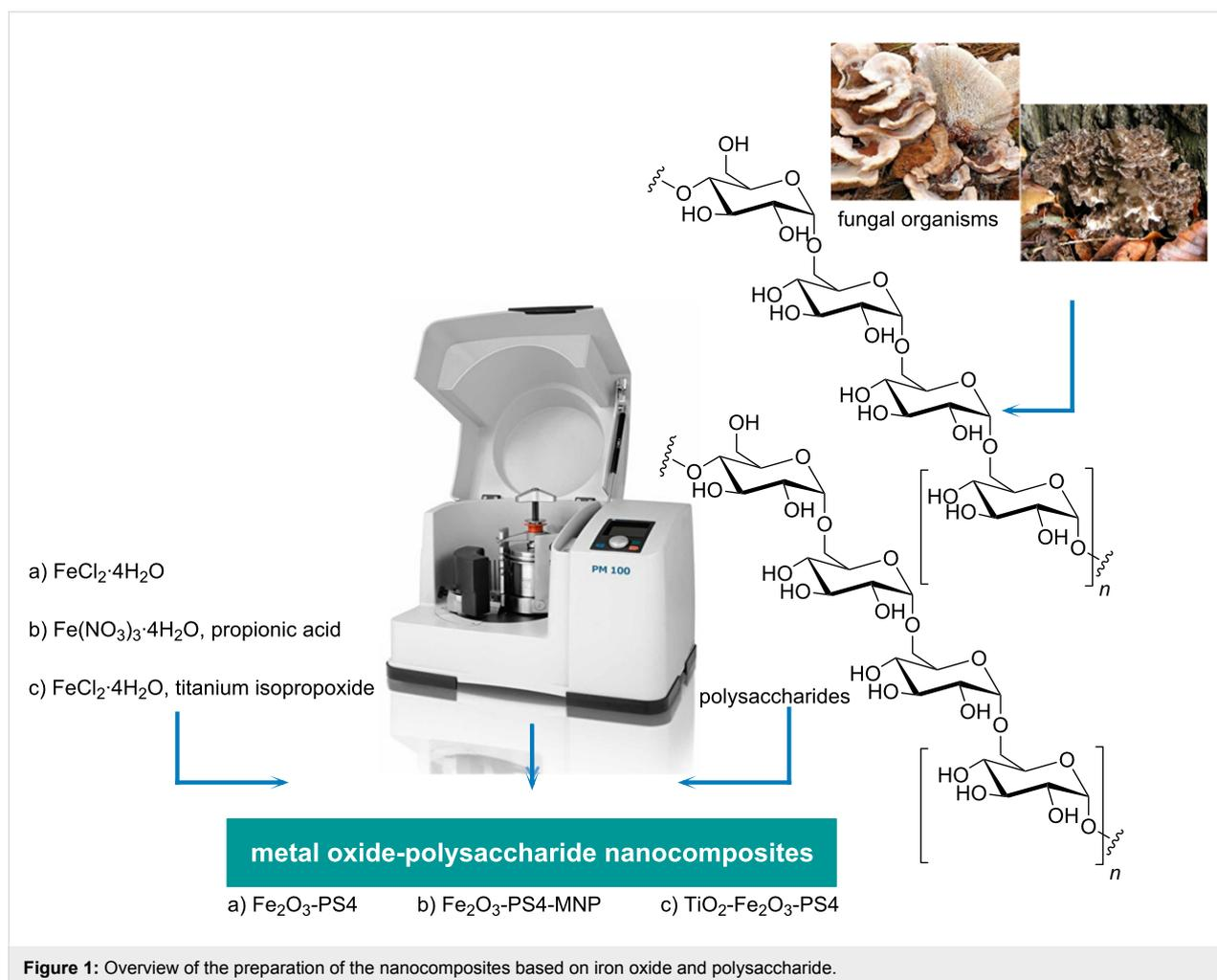
**Figure 1:** Overview of the preparation of the nanocomposites based on iron oxide and polysaccharide.
