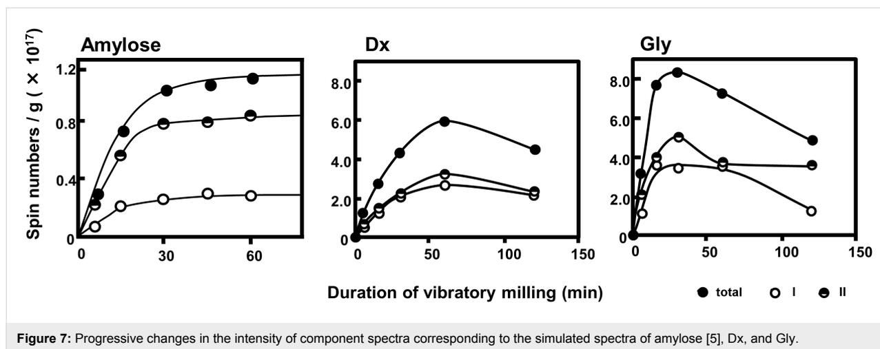
**Figure 7:** Progressive changes in the intensity of component spectra corresponding to the simulated spectra of amylose [5], Dx, and Gly.
