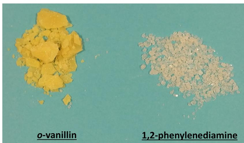
**Figure 2:** *o*-Vanillin in its flake form and 1,2-phenylenediamine in its bead form.
