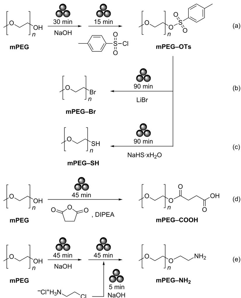
**Scheme 1:** Developed syntheses for accessing by mechanochemistry: (a) mPEG-OTs, (b) mPEG-Br, (c) mPEG-SH, (d) mPEG-COOH, and (e) mPEG<sub>x</sub>-NH<sub>2</sub>. mPEG of  $M_n = 750$  and  $2000$  Da were investigated as precursors. All milling reactions were performed at an operating frequency of 30 Hz.
