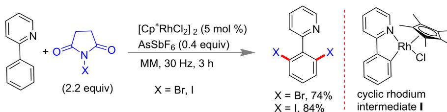
**Scheme 52:** Mechanochemical Rh-catalyzed  $\text{C}_{\text{sp}^2}$ -X bond formation [184].
