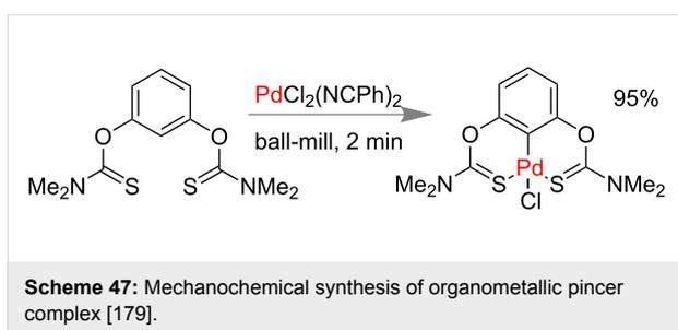
**Scheme 47:** Mechanochemical synthesis of organometallic pincer complex [179].
