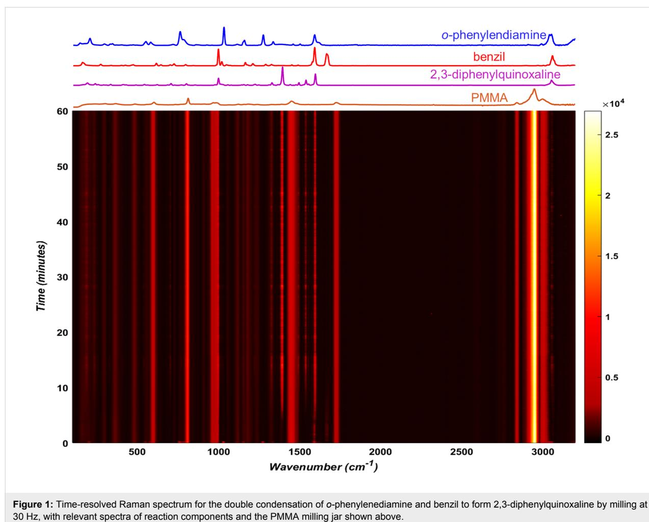
**Figure 1:** Time-resolved Raman spectrum for the double condensation of *o*-phenylenediamine and benzil to form 2,3-diphenylquinoxaline by milling at 30 Hz, with relevant spectra of reaction components and the PMMA milling jar shown above.
