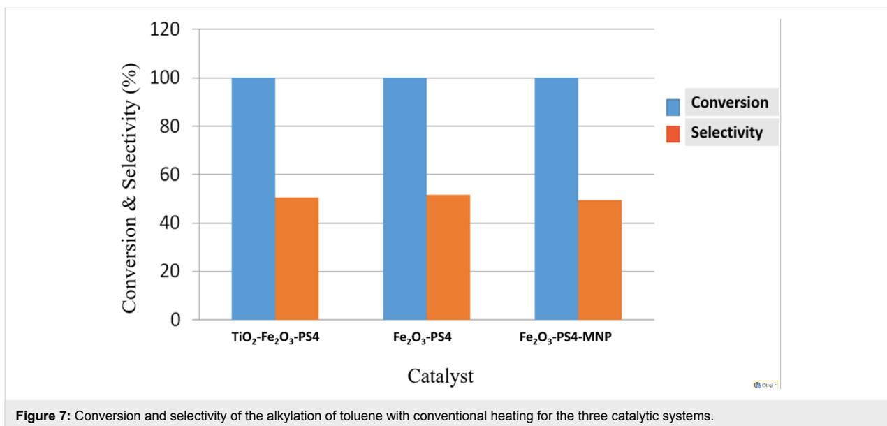
**Figure 7:** Conversion and selectivity of the alkylation of toluene with conventional heating for the three catalytic systems.
