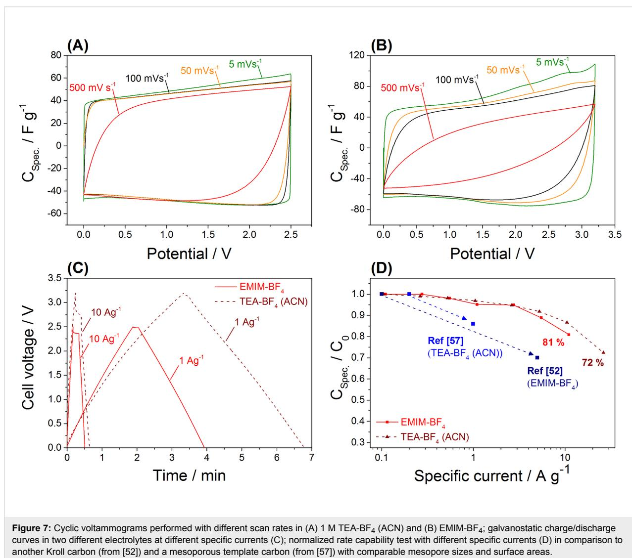
**Figure 7:** Cyclic voltammograms performed with different scan rates in (A) 1 M TEA-BF<sub>4</sub> (ACN) and (B) EMIM-BF<sub>4</sub>; galvanostatic charge/discharge curves in two different electrolytes at different specific currents (C); normalized rate capability test with different specific currents (D) in comparison to another Kroll carbon (from [52]) and a mesoporous template carbon (from [57]) with comparable mesopore sizes and surface areas.
