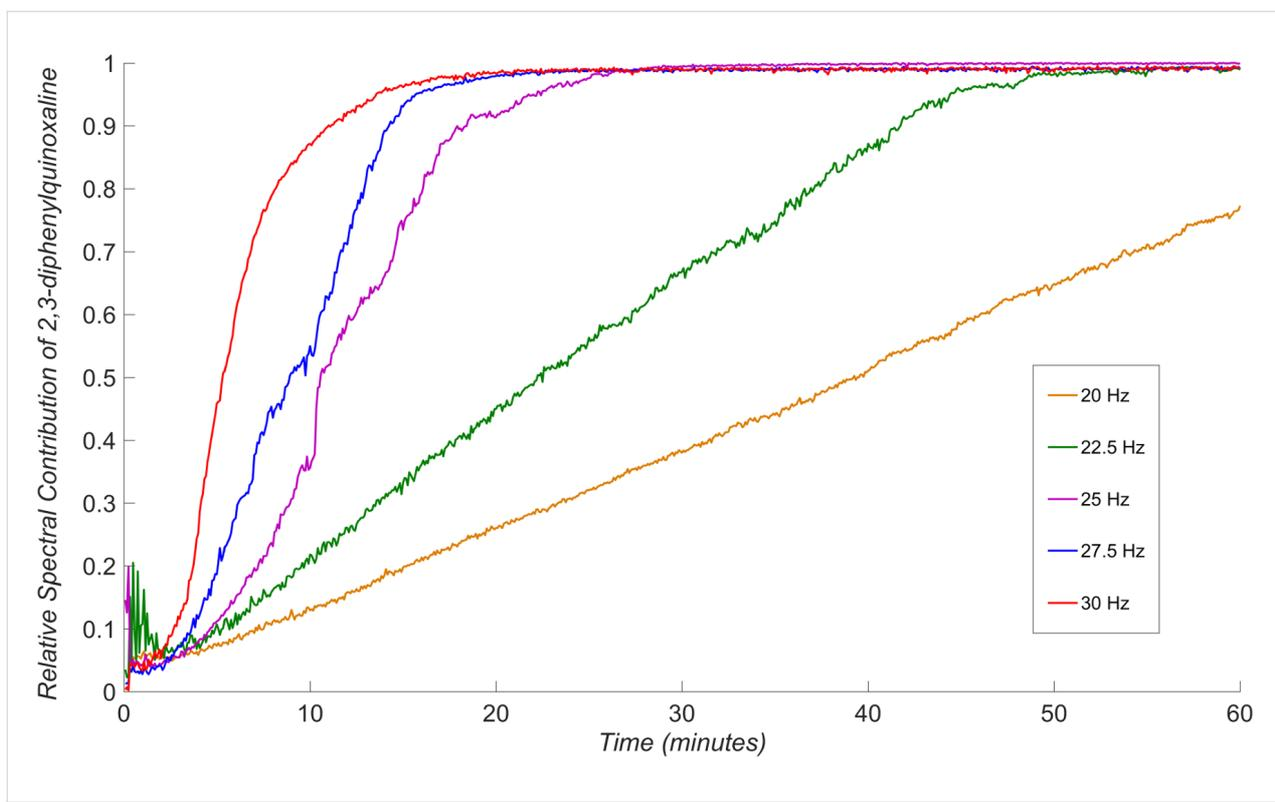
**Figure 4:** The effect of milling frequency on the milling condensation of benzil and *o*-phenylenediamine to form 2,3-diphenylquinoxaline, with data for each milling frequency averaged from a set of triplicate measurements. Variation close to the onset of milling may be due to poor initial homogeneity of the sample.
