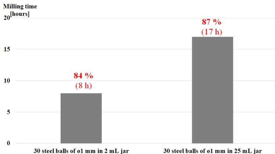
**Figure 1:** Effect of jar size on the reaction time using an equal number (30) of steel balls ( $\varnothing$  1 mm) for the Ts  $\rightarrow$  N<sub>3</sub> exchange reaction in glass vials at 550 min<sup>-1</sup> sun wheel speed.
