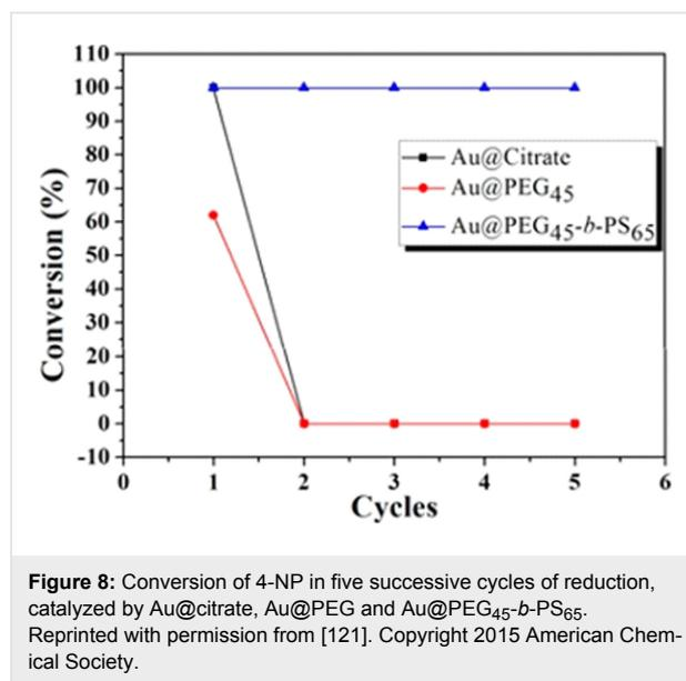
Superior catalytic activity of Au@PEG-*b*-PS was observed in the reduction reaction of 4-nitrophenol to 4-aminophenol. The catalytic activity increased with the decrease in the chain length of the PS block. In addition, the high stability imparted by the PS layer endowed Au@PEG-*b*-PS with good reusability in catalysis without the loss of catalytic activity, and prevented from electrolyte-induced aggregation, making the system very attractive as nanoreactor.
