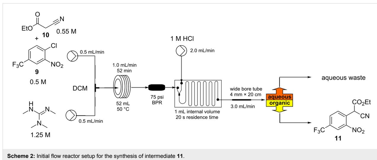
using a third flow stream of hydrochloric acid (1 M) blended via a dedicated mixer chip before the combined mixture was phase separated.
