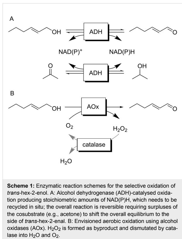
Therefore, we concentrated on alcohol oxidase-catalysed reaction schemes (Scheme 1B). Oxidases utilise O<sub>2</sub> as terminal electron acceptor for the oxidation reaction yielding H<sub>2</sub>O<sub>2</sub> as sole byproduct. The latter can be disproportionated easily by using catalase (Scheme 1B). Furthermore, O<sub>2</sub> reduction adds sufficient thermodynamic driving force to the reaction to make it essentially irreversible.
