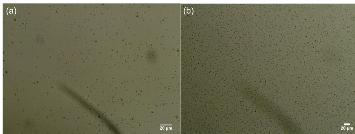
**Figure 3:** Optical microscope images of fresh aqueous dispersions, 0.05 wt %, of (a)  $\text{Ce}_{0.495}\text{Sn}_{0.495}\text{Pd}_{0.01}\text{O}_{2-\delta}$  and (b)  $\text{Ce}_{0.20}\text{Sn}_{0.79}\text{Pd}_{0.01}\text{O}_{2-\delta}$  particles.
