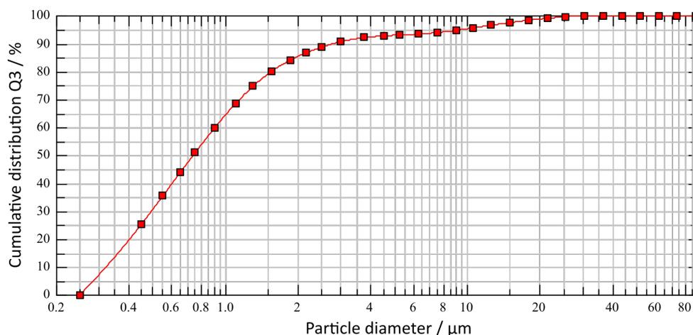
**Figure 2:** Particle size distribution of  $Ce_{0.495}Sn_{0.495}Pd_{0.01}O_{2-\delta}$  after size reduction via milling and separation via sedimentation in water.
