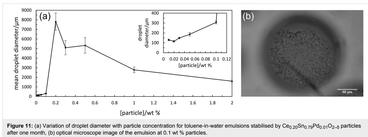
**Figure 11:** (a) Variation of droplet diameter with particle concentration for toluene-in-water emulsions stabilised by  $\text{Ce}_{0.20}\text{Sn}_{0.79}\text{Pd}_{0.01}\text{O}_{2-\delta}$  particles after one month, (b) optical microscope image of the emulsion at 0.1 wt % particles.
