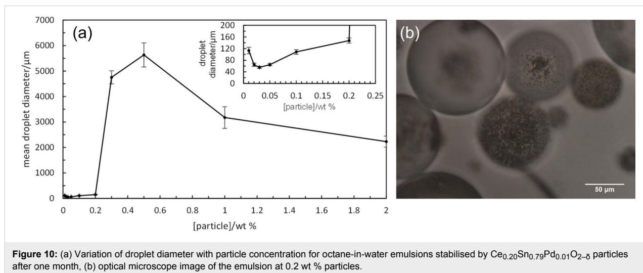
**Figure 10:** (a) Variation of droplet diameter with particle concentration for octane-in-water emulsions stabilised by  $\text{Ce}_{0.20}\text{Sn}_{0.79}\text{Pd}_{0.01}\text{O}_{2-\delta}$  particles after one month, (b) optical microscope image of the emulsion at 0.2 wt % particles.
