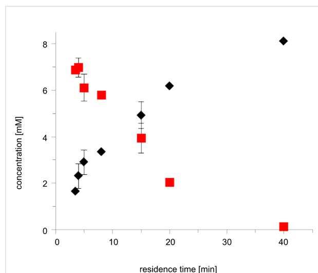
**Figure 2:** The influence of the residence time on the conversion of *trans*-hex-2-enol (red squares) to *trans*-2-hexenal (black diamonds) in a flow reactor. Conditions: 3 mL flow reactor, 50 mM  $\text{KP}_i$  buffer (pH 7, 30 °C),  $[\text{trans-hex-2-enol}]_0 = 10 \text{ mM}$ ,  $[\text{PeAAOx}] = 0.25 \text{ }\mu\text{M}$ , [catalase] =  $600 \text{ U mL}^{-1}$ .
