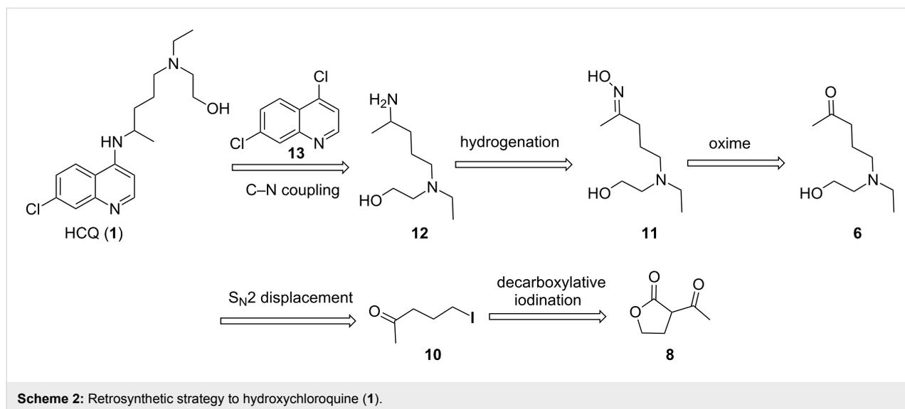
proaches are effective, they are significantly more costly than using simple heterogeneous reduction with H<sub>2</sub>/Raney-nickel. Therefore, we explored an alternate strategy: simple conversion of the ketone group of **6** to oxime **11**, followed by reduction to give 5-(ethyl(2-hydroxyethyl)amino)-2-aminopentane (**12**). We have found H<sub>2</sub>/Raney-nickel efficiently reduces **11** to **12** with THF as the solvent in a continuous stirred tank reactor (CSTR).
