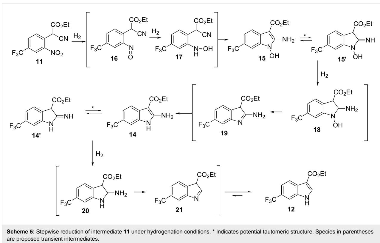
**Scheme 5:** Stepwise reduction of intermediate **11** under hydrogenation conditions. \* Indicates potential tautomeric structure. Species in parentheses are proposed transient intermediates.
