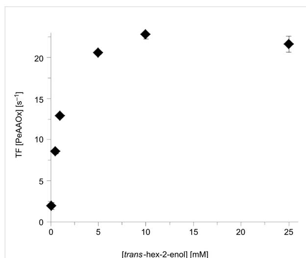
**Figure 1:** Michaelis–Menten kinetics of the *PeAAOx*-catalysed oxidation of *trans*-hex-2-enol. Conditions: 50 mM  $\text{KP}_i$  buffer (pH 7, 30 °C),  $[\text{trans-hex-2-enol}]_0 = 3 \text{ mM}$ ,  $[\text{PeAAOx}] = 0.044 \text{ }\mu\text{M}$ , [horseradish peroxidase] =  $500 \text{ U mL}^{-1}$ , [ABTS] = 2 mM.
