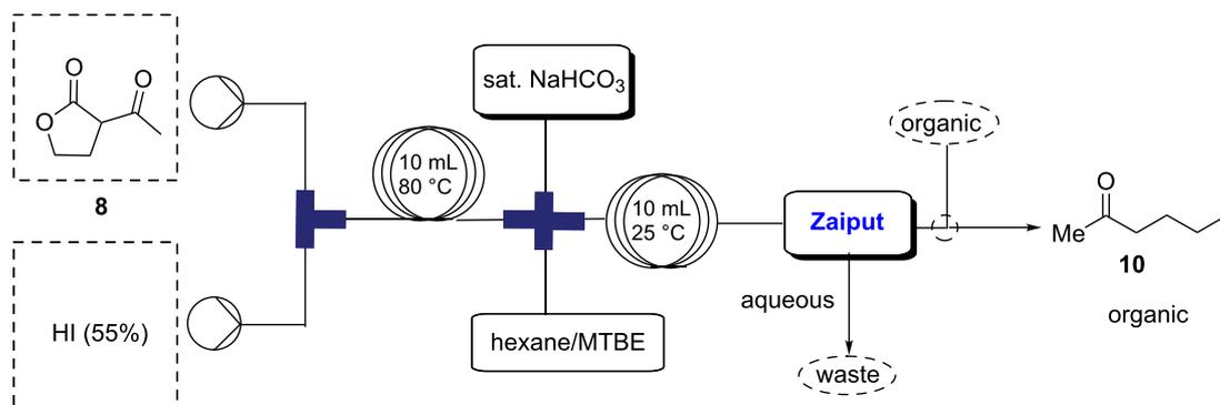
**Scheme 3:** Schematic representation for continuous in-line extraction of **10**.
