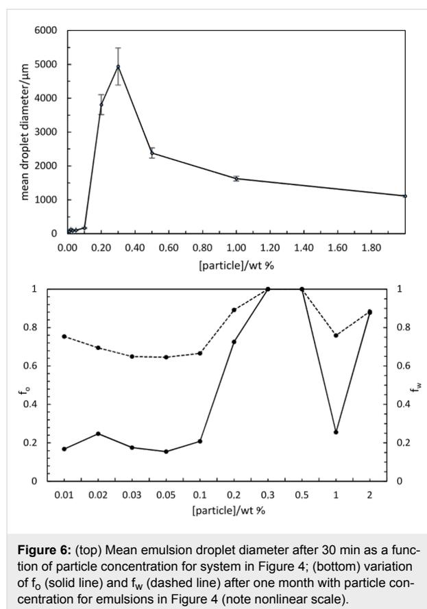
**Figure 6:** (top) Mean emulsion droplet diameter after 30 min as a function of particle concentration for system in Figure 4; (bottom) variation of  $f_o$  (solid line) and  $f_w$  (dashed line) after one month with particle concentration for emulsions in Figure 4 (note nonlinear scale).
