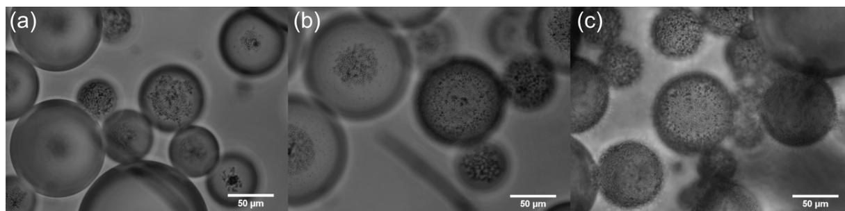
**Figure 5:** Optical microscopy images of cyclohexane-in-water emulsions of Figure 4 after one month for particle concentrations of (a) 0.02 wt %, (b) 0.05 wt % and (c) 0.10 wt %.
