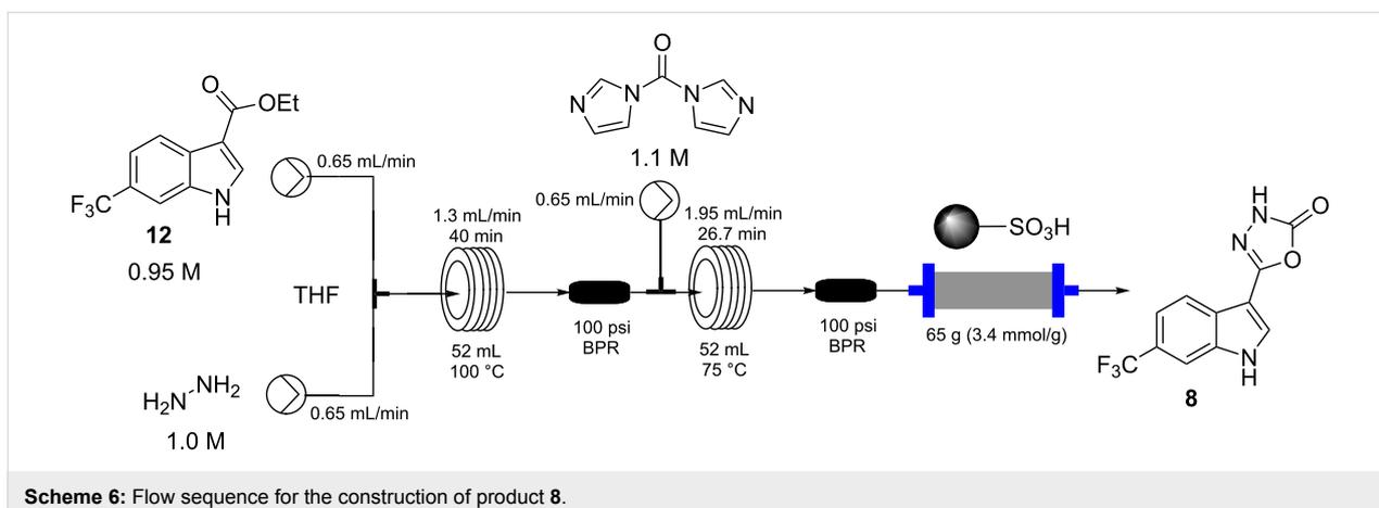
through a scavenging cartridge of QP-SA (a sulfonic acid functionalised polymer). The product **8** was obtained after solvent evaporation as a yellow solid (94%) but required recrystallization from DCM to give a white amorphous powder of high purity in 82% yield.
