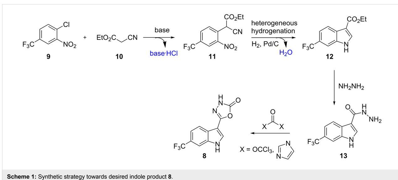
(base·HCl, H<sub>2</sub>O) and uses industrially favourable hydrogenation protocols in the key cyclisation step.
