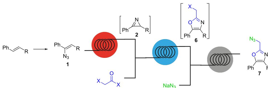
**Scheme 3:** Integrated continuous-flow synthesis of 2-(azidomethyl)oxazoles **7**.
