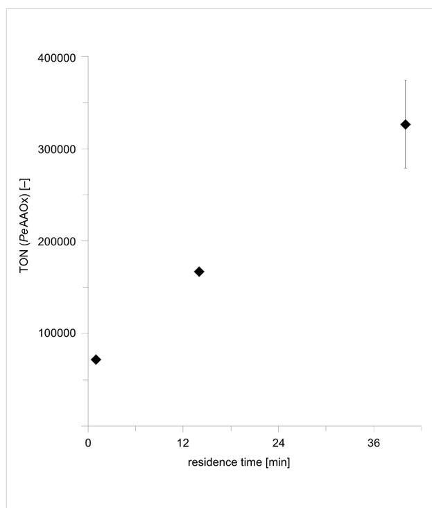
**Figure 3:** Increasing the *PeAAOx* turnover numbers (TN) by increasing the residence time. Conditions: 6 mL flow reactor, 50 mM KP<sub>i</sub> buffer (pH 7, 30 °C), [*trans*-hex-2-enol]<sub>0</sub> = 40 mM, [*PeAAOx*] = 0.02 μM, [catalase] = 600 U mL<sup>-1</sup>. The TN value was calculated based on the GC yield of every run. The TN was obtained by dividing the product concentration (as determined chromatographically) by the biocatalyst concentration.
