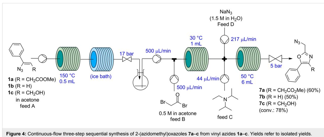
ploying a 0.25 M solution of substrate **1c**. Under diluted conditions the reaction mixture remained fully homogeneous but no full conversion from bromo oxazole **6c** to azido oxazole **7c** was achieved (78%), which prevented the formation of the final product in a pure form.
