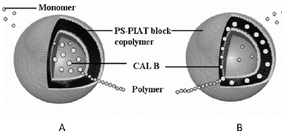
**Figure 5:** Schematic representation of enzymatic polymerization in polymersomes. (A) CALB in the aqueous compartment (B) CALB embedded in the bilayer. Reprinted with permission from [21]. Copyright 2007 American Chemical Society.
