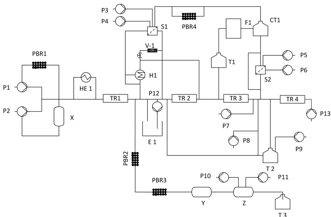
**Figure 2:** Schematic representation of a unified platform for the flow synthesis (P1–P14 pumps, PBR packed bed reactor, HE1 heat exchanger, H1 heater, S1 and S2 separator, E1 extractor, TR1–TR4 tubular reactor, CH charcoal, CT1 crystallization tank, T1–T3 tanks, F1 filtration).
