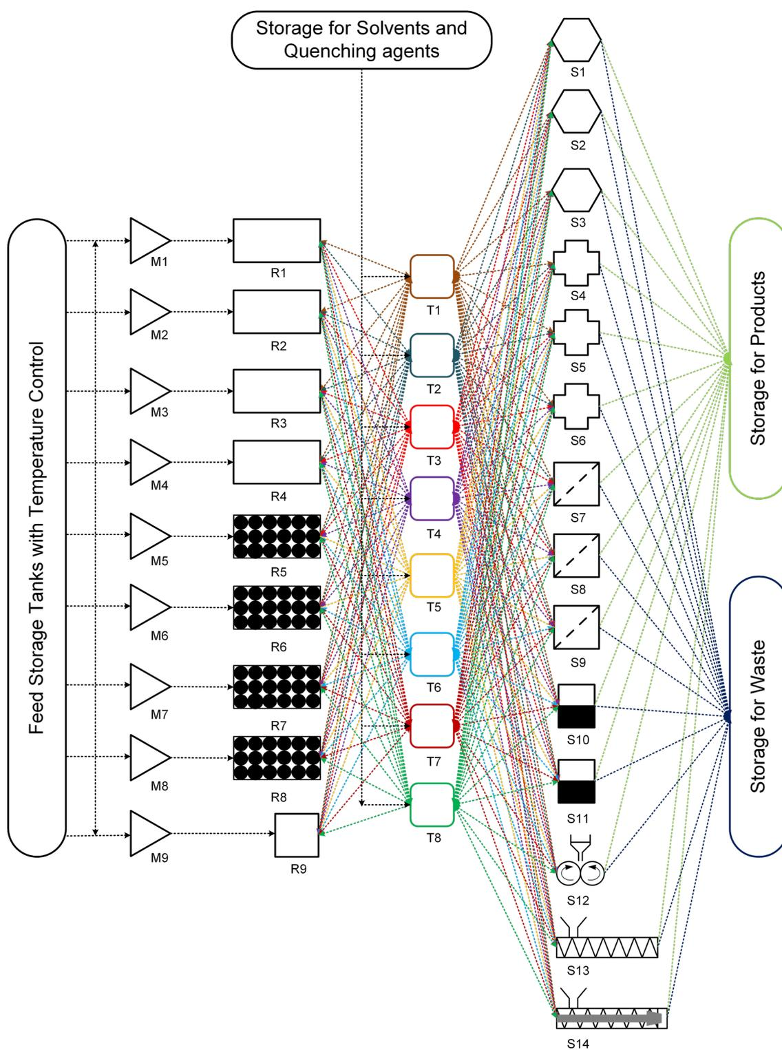
**Figure 5:** Approach 3 for a unified platform for multistep synthesis. M1–M9 = mixers, R1–R4 = tubular reactors, R5–R8 = packed bed reactor, R9 = stirred tank reactor, T1–T8 = Intermediate storage tanks, S1–S3 = adsorption columns, S4–S6 = extraction columns/gravity-based separator, S7–S9 = membrane separator/Filter, S10–S11 = evaporator, S12 = rotary drum dryer, S13 = vacuum screw dryer, S14 = extruder.
