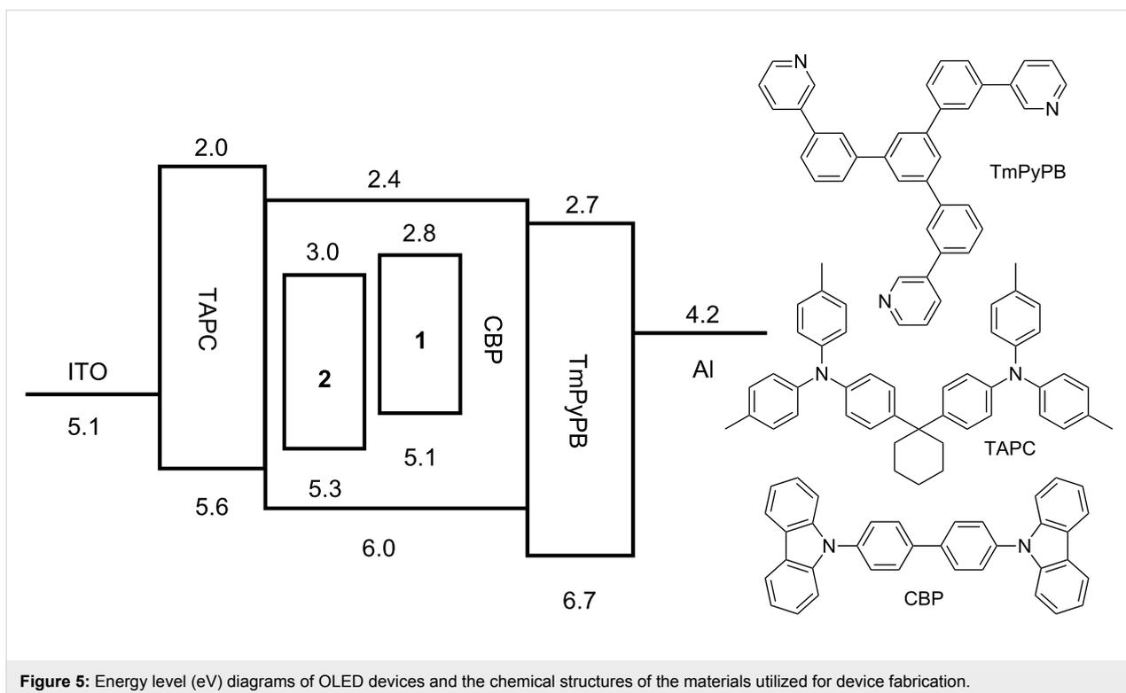
**Figure 5:** Energy level (eV) diagrams of OLED devices and the chemical structures of the materials utilized for device fabrication.
