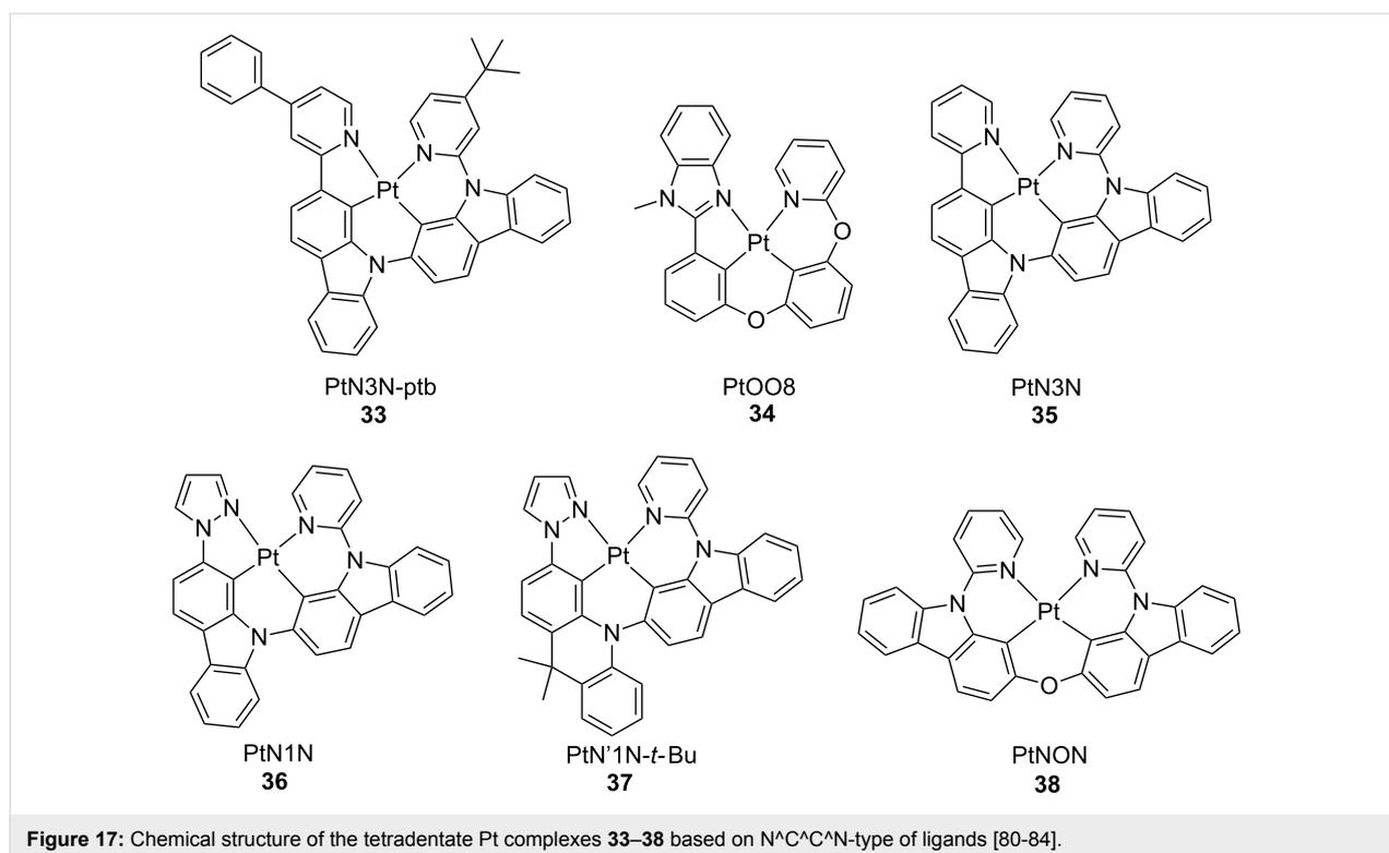
order to shift exciton formation zone deeper into the emissive layer (device configuration: ITO/HATCN/NPD/TrisPCz/compound **35** 20 wt %:CBP/compound **35** 6 wt %:CBP/BAIq/BPyTP/LiF/Al). Such devices displayed EL spectra that was slightly broader than PL emission due to the relatively high dopant concentration with an estimated  $LT_{97} = 2057$  h and  $EQE = 15.3\%$  at  $1000 \text{ cd m}^{-2}$ .
