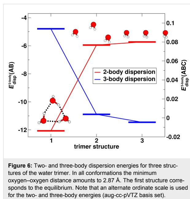
**Figure 6:** Two- and three-body dispersion energies for three structures of the water trimer. In all conformations the minimum oxygen–oxygen distance amounts to 2.87 Å. The first structure corresponds to the equilibrium. Note that an alternate ordinate scale is used for the two- and three-body energies (aug-cc-pVTZ basis set).
