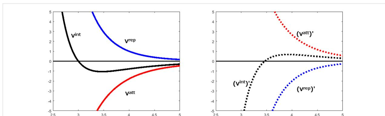
**Figure 1:** Left: The graphs of an interaction potential  $V^{\text{int}}$  composed of an attractive component  $V^{\text{att}}$  and a repulsive component  $V^{\text{rep}}$ . Right: The corresponding slope functions.
