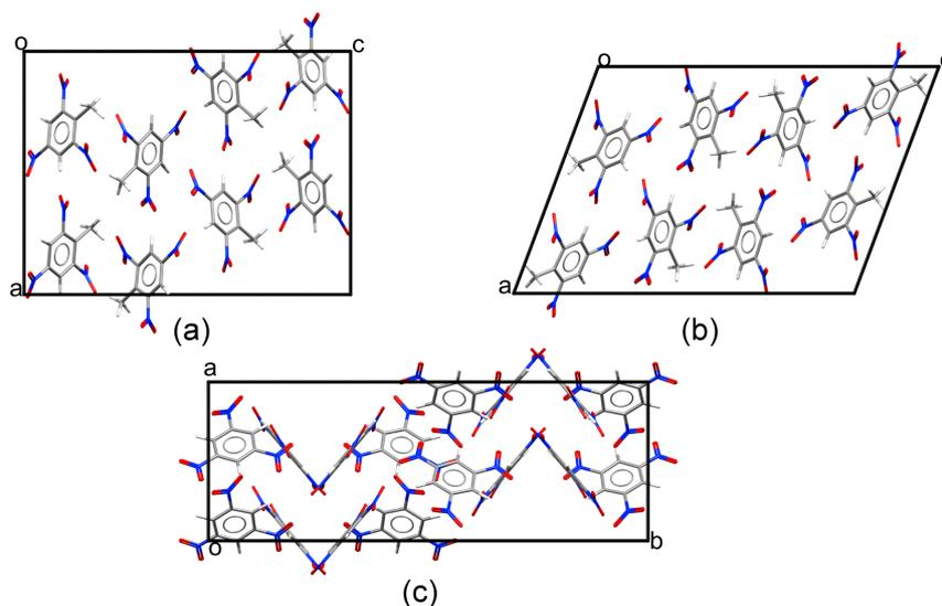
**Figure 1:** Structures of: (a) orthorhombic TNT, (b) monoclinic TNT, (c) orthorhombic TNB. For each structure, the direction of two of the three lattice vectors ( $a$ ,  $b$ ,  $c$ ) is shown in the figure and the third one points inwards at the origin ( $o$ ).
