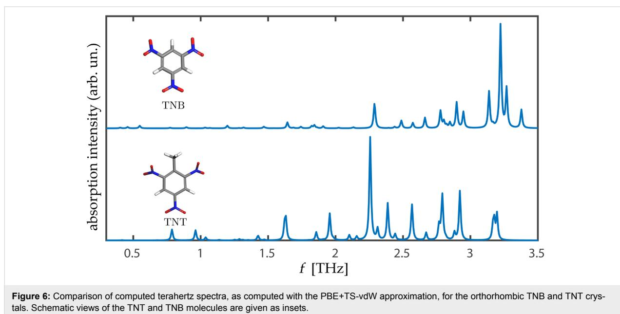
**Figure 6:** Comparison of computed terahertz spectra, as computed with the PBE+TS-vdW approximation, for the orthorhombic TNB and TNT crystals. Schematic views of the TNT and TNB molecules are given as insets.
