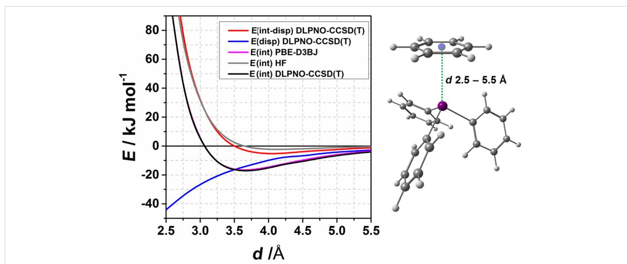
**Figure 9:** Computed interaction potentials of the distance scan for the idealized  $\text{BiPh}_3$ –benzene complex.  $E(\text{int})$  denotes the interaction energy obtained at the particular level of theory,  $E(\text{disp})$  denotes the dispersion energy,  $E(\text{int-disp})$  – the interaction energy without the dispersion contribution.
