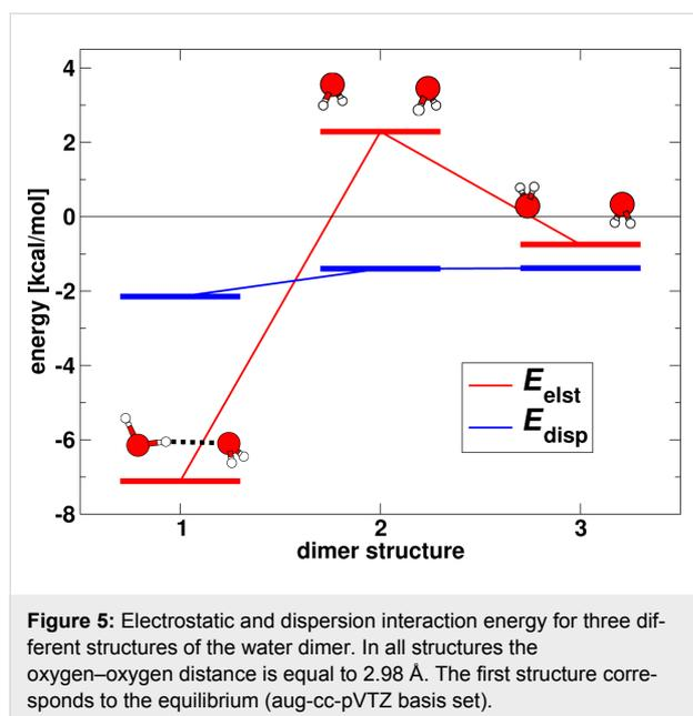
**Figure 5:** Electrostatic and dispersion interaction energy for three different structures of the water dimer. In all structures the oxygen–oxygen distance is equal to 2.98 Å. The first structure corresponds to the equilibrium (aug-cc-pVTZ basis set).
