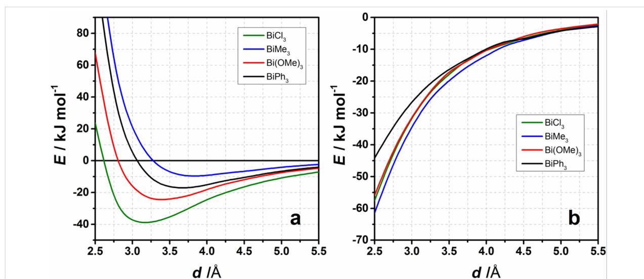
**Figure 10:** a) The  $\text{BiPh}_3$  potential energy curve for idealized interaction structures compared to the interaction energy curves for the series of compounds  $\text{BiR}_3 \cdots \text{C}_6\text{H}_6$  with  $\text{R} = \text{Me}, \text{OMe}, \text{Cl}$  obtained at the DLPNO-CCSD(T) level of theory. b) Dispersion energy contributions according to LED (DLPNO-CCSD(T)) for the distance scans shown in Figure 9.
