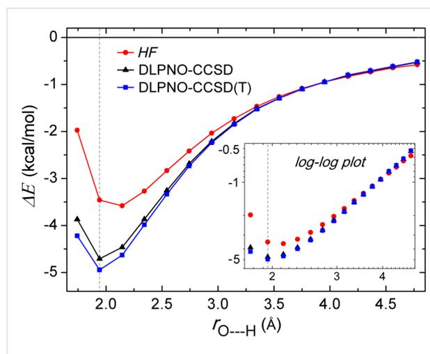
**Figure 3:** Dissociation curve of Conf1 of water dimer as a function of the H-bond distance. Its nearly linear relation in the log–log scale for the long range is shown as insert on the graph. The black dotted vertical line at 1.943 Å corresponds to the equilibrium  $r_e(\text{O}\cdots\text{H})$  distance.
