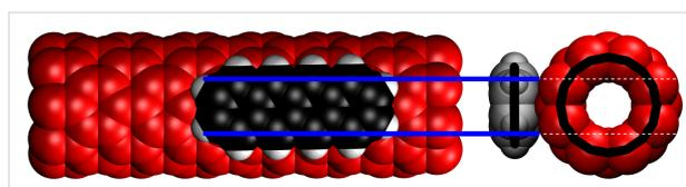
**Figure 6:** The contact zone of an (8,0)-CNT/tetracene complex. The bold black lines in the traverse section represent the positions of the nuclei. Reprinted with permission from [44], copyright 2017 Elsevier.
