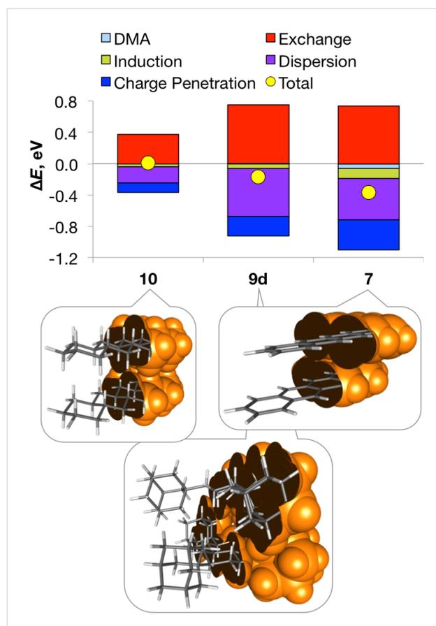
**Figure 4:** Decomposition of the SAPT0/jun-cc-pVDZ energy difference between the optimized and frozen dimers (*i.e.*,  $\Delta E = E_{\text{total or component}}[\text{optimized}] - E_{\text{total or component}}[\text{frozen}]$ ) for the representative cores from classes (II) and (III), as well as the M06-2X/def2-SVP geometries of their optimized dimers (clipped van der Waals surfaces are shown in orange).
