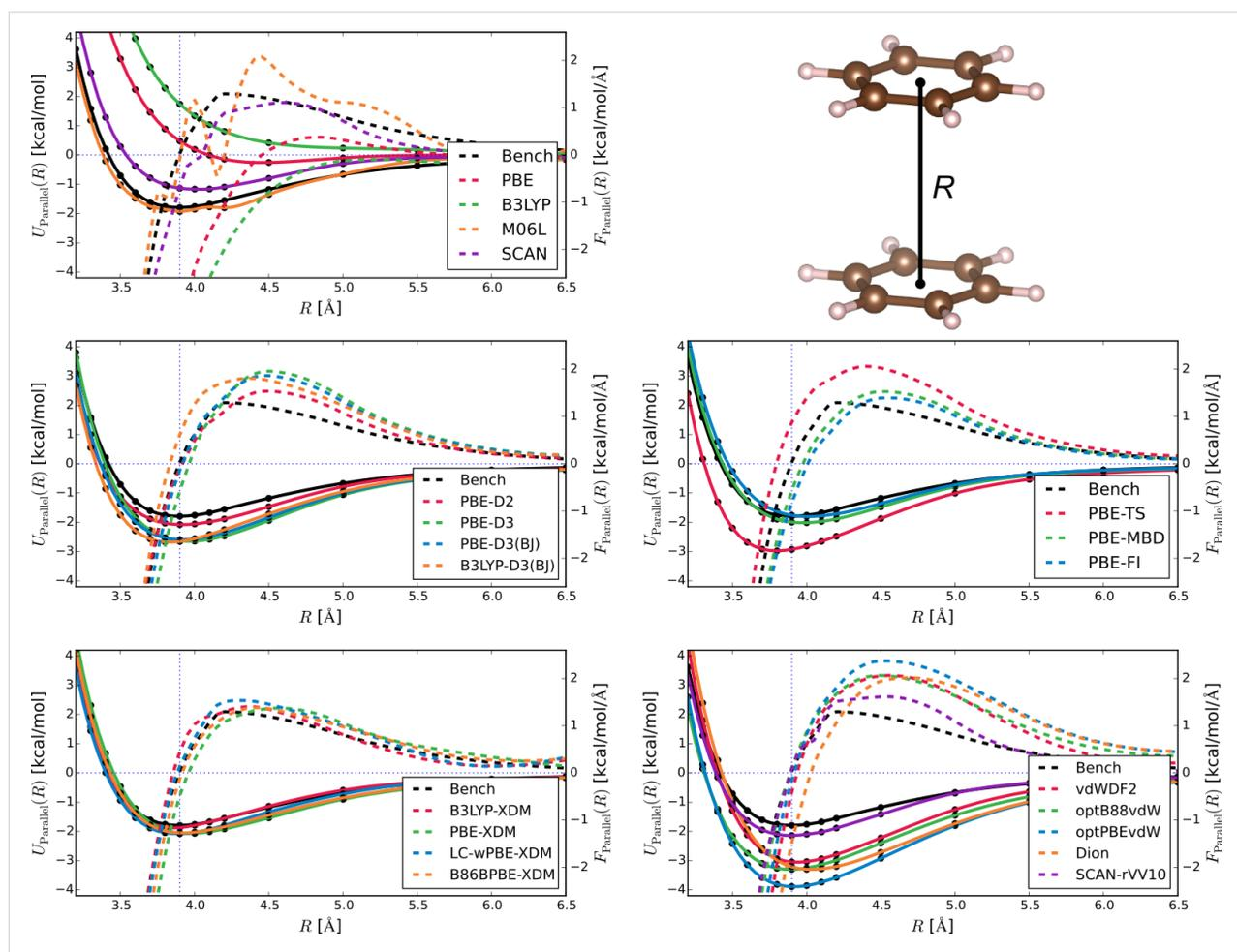
**Figure 1:** Interaction energies (solid lines) and forces (dashed lines) for the parallel configuration of the benzene dimer. Each panel groups a different family of computational approach. The top row (from left to right) shows GGAs and meta-GGAs without dispersion corrections, and the dimer geometry. The second row reports Grimme-D variants (l) and TS/MBD variants (r). The bottom row shows XDM on different DFAs (l), and vdW-DFAs (r). The benchmark data is always shown in black.
