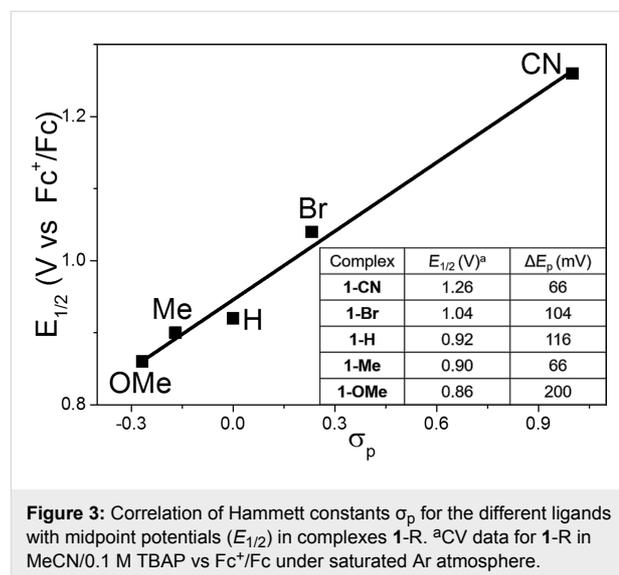
**Figure 3:** Correlation of Hammett constants  $\sigma_p$  for the different ligands with midpoint potentials ( $E_{1/2}$ ) in complexes **1**-R. <sup>a</sup>CV data for **1**-R in MeCN/0.1 M TBAP vs  $Fc^+/Fc$  under saturated Ar atmosphere.
