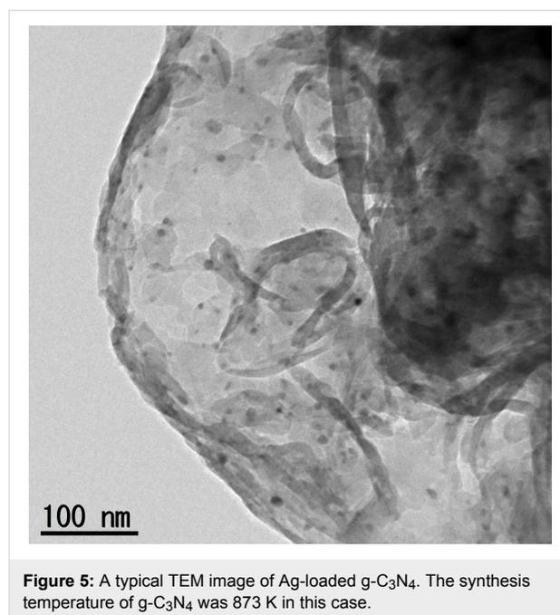
**Figure 5:** A typical TEM image of Ag-loaded g-C<sub>3</sub>N<sub>4</sub>. The synthesis temperature of g-C<sub>3</sub>N<sub>4</sub> was 873 K in this case.
