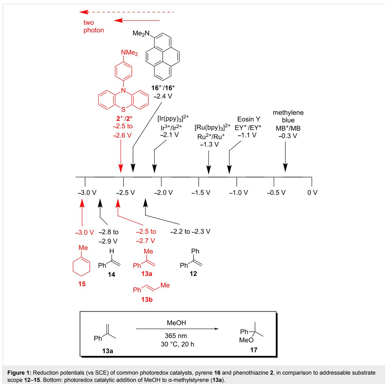
**Figure 1:** Reduction potentials (vs SCE) of common photoredox catalysts, pyrene **16** and phenothiazine **2**, in comparison to addressable substrate scope **12–15**. Bottom: photoredox catalytic addition of MeOH to  $\alpha$ -methylstyrene (**13a**).
