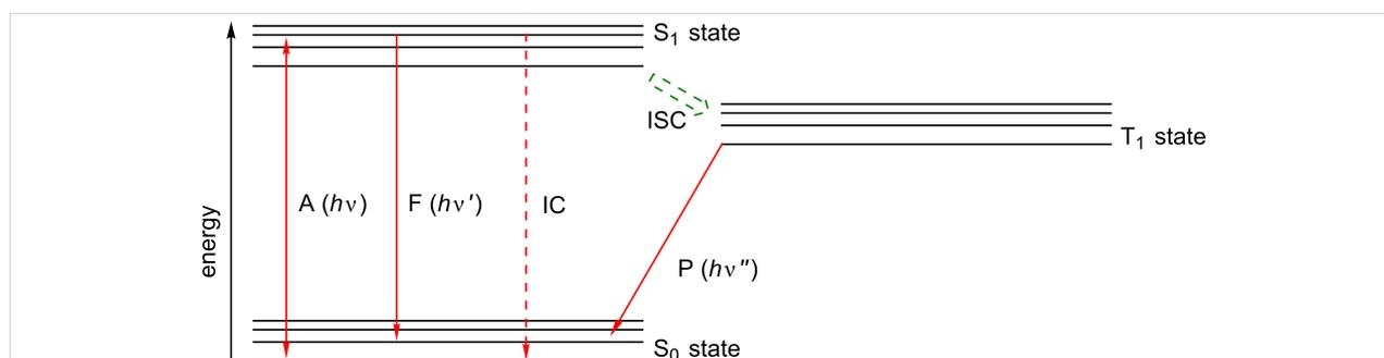
**Figure 1:** Depiction of the energy levels of a typical organic molecule and the photophysical processes it can undergo. A – absorption and emission, F – fluorescence, IC – internal conversion (non-radiative), ISC – intersystem crossing, P – phosphorescence.
