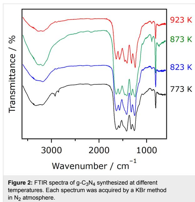
**Figure 2:** FTIR spectra of g-C<sub>3</sub>N<sub>4</sub> synthesized at different temperatures. Each spectrum was acquired by a KBr method in N<sub>2</sub> atmosphere.
