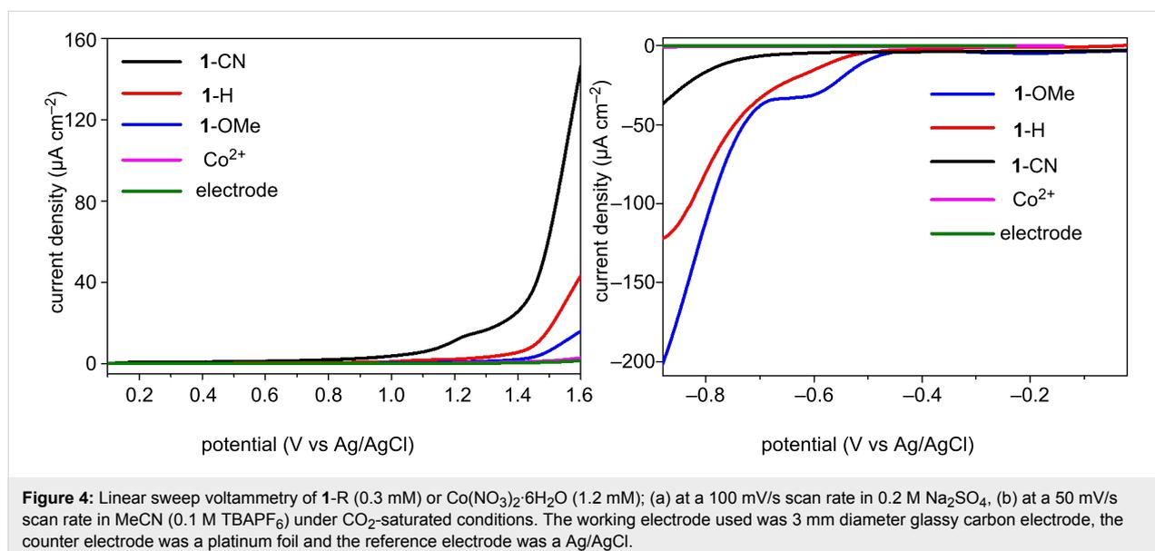
**Figure 4:** Linear sweep voltammetry of **1**-R (0.3 mM) or  $Co(NO_3)_2 \cdot 6H_2O$  (1.2 mM); (a) at a 100 mV/s scan rate in 0.2 M  $Na_2SO_4$ , (b) at a 50 mV/s scan rate in MeCN (0.1 M  $TBAPF_6$ ) under  $CO_2$ -saturated conditions. The working electrode used was 3 mm diameter glassy carbon electrode, the counter electrode was a platinum foil and the reference electrode was a Ag/AgCl.
