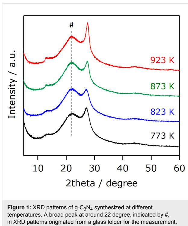
**Figure 1:** XRD patterns of g-C<sub>3</sub>N<sub>4</sub> synthesized at different temperatures. A broad peak at around 22 degree, indicated by #, in XRD patterns originated from a glass folder for the measurement.
