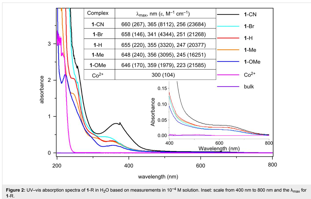
**Figure 2:** UV–vis absorption spectra of **1-R** in H<sub>2</sub>O based on measurements in 10<sup>-4</sup> M solution. Inset: scale from 400 nm to 800 nm and the  $\lambda_{\max}$  for **1-R**.
