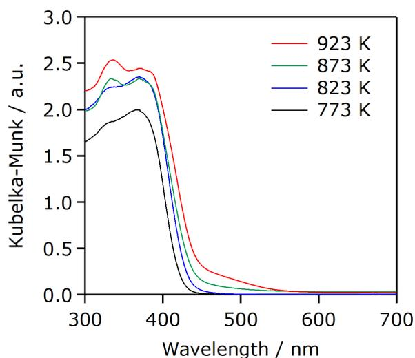
**Figure 4:** UV–visible diffuse reflectance spectra of g-C<sub>3</sub>N<sub>4</sub> synthesized at different temperatures.
