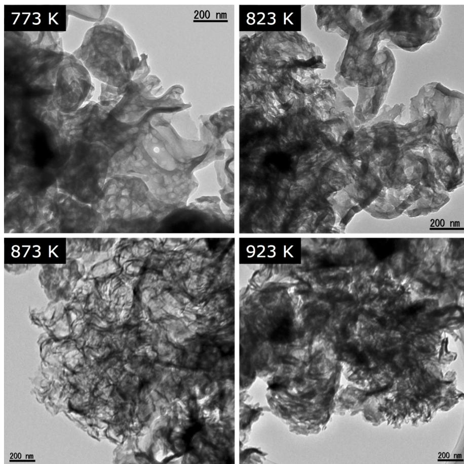
**Figure 3:** TEM images of g-C<sub>3</sub>N<sub>4</sub> synthesized at different temperatures.
