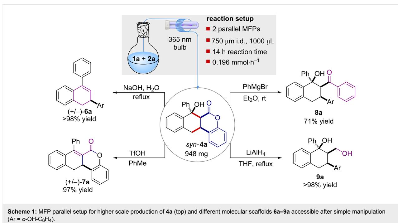
**Scheme 1:** MFP parallel setup for higher scale production of **4a** (top) and different molecular scaffolds **6a–9a** accessible after simple manipulation (Ar = *o*-OH-C<sub>6</sub>H<sub>4</sub>).
