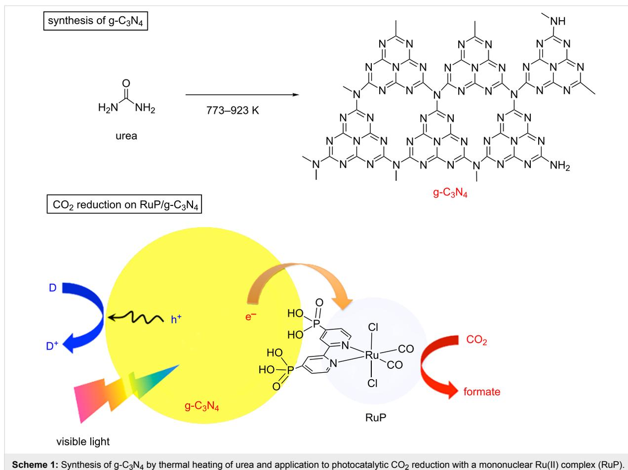
**Scheme 1:** Synthesis of  $g\text{-C}_3\text{N}_4$  by thermal heating of urea and application to photocatalytic CO<sub>2</sub> reduction with a mononuclear Ru(II) complex (RuP).
