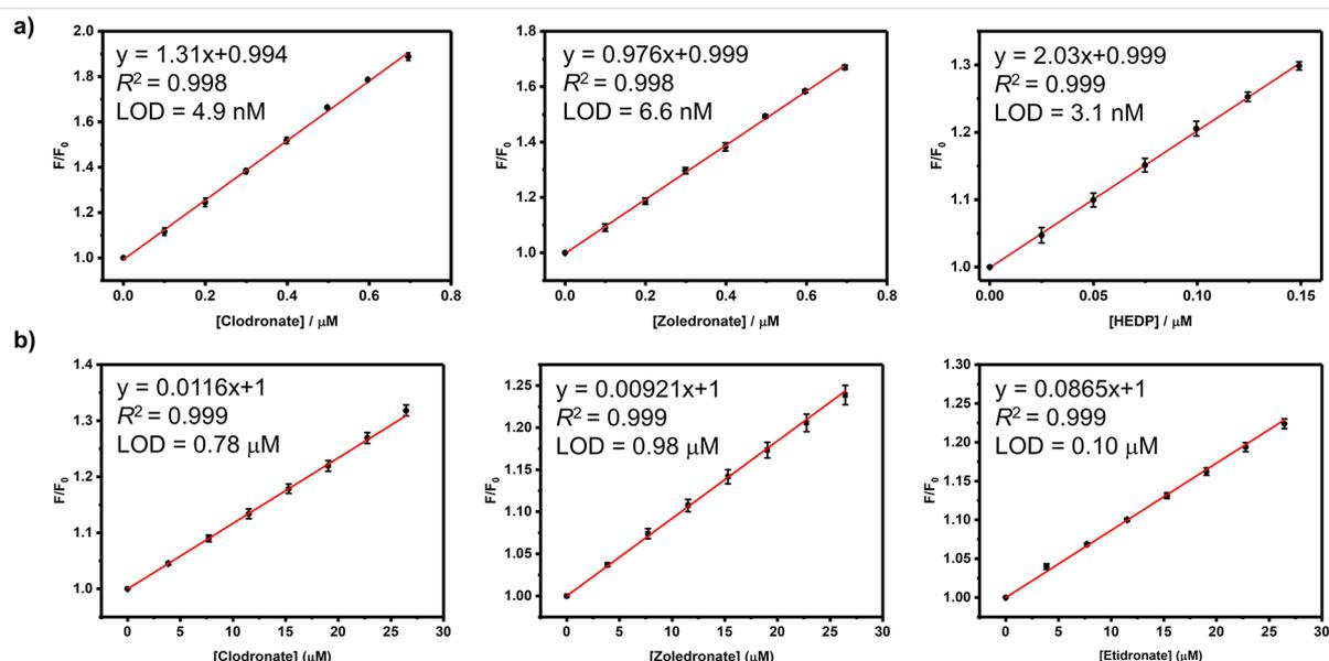
**Figure 2:** The set-up calibration lines of the fluorescence intensities for quantitatively determining the concentrations of clodronate, zoledronate and etidronate in (a) HEPES buffer (10 mM, pH 7.4) and (b) artificial urine at 25  $^{\circ}\text{C}$ . Error bars could not be shown if less than 0.005.
