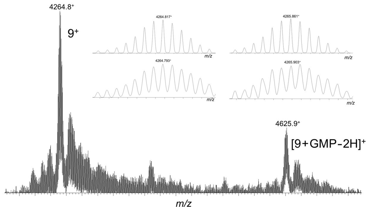
**Figure 6:** MALDI-MS analysis of a solution containing conjugate **9** and GMP after continuous light irradiation. In the inset, the experimental (bottom) and theoretical (top) isotope distributions are compared for both **9**<sup>+</sup> and [**9** + GMP - 2H]<sup>+</sup> ions.
