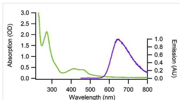
**Figure 3:** Absorption and emission spectra of Ru<sup>II</sup>-calix[4]arene-[c-(RGDfK)<sub>4</sub>] conjugate **9** in water.
