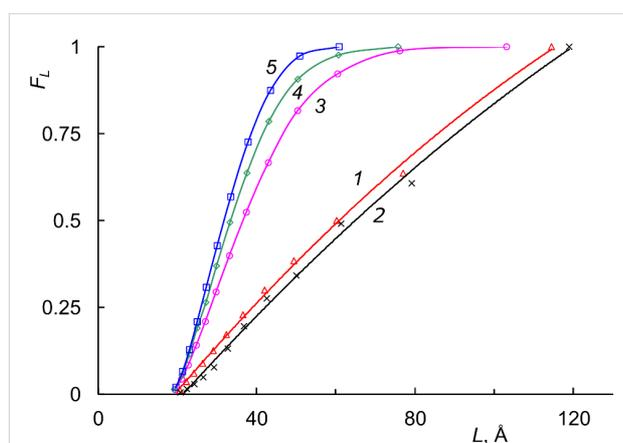
**Figure 8:** Integral distribution functions for the lamella thickness of crystallites in thermally fractionated (1) PCOE after Gr1 treatment, (2) PCOE/PNB blend, and NB–COE copolymers with different COE-block lengths, (3)  $L_{COE} = 22$ , (4)  $L_{COE} = 12$ , and (5)  $L_{COE} = 9.4$  [92]
