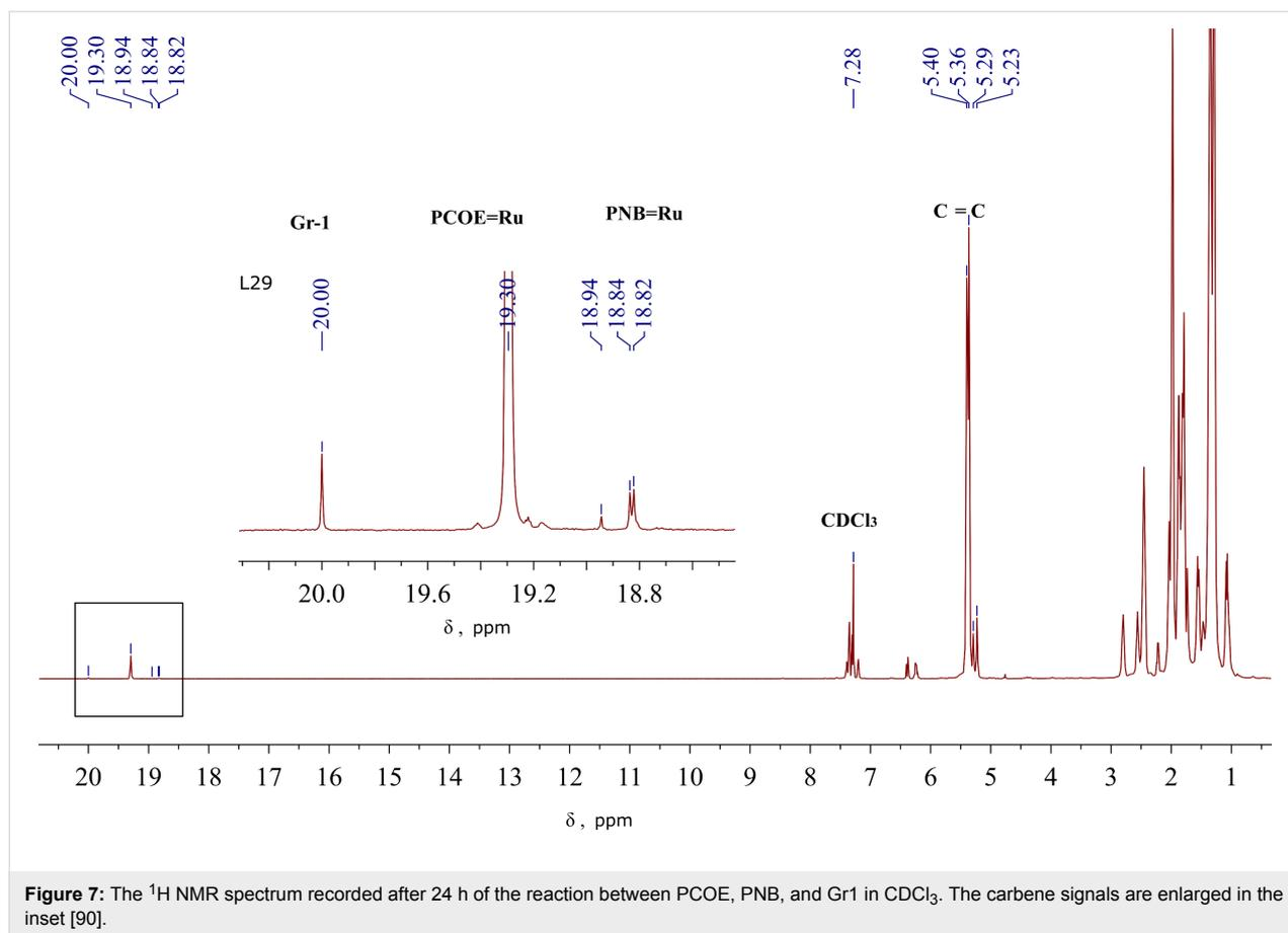
**Figure 7:** The  $^1\text{H}$  NMR spectrum recorded after 24 h of the reaction between PCOE, PNB, and Gr1 in  $\text{CDCl}_3$ . The carbene signals are enlarged in the inset [90].
