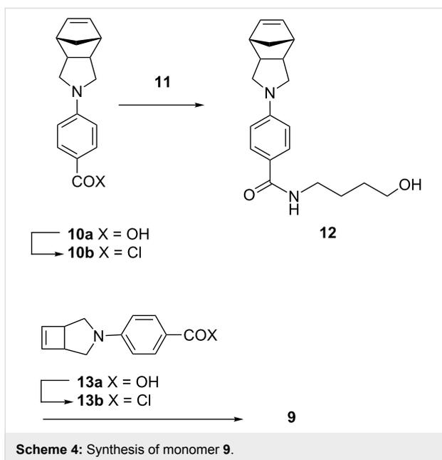
inary studies that only the cyclobutene moiety, but not norbornene in **9**, proceeds **6**-catalyzed ROMP under these conditions. The degree of polymerization of **14** was estimated to be 10 based on the  $^1\text{H}$  NMR integration of relevant peaks.
