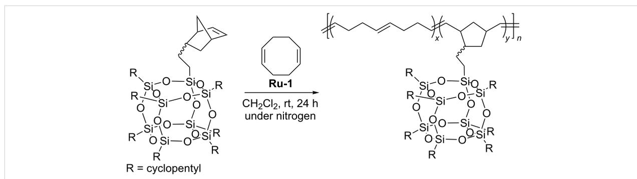
**Scheme 22:** ROMP of norbornenylethyl-POSS with 1,5-cyclooctadiene.
