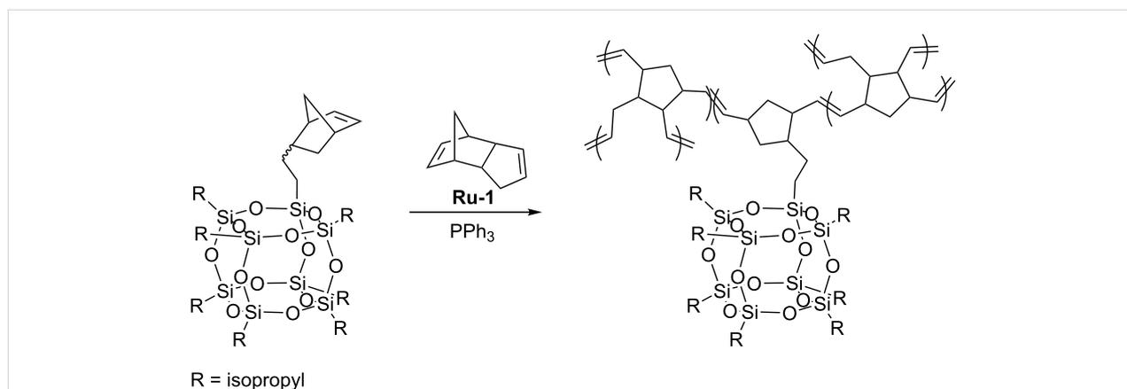
**Scheme 23:** Copolymerization of POSS-functionalized norbornene with DCPD.
