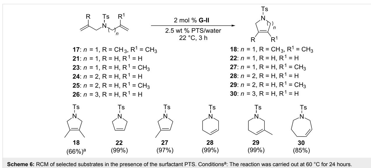
**Scheme 6:** RCM of selected substrates in the presence of the surfactant PTS. Conditions<sup>a</sup>: The reaction was carried out at 60 °C for 24 hours.
