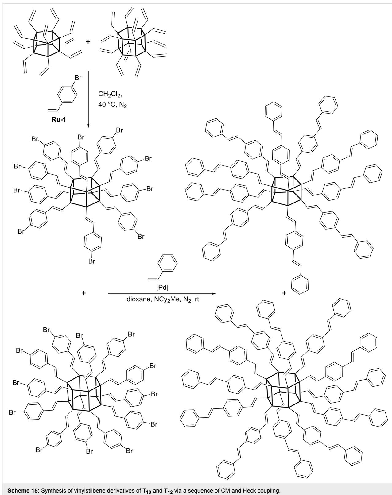
**Scheme 15:** Synthesis of vinylstilbene derivatives of **T**<sub>10</sub> and **T**<sub>12</sub> via a sequence of CM and Heck coupling.
