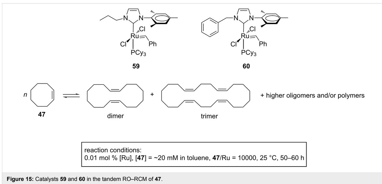
**Figure 15:** Catalysts **59** and **60** in the tandem RO-RCM of **47**.
