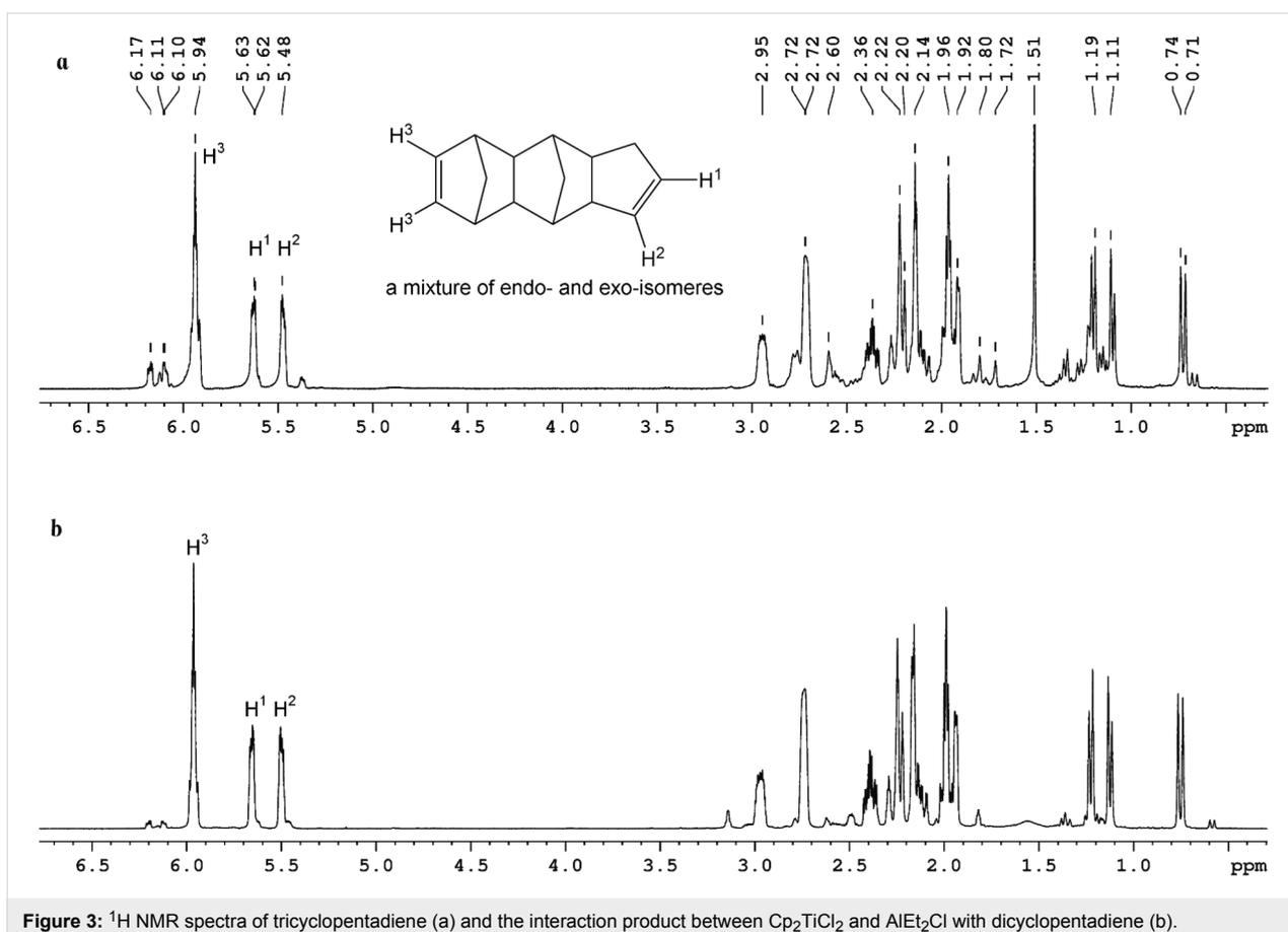
**Figure 3:**  $^1\text{H}$  NMR spectra of tricyclopentadiene (a) and the interaction product between  $\text{Cp}_2\text{TiCl}_2$  and  $\text{AlEt}_2\text{Cl}$  with dicyclopentadiene (b).
