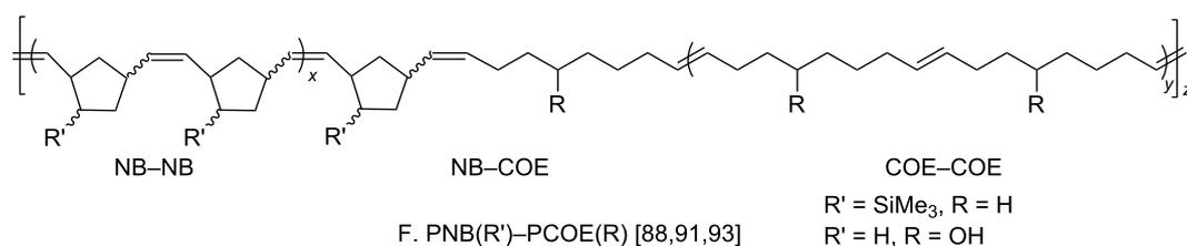
Figure 4: Multiblock copolymers synthesized by macromolecular cross metathesis.
