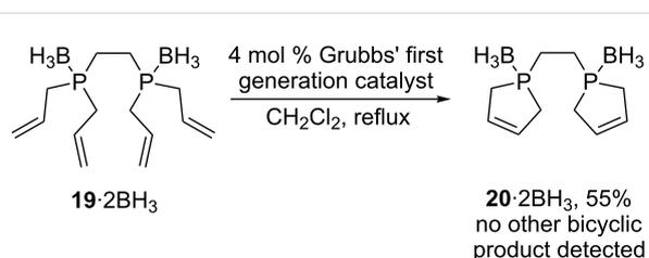
**Scheme 10:** Alkene metathesis of the tetraalkenyldiphosphine diborane **19**·2BH<sub>3</sub>.
