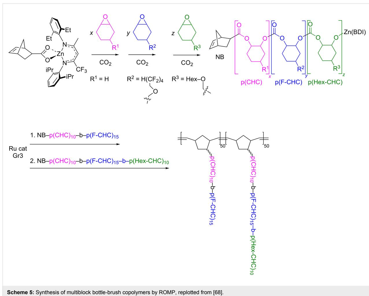
through” by ROMP of norbornene resulted in the synthesis of multiblock copolymer brushes. Changes in the synthetic stage sequence led to variable layer compositions.
