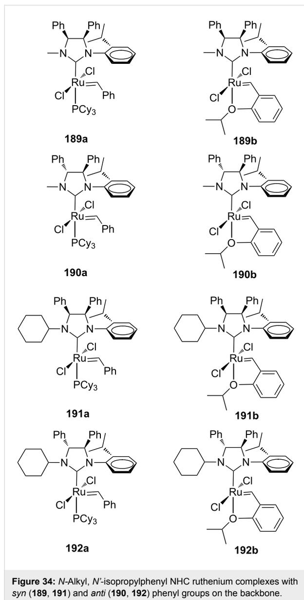
The effect of the NHC backbone configuration on the catalytic properties has been justified considering a more electron-donating nature of the *anti* ligand with respect to the *syn* ligand, as suggested by experimental and theoretical studies on the steric and electronic properties of *N*-cyclohexyl, *N'*-isopropylphenyl
