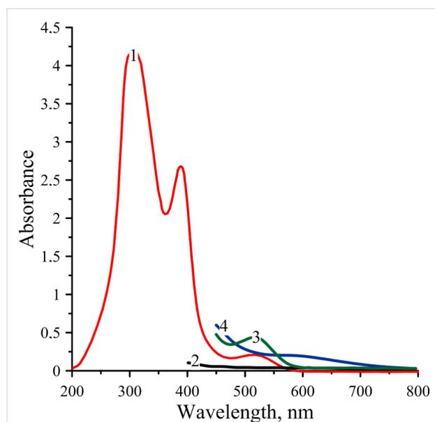
**Figure 1:** Absorption spectra in the UV and visible spectral region: 1) bis(cyclopentadienyl)titan dichloride (*n*-hexane, 0.4 mmol/L); 2) diethylaluminum chloride (*n*-hexane, 2.5 mmol/L); 3)  $\text{Cp}_2\text{TiCl}_2\cdot\text{AlEt}_2\text{Cl}$  (toluene, 10 mmol/L, Ti/Al ratios is 1:1, immediately after mixing); 4)  $\text{Cp}_2\text{TiCl}_2\cdot\text{AlEt}_2\text{Cl}$  (toluene, 10 mmol/L, Ti/Al ratios is 1:1, 10 minutes after mixing).
