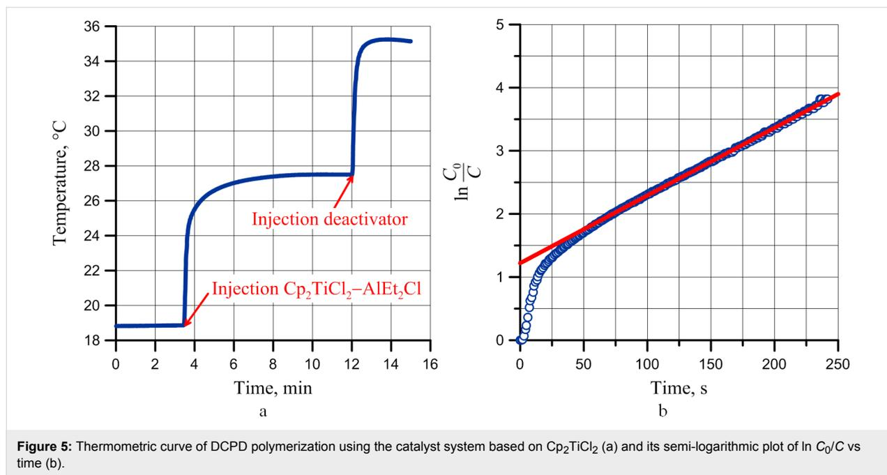
**Figure 5:** Thermometric curve of DCPD polymerization using the catalyst system based on  $\text{Cp}_2\text{TiCl}_2$  (a) and its semi-logarithmic plot of  $\ln C_0/C$  vs time (b).
