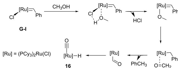
Scheme 4: Degradation pathway of first generation Grubbs catalyst (**G-I**) in methanol.Table 1: RCM of challenging substrate **17** in air and in the presence of water.
