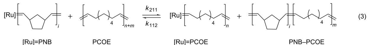
**Scheme 9:** Elementary reactions of MCM between PNB and PCOE, replotted from [90].
