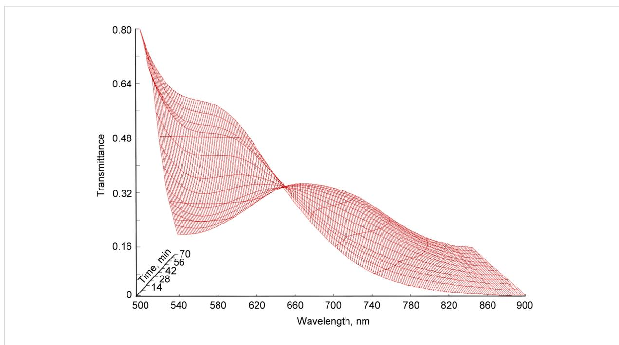
**Figure 4:** Visible spectra of a mixture of  $\text{Cp}_2\text{TiCl}_2$  and  $\text{AlEt}_2\text{Cl}$  as function of time.
