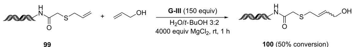
**Scheme 20:** On-DNA cross-metathesis reaction of allyl sulfide **99**.
