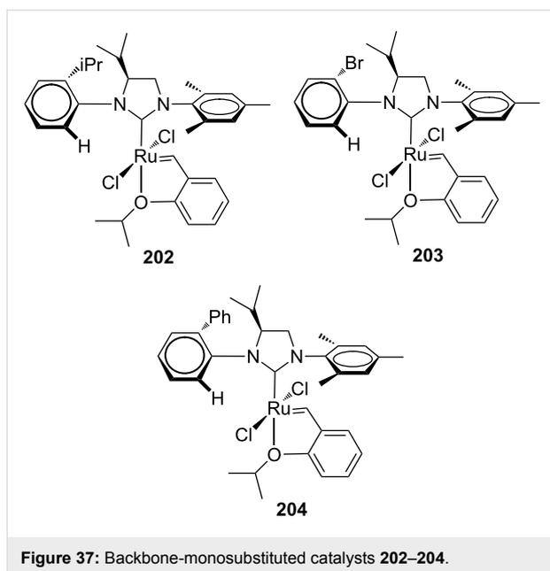
The catalysts **202–204** were tested in model ARCM and AROCM reactions. In the latter transformation, they were found to be highly efficient showing both excellent enantioselectivity and *E*-selectivity. In the AROCM of **75** with styrene (Scheme 8, reaction performed at  $-10$  °C using 5 equiv styrene and 1 mol % of the catalyst), complex **204** gave the desired product **76** in >98% conversion, 93% ee and *E/Z* ratio > 30:1.
