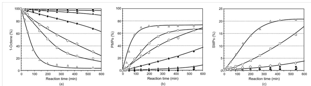
**Figure 6:** The influence of the reaction temperature on the (a) conversion of 1-octene, (b) formation of PMPs and (c) formation of SMPs using precatalyst 8 (Ru/1-octene = 1:9000). ◆ 40 °C, ■ 50 °C, ▲ 60 °C, ● 70 °C, ◇ 80 °C, □ 90 °C, △ 100 °C].
