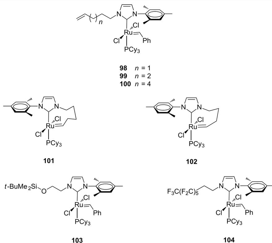
Figure 19: Grubbs-type complexes **98–104** with *N*-alkyl, *N'*-mesityl NHCs.
