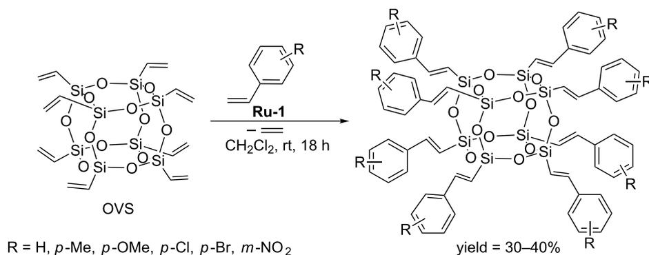
**Scheme 4:** Cross metathesis of OVS with substituted styrenes.
