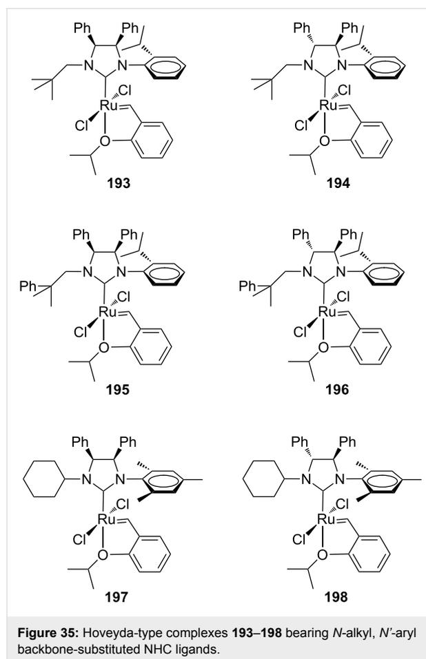
All the aforementioned catalysts with an *anti* NHC backbone configuration (**190**, **192**, **194**, **196** and **198**) were tested in model ARCM and AROCM reactions displaying moderate enantioselectivities [60,61]. In the ARCM of **166**, differently from the other *C*<sub>1</sub>-symmetric catalysts reported by Collins [52,54],
