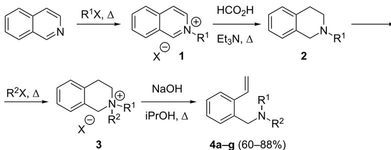
**Scheme 1:** Efficient multigram synthesis of *N,N*-dialkyl-2-vinylbenzylamines **4** (R<sup>1</sup>X = Me<sub>2</sub>SO<sub>4</sub>, Et<sub>2</sub>SO<sub>4</sub> or BnCl, see Experimental part, Supporting Information File 1 and Table 1).
