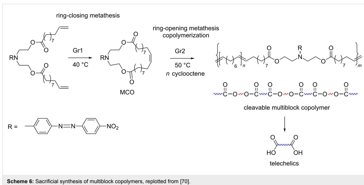
**Scheme 6:** Sacrificial synthesis of multiblock copolymers, replotted from [70].
