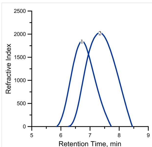
**Figure 8:** GPC traces for two samples of DCPD polymers obtained at a concentration of  $\text{Cp}_2\text{TiCl}_2/\text{AlEt}_2\text{Cl}$  complex 2 mmol/L (curve 1) and 10 mmol/L (curve 2).
