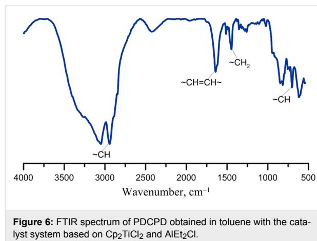
**Figure 6:** FTIR spectrum of PDCPD obtained in toluene with the catalyst system based on  $\text{Cp}_2\text{TiCl}_2$  and  $\text{AlEt}_2\text{Cl}$ .
