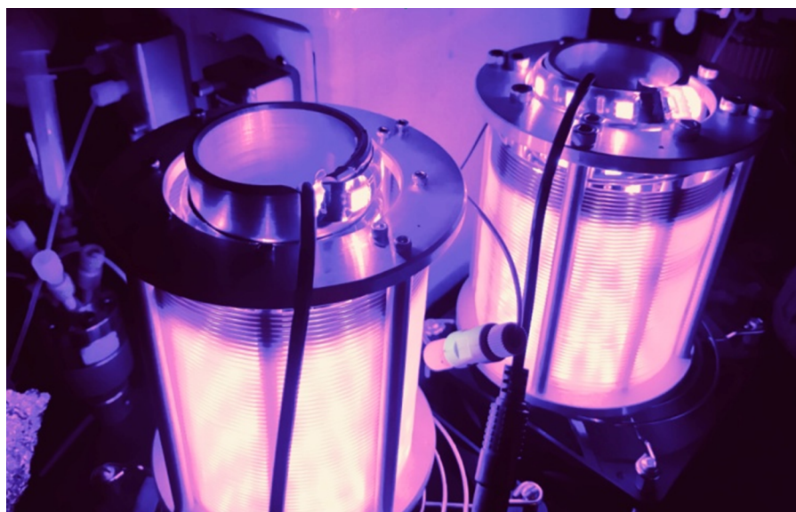
Figure 4: Experimental set-up for the photocatalytic conversion of alcohols to bromides. PFA tubing is wrapped around purple LEDs (394 nm) and fans are placed underneath reactors to maintain cooling.
