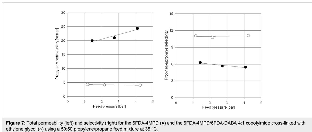
**Figure 7:** Total permeability (left) and selectivity (right) for the 6FDA-4MPD (●) and the 6FDA-4MPD/6FDA-DABA 4:1 copolyimide cross-linked with ethylene glycol (○) using a 50:50 propylene/propane feed mixture at 35 °C.
