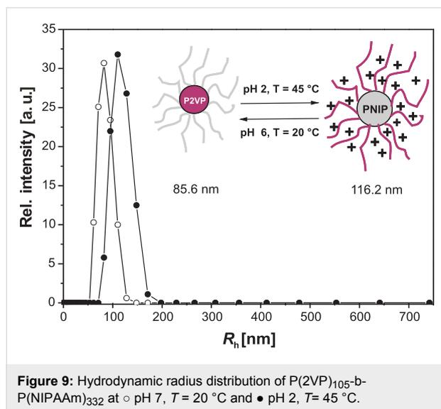
**Figure 9:** Hydrodynamic radius distribution of P(2VP)<sub>105</sub>-*b*-P(NIPAAm)<sub>332</sub> at ○ pH 7,  $T = 20$  °C and ● pH 2,  $T = 45$  °C.
