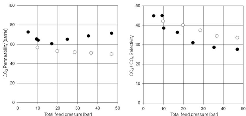
**Figure 15:** CO<sub>2</sub>/CH<sub>4</sub> separation characteristics for the 6FDA-4MPD/6FDA-DABA 4:1 copolyimide ionically cross-linked with aluminium acetylacetonate (●) and covalently cross-linked with ethylene glycol (○) at 35 °C using a 50:50 CO<sub>2</sub>/CH<sub>4</sub> feed gas mixture.
