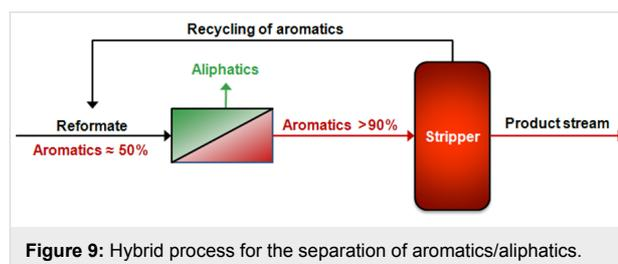
**Figure 9:** Hybrid process for the separation of aromatics/aliphatics.
