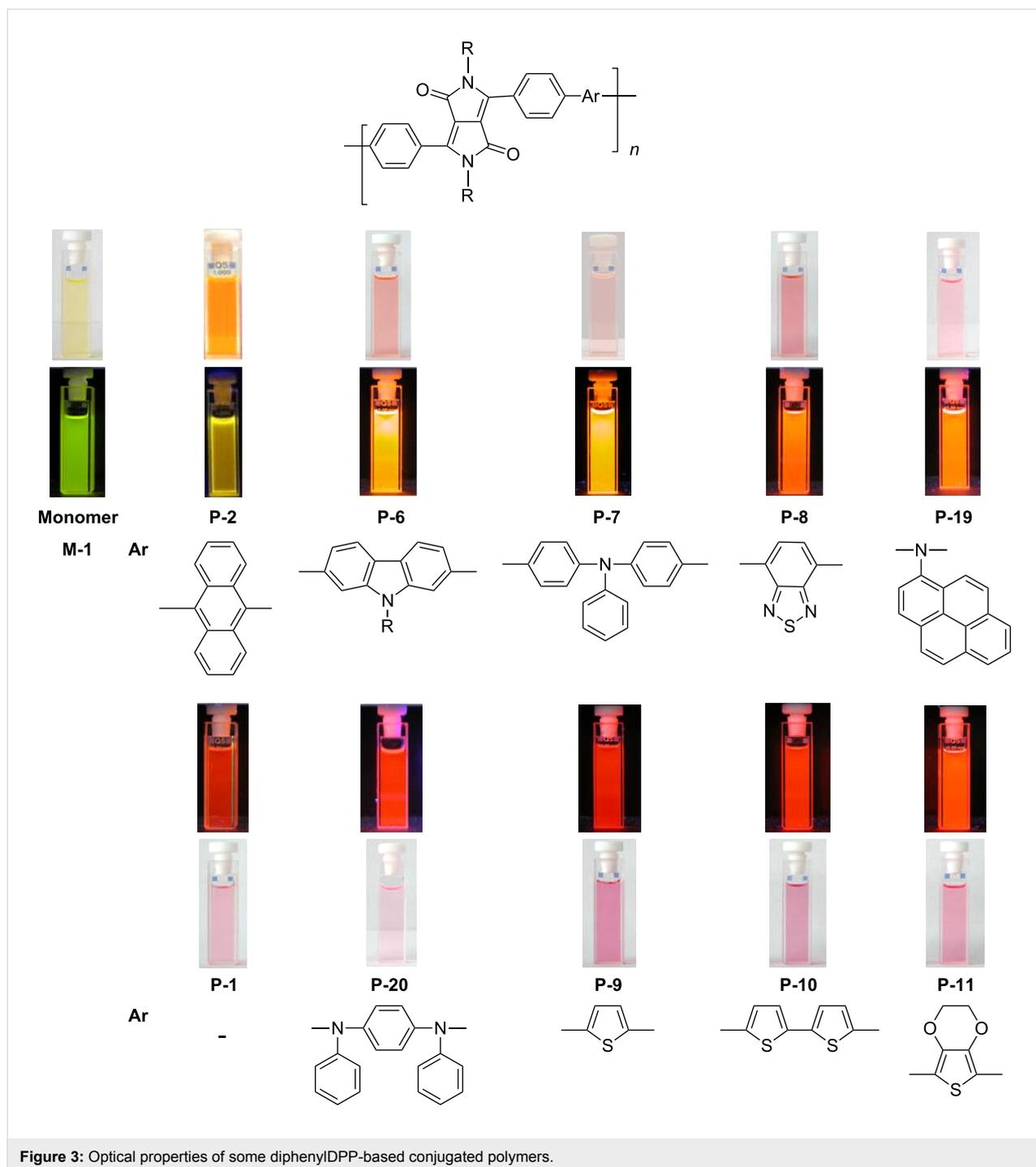
secondary arylamines to yield DPP-containing polyiminoarylenes. The solutions of the polymers in chloroform exhibited a purple red colour with absorption maxima between 530 and 550 nm, and emission maxima from 610 to 630 nm. Fluorescence quantum yields were moderate (20 to 60%) (see also Table 3). The nitrogen atoms in the backbone lower the band gap of the polymers to approximately 1.9 eV. The band gaps are lower than for the conjugated DPP-arene copolymers prepared
