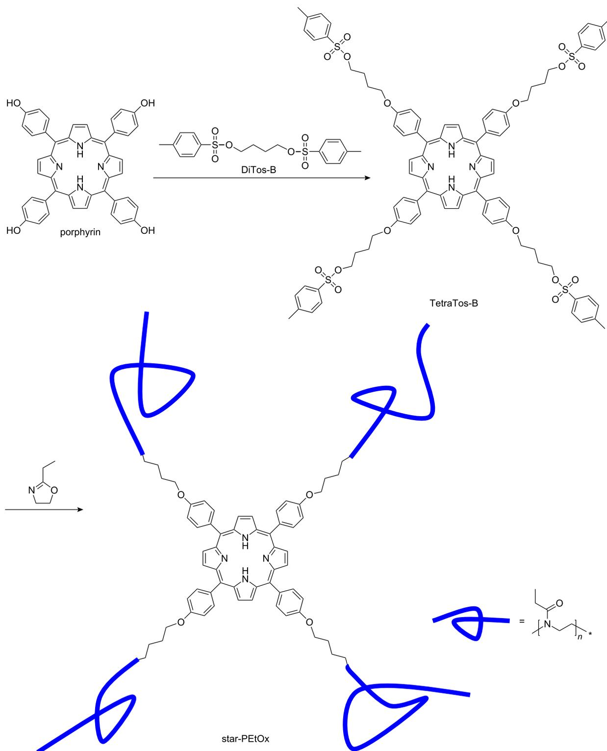
**Scheme 2:** Schematic representation of the synthesis of a porphyrin initiated four-armed star-pEtOx starting from *tetrakis*(hydroxyphenyl)porphyrin (**porphyrin**).
