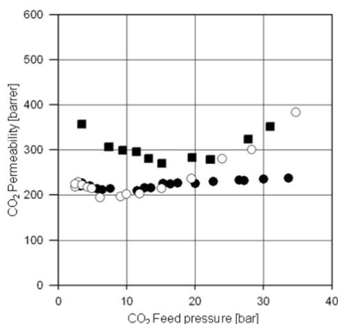
**Figure 14:** Pure CO<sub>2</sub> permeabilities at 35 °C for the 6FDA-4MPD (■), the 6FDA-4MPD/6FDA-DABA 4:1 copolyimide ionically cross-linked with aluminium acetylacetonate (○) and covalently cross-linked with ethylene glycol (●).
