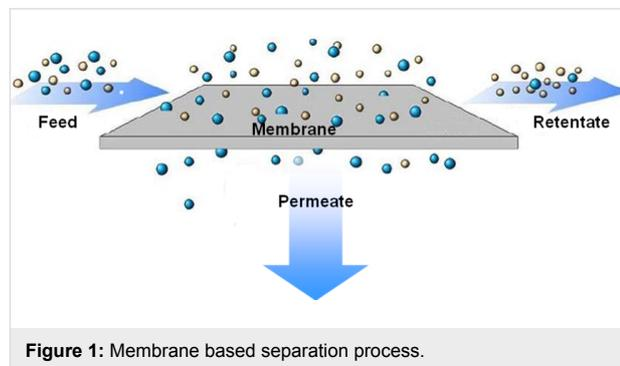
Figure 1: Membrane based separation process.
