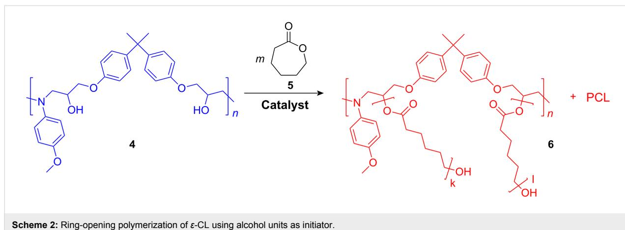
The dilution of the hydroxy groups in the obtained product **6** was proven by IR spectroscopy by the nearly complete disappearance of the OH-related absorption band at  $3370\text{ cm}^{-1}$ . Furthermore, the formation of ester units was confirmed by the appearance of two strong bands at  $1721$  and  $1176\text{ cm}^{-1}$  associated with C=O and C-O stretching vibrations, respectively.
