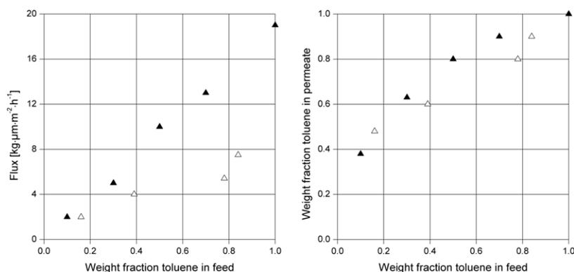
**Figure 11:** Pervaporation results for 6FDA-4MPD/6FDA-DABA 4:1 copolyimide (non cross-linked) conditioned in pure toluene (▲) and in a mixture of 90:10 toluene/cyclohexane (Δ). After conditioning, the measurements were performed using toluene/cyclohexane mixtures at 60 °C and a permeate pressure of 20–25 mbar.
