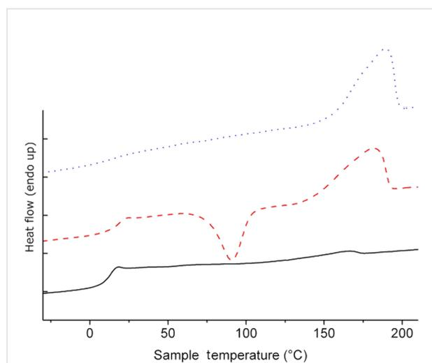
**Figure 6:** DSC heating traces (second heating run at 20 °C/min) for *hb*- $\text{PG}_{38}$ -*b*- $\text{GA}_4$  (bottom), *hb*- $\text{PG}_{38}$ -*b*- $\text{GA}_8$  (middle) and *hb*- $\text{PG}_{38}$ -*b*- $\text{GA}_{12}$  (top), reflecting the increasing influence of polyglycolide chain length.
