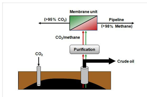
**Figure 13:** Hybrid process for the removal of CO<sub>2</sub> in tertiary oil production processes.
