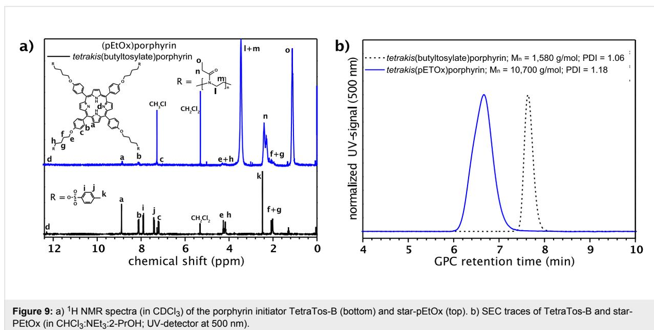
**Figure 9:** a)  $^1\text{H}$  NMR spectra (in  $\text{CDCl}_3$ ) of the porphyrin initiator TetraTos-B (bottom) and star-pETox (top). b) SEC traces of TetraTos-B and star-PETox (in  $\text{CHCl}_3\text{:NEt}_3\text{:2-PrOH}$ ; UV-detector at 500 nm).
