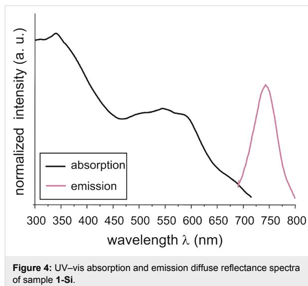
**Figure 4:** UV-vis absorption and emission diffuse reflectance spectra of sample **1-Si**.
