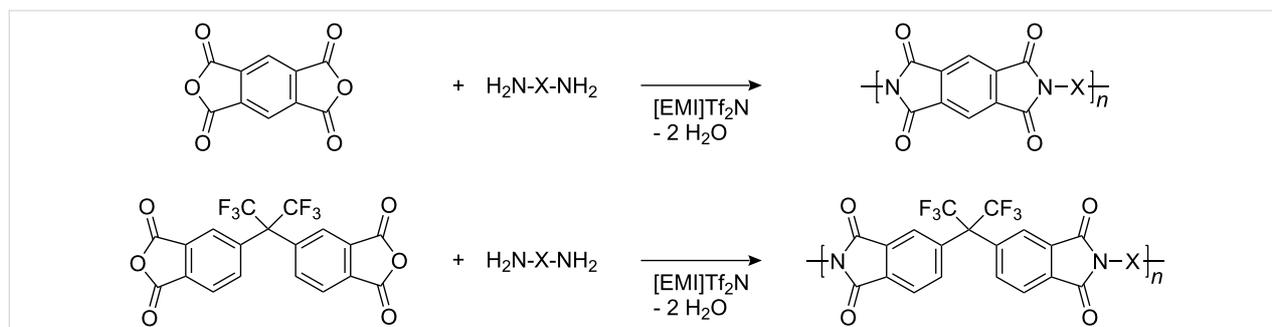
**Scheme 2:** Polyimide from the reaction performed in the ionic liquid 1-ethyl-3-methylimidazolium bis(trifluoromethylsulfonyl)imide  $[\text{EMI}]\text{Tf}_2\text{N}$  between a diamine  $\text{H}_2\text{N-X-NH}_2$  and pyromellitic acid dianhydride, and 4,4'-(hexafluoroisopropylidene)diphthalic anhydride (from [15]).
