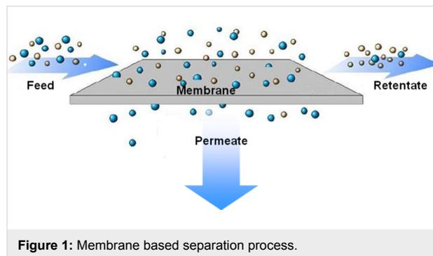
Figure 1: Membrane based separation process.
