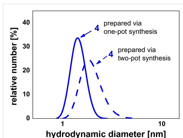
**Figure 4:** Number-average hydrodynamic diameters of compound **4** prepared via the one-pot (continuous line) and the two-pot (dashed line) synthesis.
