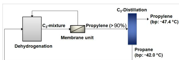
**Figure 6:** Hybrid process for the separation of propylene/propane.
