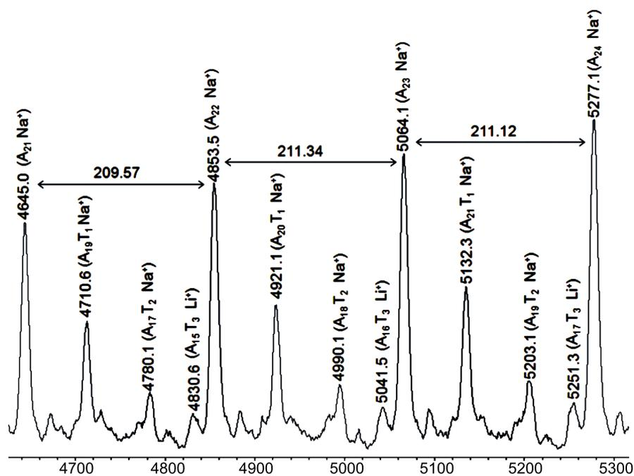
Figure 10: MALDI-TOF mass spectrum of BCP-A<sub>25</sub>T<sub>2</sub> 13 synthesized with catalyst U3.
