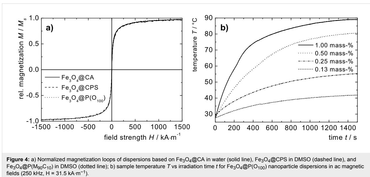
**Figure 4:** a) Normalized magnetization loops of dispersions based on  $\text{Fe}_3\text{O}_4@CA$  in water (solid line),  $\text{Fe}_3\text{O}_4@CPS$  in DMSO (dashed line), and  $\text{Fe}_3\text{O}_4@P(\text{M}_{90}\text{C}_{10})$  in DMSO (dotted line); b) sample temperature  $T$  vs irradiation time  $t$  for  $\text{Fe}_3\text{O}_4@P(\text{O}_{100})$  nanoparticle dispersions in ac magnetic fields (250 kHz,  $H = 31.5 \text{ kA}\cdot\text{m}^{-1}$ ).
