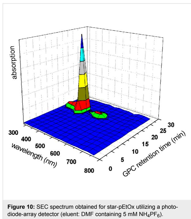
**Figure 10:** SEC spectrum obtained for star-pEtOx utilizing a photodiode-array detector (eluent: DMF containing 5 mM  $\text{NH}_4\text{PF}_6$ ).
