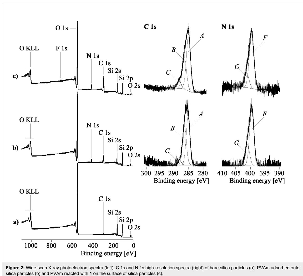
**Figure 2:** Wide-scan X-ray photoelectron spectra (left), C 1s and N 1s high-resolution spectra (right) of bare silica particles (a), PVAm adsorbed onto silica particles (b) and PVAm reacted with **1** on the surface of silica particles (c).
