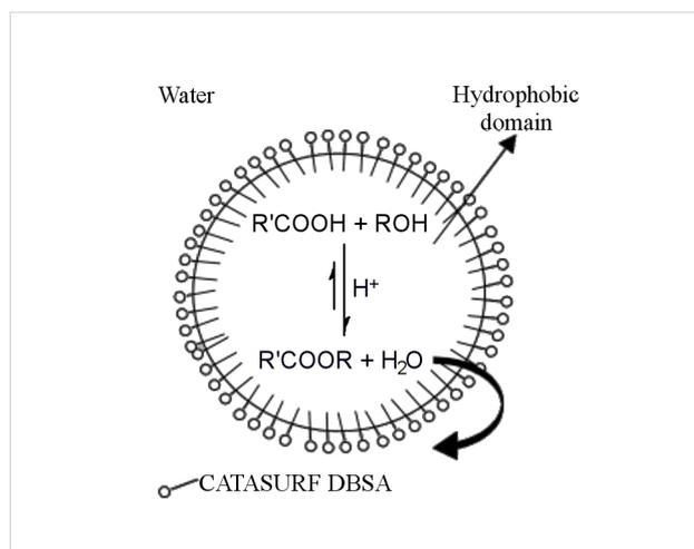
**Figure 8:** Schematics for the polycondensation reaction between hydrophobic alcohols and carboxylic acids surrounded by the aqueous continuous phase (not to scale for the surfactant) (reprinted with permission from [13]. Copyright (2003) Elsevier).
