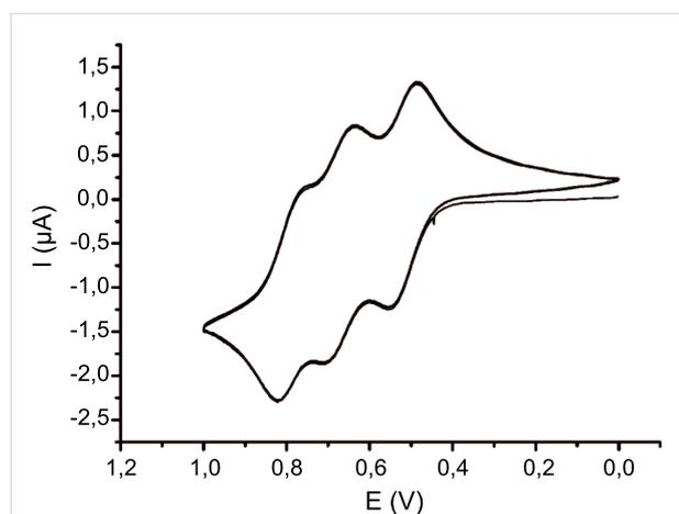
**Figure 2:** Cyclic voltammogram of thioacetate **2d** (recorded in  $\text{CH}_2\text{Cl}_2$ ,  $T = 293$  K; 0.1 M electrolyte  $[\text{Bu}_4\text{N}][\text{PF}_6]$ ;  $\nu = 100$  mV/s; Pt-working electrode, Ag/AgCl-reference and Pt-counter electrode).
