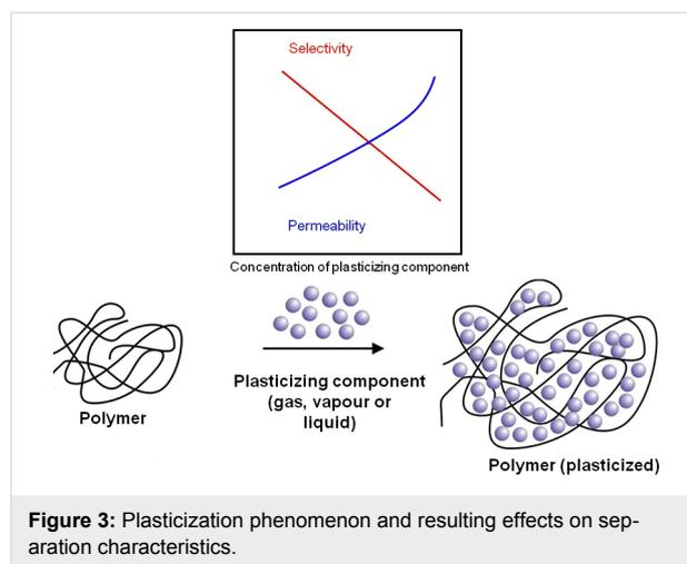
**Figure 3:** Plasticization phenomenon and resulting effects on separation characteristics.
