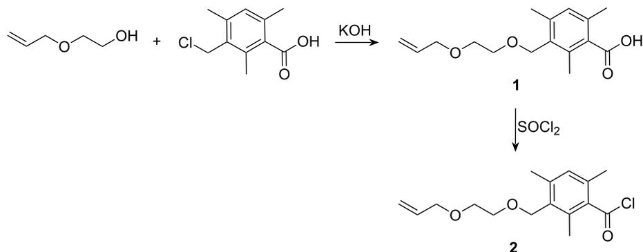
**Scheme 2:** Etherification of 3-(chloromethyl)-2,4,6-trimethylbenzoic acid and chlorination of **1**.
