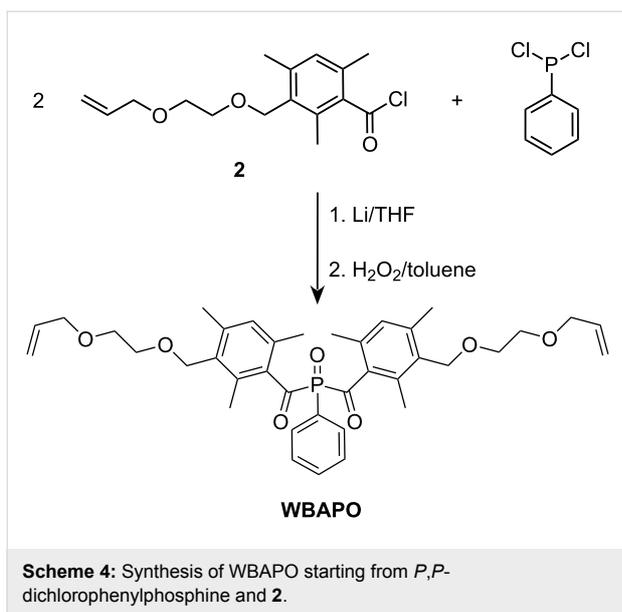
tions during the lithiation step. Furthermore, it was found that the temperature of the phosphine oxidation significantly influenced the yield and the purity of the formed phosphine oxide as
