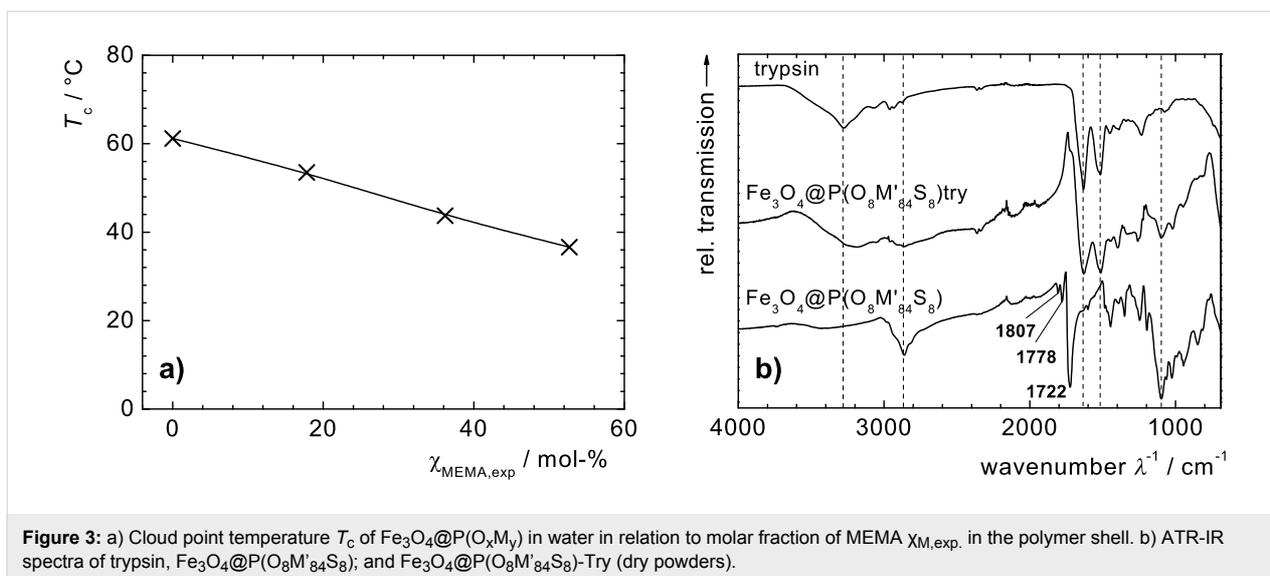
**Figure 3:** a) Cloud point temperature  $T_c$  of  $\text{Fe}_3\text{O}_4@P(\text{O}_x\text{M}_y)$  in water in relation to molar fraction of MEMA  $\chi_{\text{MEMA,exp}}$  in the polymer shell. b) ATR-IR spectra of trypsin,  $\text{Fe}_3\text{O}_4@P(\text{O}_8\text{M}'_{84}\text{S}_8)$ ; and  $\text{Fe}_3\text{O}_4@P(\text{O}_8\text{M}'_{84}\text{S}_8)\text{-Try}$  (dry powders).
