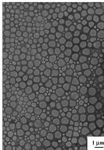
**Figure 7:** Transmission electron micrograph of polyurethane capsules synthesized by interfacial polyaddition in inverse miniemulsion (reprinted with permission from [116]. Copyright (2007) American Chemical Society).
