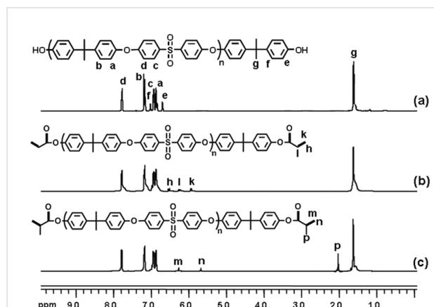
**Figure 2:** <sup>1</sup>H NMR spectra of PSU-2000 (a), PSU-DA-2000 (b) and PSU-DM-2000 (c) in CDCl<sub>3</sub>.
