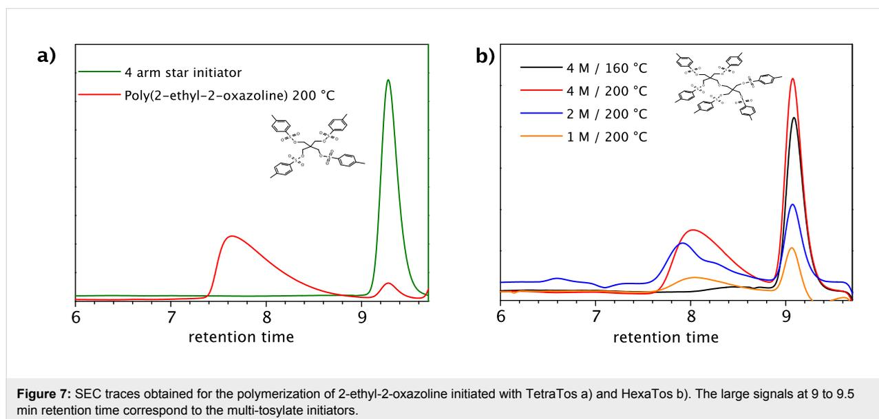
**Figure 7:** SEC traces obtained for the polymerization of 2-ethyl-2-oxazoline initiated with TetraTos a) and HexaTos b). The large signals at 9 to 9.5 min retention time correspond to the multi-tosylate initiators.
