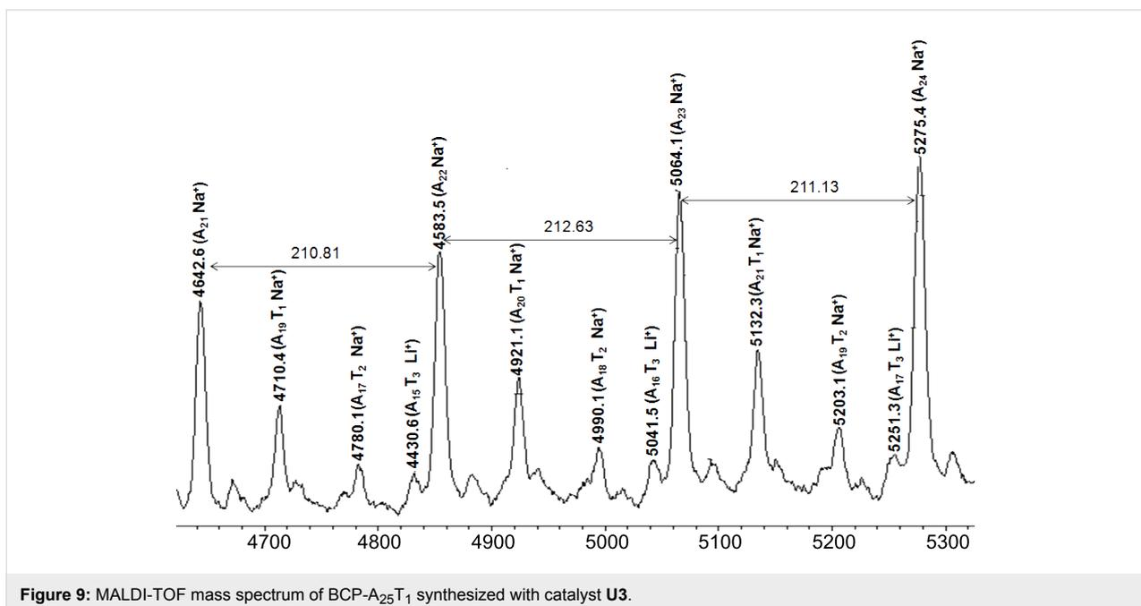
Figure 9: MALDI-TOF mass spectrum of BCP- $A_{25}T_1$  synthesized with catalyst **U3**.
