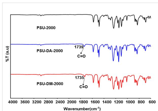
**Figure 1:** FT-IR spectra of PSU-2000, PSU-DA-2000 and PSU-DM-2000.
