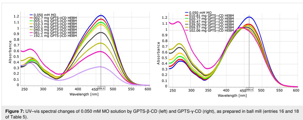
**Figure 7:** UV-vis spectral changes of 0.050 mM MO solution by GPTS- $\beta$ -CD (left) and GPTS- $\gamma$ -CD (right), as prepared in ball mill (entries 16 and 18 of Table 5).
