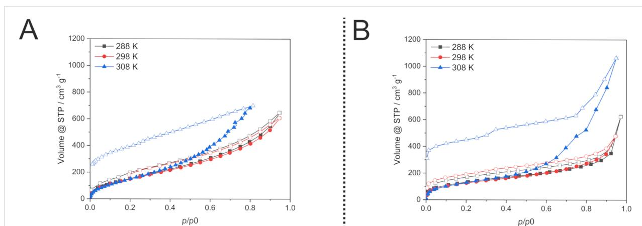
**Figure 5:** Physisorption isotherms of benzene vapour at different temperatures on HCP synthesised classically from solution (left, A) and mechanochemically (right, B). Filled symbols denote adsorption and open symbols desorption, respectively.
