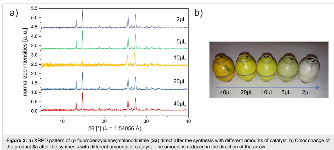
**Figure 2:** a) XRPD pattern of (*p*-fluorobenzylidene)malonodinitrile (**3a**) direct after the synthesis with different amounts of catalyst. b) Color change of the product **3a** after the synthesis with different amounts of catalyst. The amount is reduced in the direction of the arrow.
