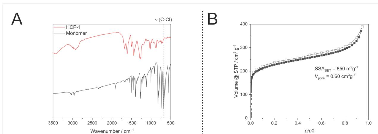
**Figure 2:** A: IR spectra of the monomer BCMBP and NG-HCP showing a decrease of the C–Cl vibration after the reaction. B: Low pressure nitrogen isotherm of NG-HCP demonstrating the textural properties.
