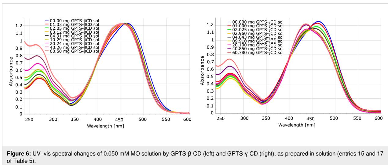
**Figure 6:** UV-vis spectral changes of 0.050 mM MO solution by GPTS- $\beta$ -CD (left) and GPTS- $\gamma$ -CD (right), as prepared in solution (entries 15 and 17 of Table 5).
