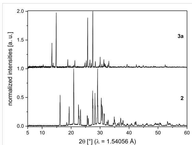
**Figure 1:** Comparison of XRPD pattern of malonodinitrile (**2**) and (*p*-fluorobenzylidene) malonodinitrile (**3a**). The patterns are baseline corrected.
