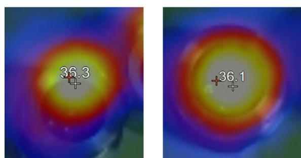
**Figure 1:** IR thermometer images showing reactor temperatures at the end of the two individual ball-milling reactions (averaged results collected in Table 1, entry 11; individual results, see Supporting Information File 1, left: Table S1, entry 11-1, right: Table S1, entry 11-2).
