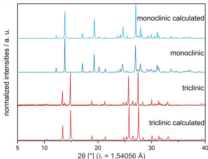
**Figure 5:** Comparison of XRPD patterns of both polymorphs of the product **3a**. Red: triclinic polymorph **t3a**. Blue: monoclinic polymorph **m3a**. The light XRPD pattern were calculated from single crystal diffraction data.
