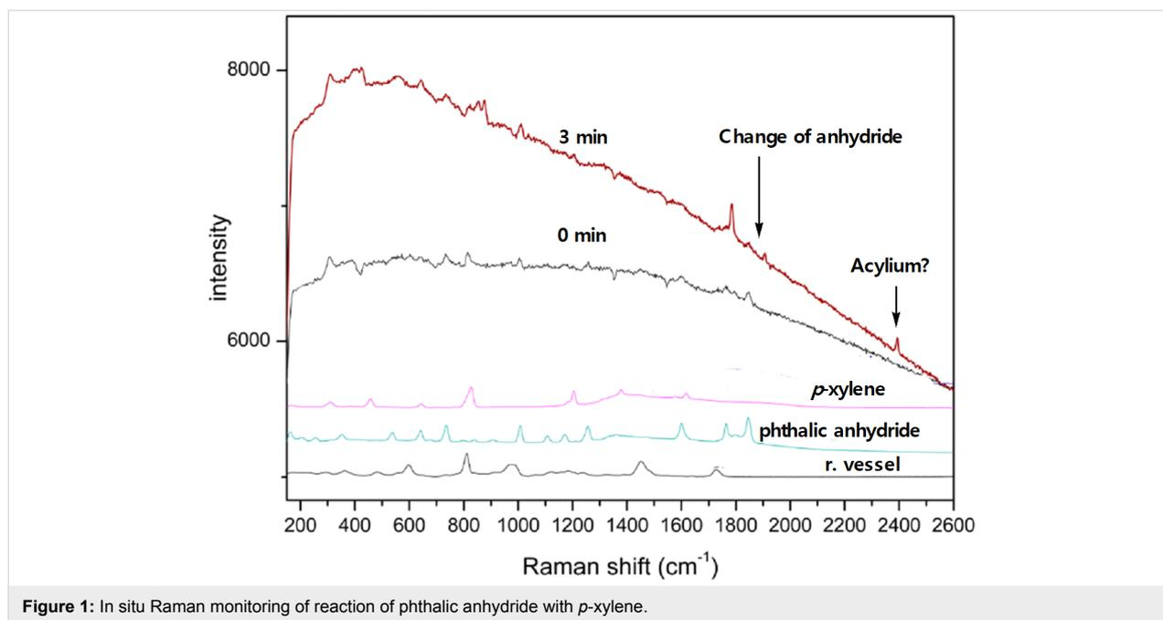
**Figure 1:** In situ Raman monitoring of reaction of phthalic anhydride with *p*-xylene.
