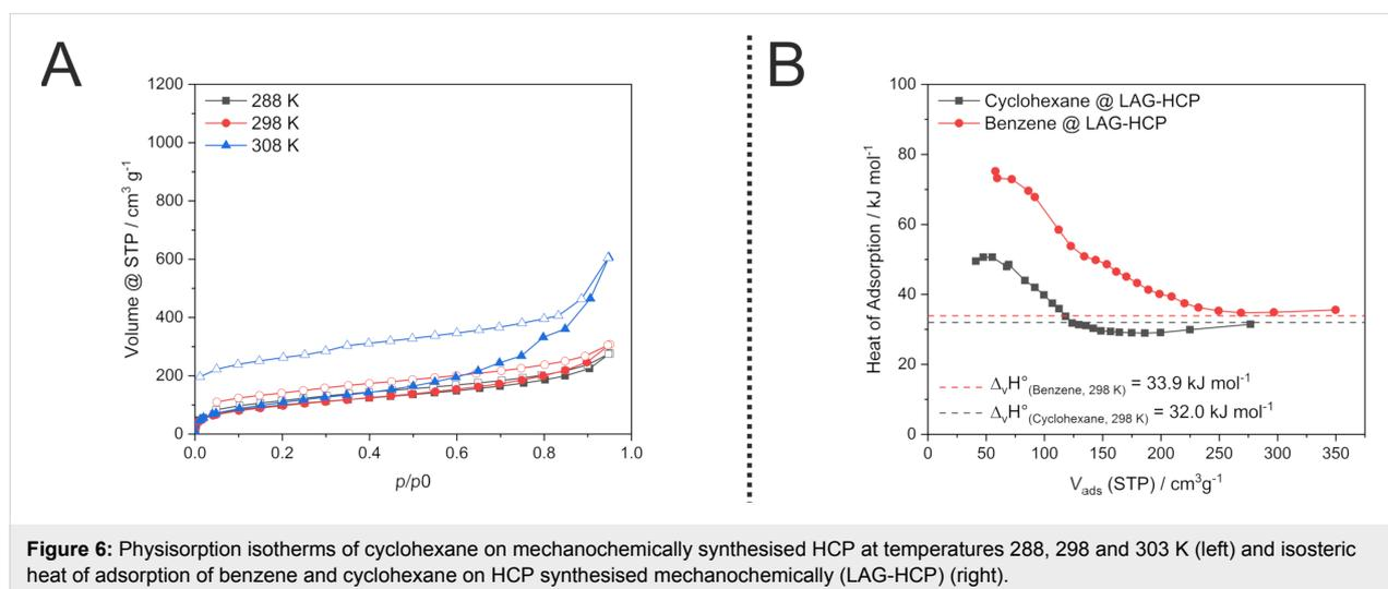
**Figure 6:** Physisorption isotherms of cyclohexane on mechanochemically synthesised HCP at temperatures 288, 298 and 303 K (left) and isosteric heat of adsorption of benzene and cyclohexane on HCP synthesised mechanochemically (LAG-HCP) (right).
