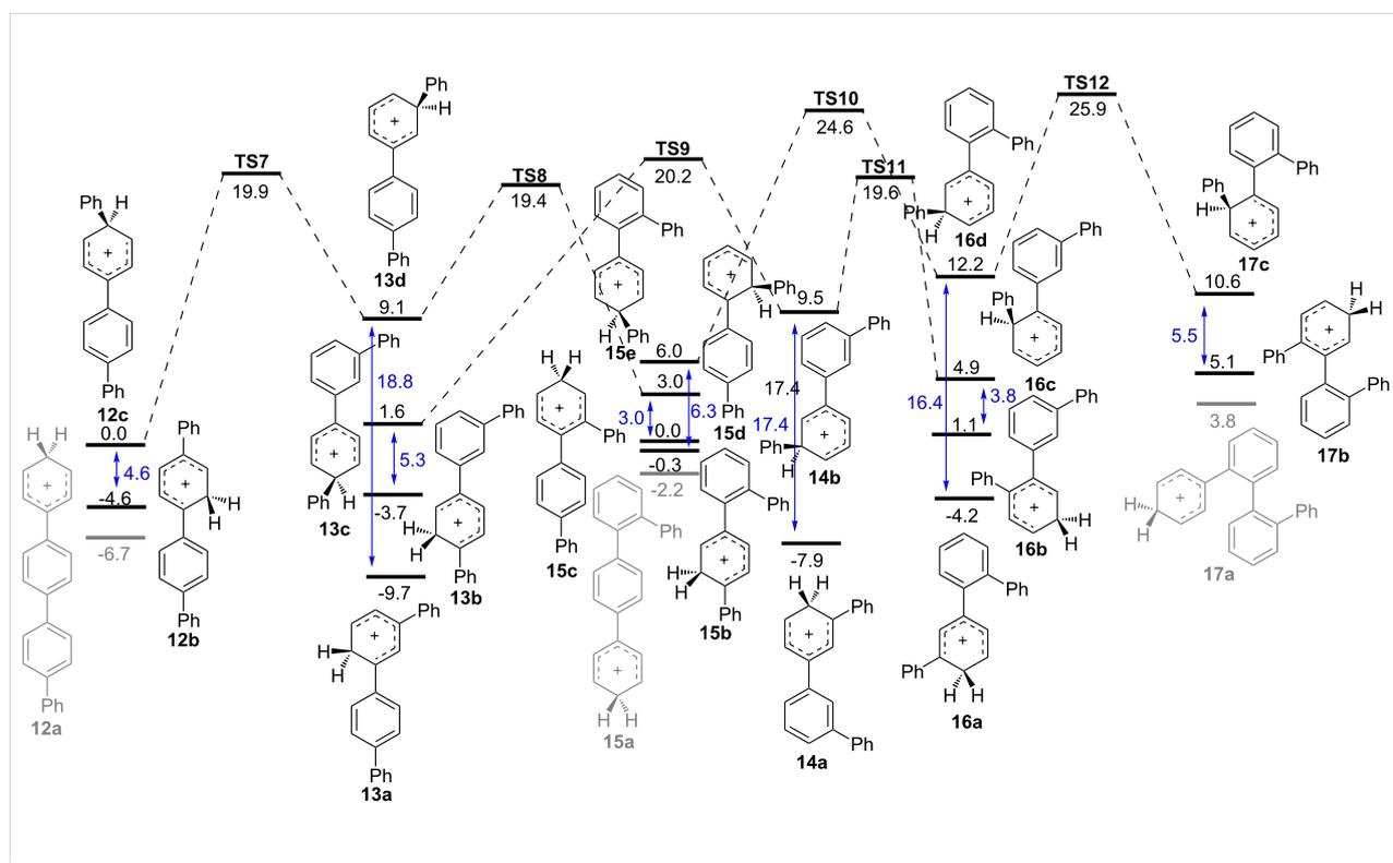
**Figure 1:** Pathways for terminal 1,2-phenyl shifts in quaterphenyl isomers calculated with IEFPCM(DCE)/B3LYP/6-31+G(d,p) theory. Relative free energies are given in kcal/mol.
