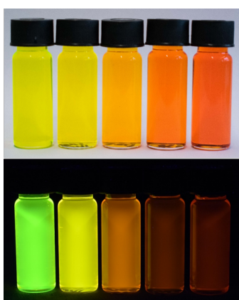
Figure 11: Absorption (top) and fluorescence (bottom) of compound 6c with variable solvent polarity (left to the right: toluene, ethyl acetate, acetone, DMF and DMSO, c(\mathbf{6c}) = 10^{-4} M; \lambda_{\text{exc}} = 365 nm, handheld UV lamp).
