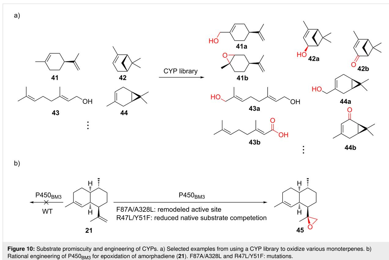
**Figure 10:** Substrate promiscuity and engineering of CYPs. a) Selected examples from using a CYP library to oxidize various monoterpenes. b) Rational engineering of P450<sub>BM3</sub> for epoxidation of amorphaadiene (**21**). F87A/A328L and R47L/Y51F: mutations.
