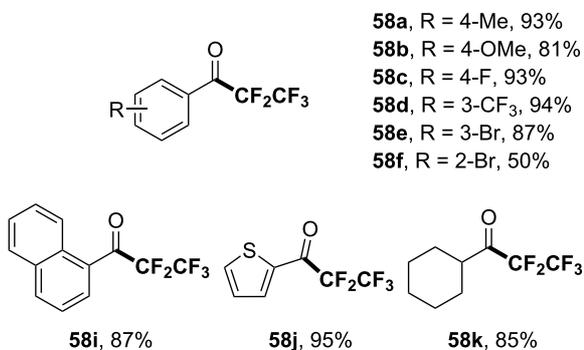
**Scheme 16:** Synthesis of pentafluoroethyl ketones using the  $(\text{Ph}_3\text{P})\text{Cu}(\text{phen})\text{CF}_2\text{CF}_3$  reagent.  $^{19}\text{F}$  NMR yields were given using 1,3-bis(trifluoromethyl)benzene as the internal standard.
