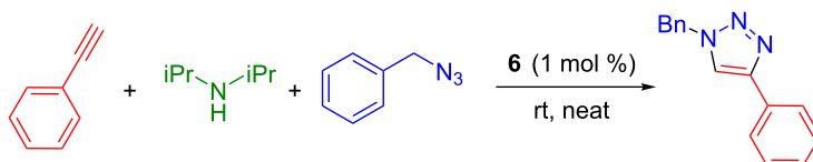
Scheme 6: Reactivity of "non-sulfonyl" azide [33]. Reaction conditions: phenylacetylene (0.5 mmol), benzyl azide (0.6 mmol), diisopropylamine (0.6 mmol), 24 h.
