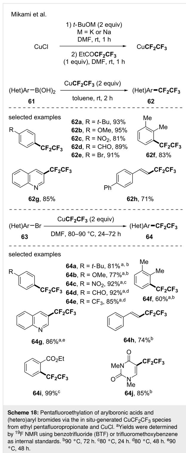
More recently, in the course of their investigation to generate a CuCF<sub>3</sub> reagent from a cyclic-protected hexafluoroacetone, an air-stable liquid trifluoromethylating reagent, and KCu(O*t*-Bu)<sub>2</sub>, the group of Mikami showed that a CF<sub>2</sub>CF<sub>3</sub> analog (Scheme 19) was prepared in a similar way and applied for the pentafluoroethylation of aromatic derivatives [74] (2 examples).
