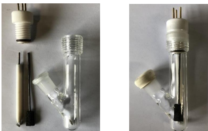
Figure S1. Components of the reaction setup (left) and assembled reaction vessel (right).
