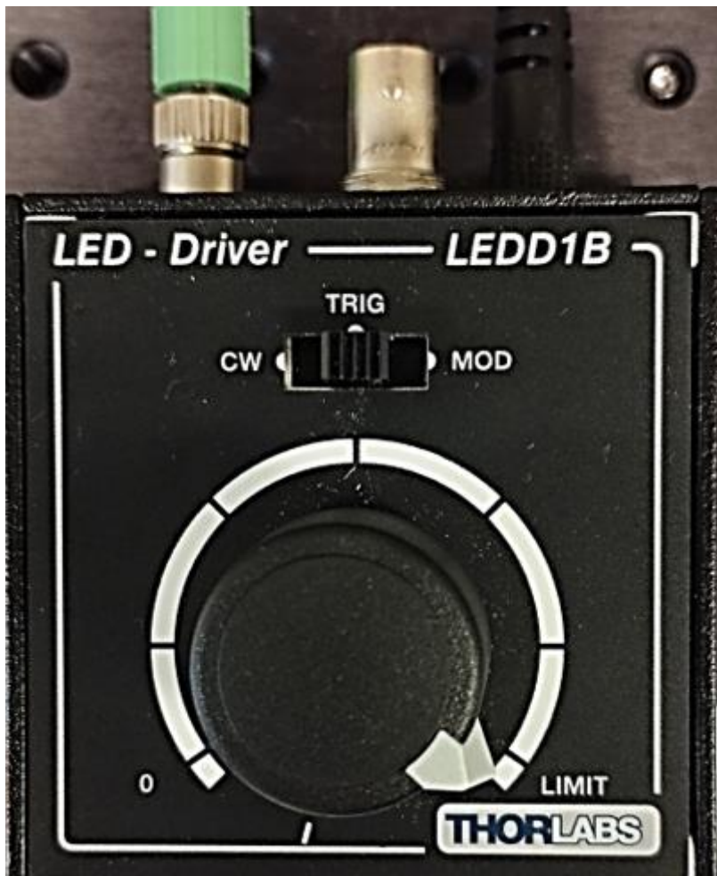
Figure S2: Picture of the LED driver in TRIG mode.
