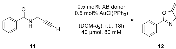
Scheme 2: Schematic representation of the activation of propargylic amide 11 with a catalyst system loading of 0.5 mol %.
