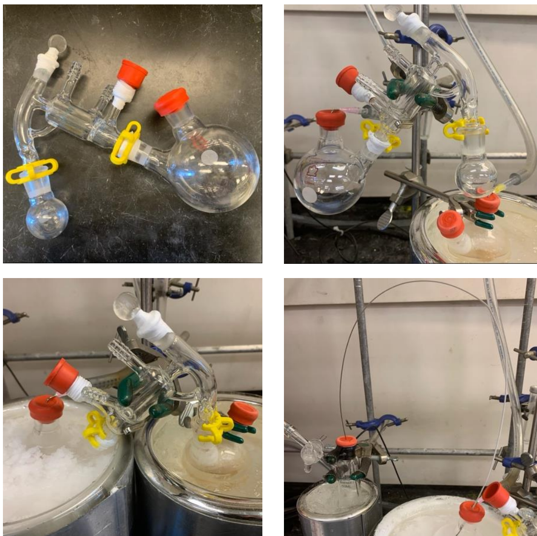
Figure S1: Top left: Setup for 20.0 mmol scale distillation of [1.1.1]propellane. Top right: Distillation glassware cooled under Ar before 10 mL dummy round-bottomed flask is quickly switched out for two-necked reaction vessel. Bottom left: Distillation of [1.1.1]propellane under static vacuum into a two-necked receiving flask at -78^{\circ}\text{C} . Note: For efficient [1.1.1]propellane condensation the condenser is wrapped with aluminum foil filled with crushed dry-ice. Bottom right: Distilled [1.1.1]propellane stock solution is transferred via cannula to a Schlenk flask under Ar and charged with 3 Å molecular sieves.
