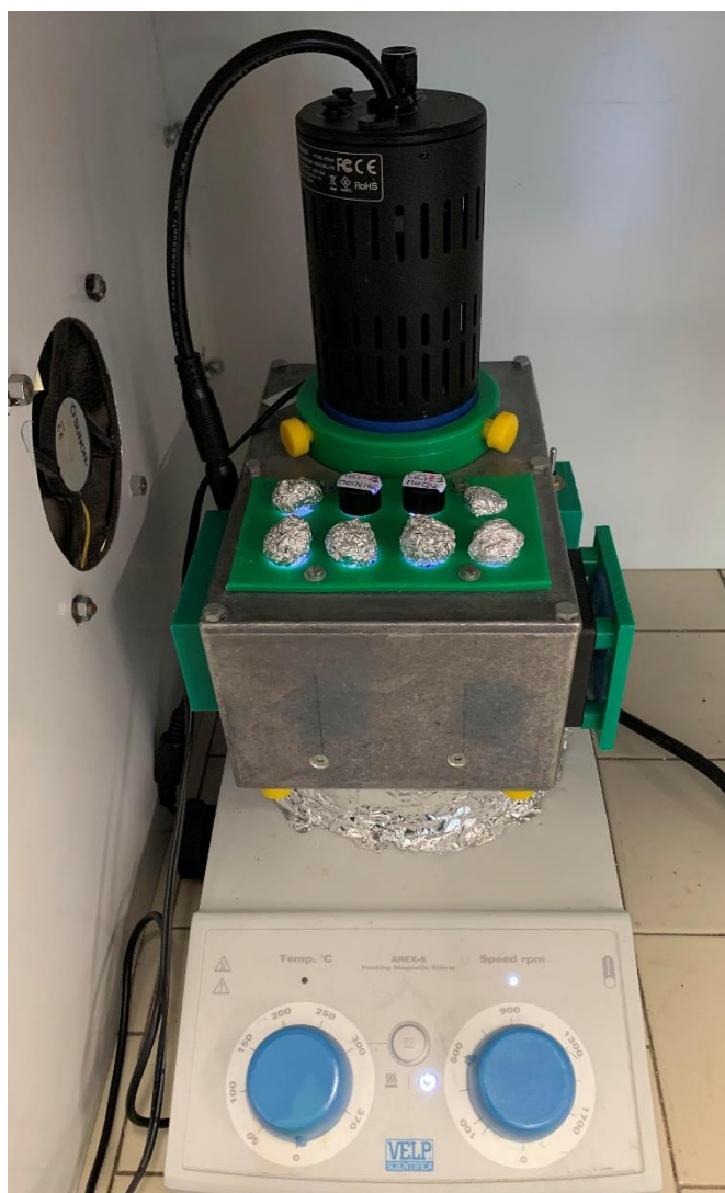
Figure S3: Glass vessel containing the reaction mixture, equipped with a magnetic stirrer and closed with a screw cap in a homemade photoreactor equipped with a lateral fan, on a magnetic plate and irradiated with a 40 W Kessil lamp (full power; emission centered at 427 nm).
