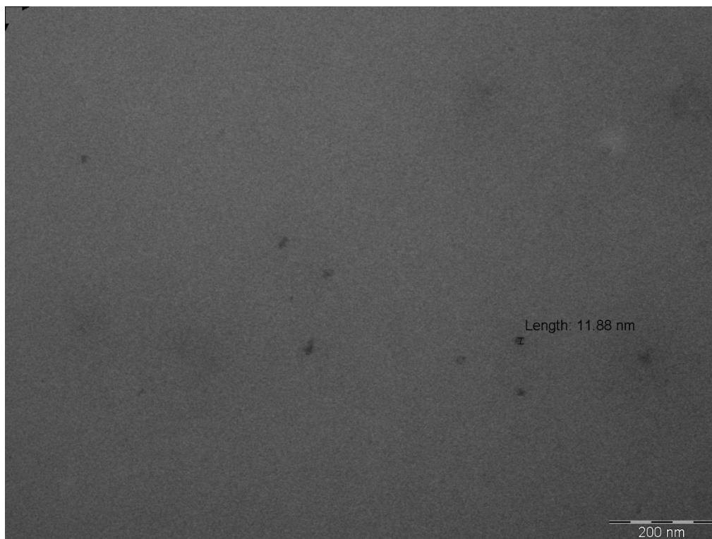
Figure S2: TEM image of carbon dots obtained from blackberries residue (CD-a-N-BB).
