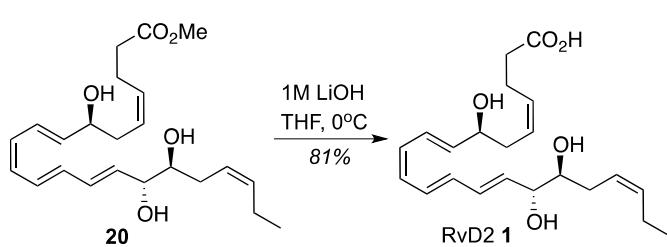
To a solution of the RvD2 methyl ester (**20**) (9.6 mg, 24.6  $\mu$ mol) in THF (0.5 mL) at 0 °C was added LiOH (1 M, 120  $\mu$ L, 120  $\mu$ mol). The solution was stirred at
