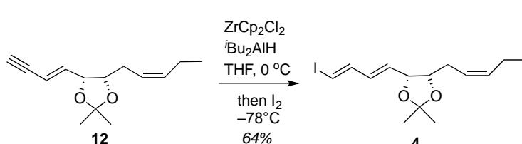
To a suspension of ZrCp<sub>2</sub>Cl<sub>2</sub> (262.5 mg, 0.898 mmol) in THF (3.2 mL) at 0 °C was added a solution of iBu<sub>2</sub>AlH in THF (1M, 0.89 mL, 0.898 mmol).
