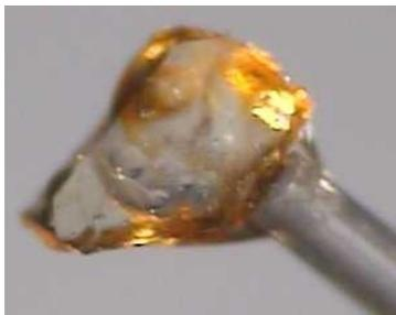
**Figure S1.** Specimen employed in the X-ray experiment. Real dimensions:  $0.500 \times 0.350 \times 0.175$  mm
