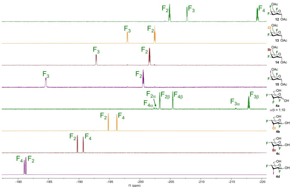
Figure S1. Direct comparison of ^{19}\text{F} resonances of halogenated talose analogues 12–15 ( ^{19}\text{F} NMR; 470 MHz, \text{CDCl}_3 ) and halogenated allose analogues 4a–d ( ^{19}\text{F} NMR; 470 MHz, acetone- d 6 ).
