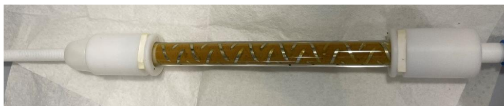
Figure 6. Photos of the packed column with a helical static mixer (polished SS316, 10 cm length, 15 mixing elements L/D= 1.04 from Stamixco AG).
